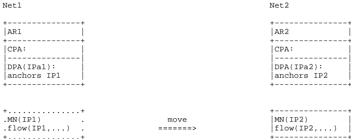
Figure 3. Changing to the new IP prefix/address. MN running a flow using IP1 in Net1 changes to running a flow using IP2 in Net2.
