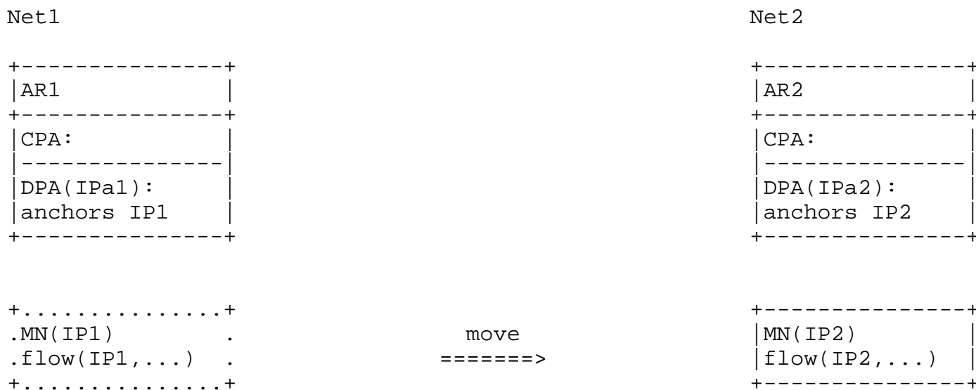
Figure 4. Changing to the new IP prefix/address. MN running a flow using IP1 in a network Net1 changes to running a flow using IP2 in Net2.
