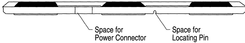
Figure 1-5. Back Edge of Air Flow Module
