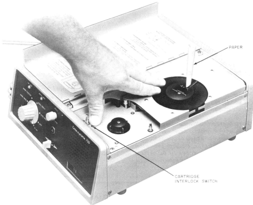
Fig. 7—Resetting “0” Registration on Message Indicator Dial
