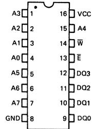
A – Address Input       $\bar{W}$  – Write Enable
