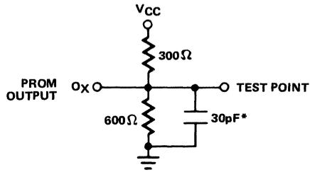
\* Includes jig & probe total capacitance
