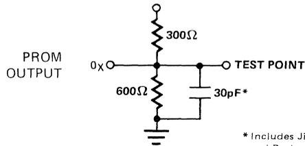
\* Includes Jig and Probe Total Capacitance
