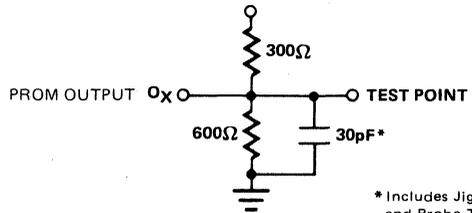
\* Includes Jig and Probe Total Capacitance
