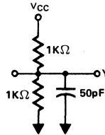
OUTPUT TEST CIRCUIT
