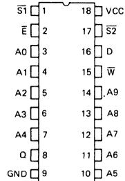
A - ADDRESS INPUT      W - WRITE ENABLE
