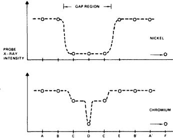
NOTE: (A) "FROZEN SPLASH" EFFECT PROGRAMMING HAS MELTED NiCr IN GAP REGION.
