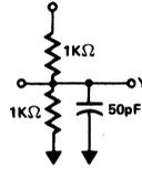
OUTPUT TEST CIRCUIT
