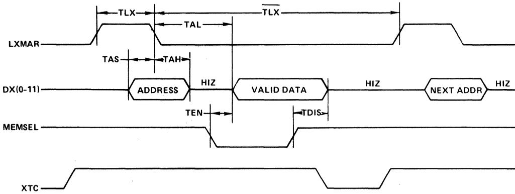
FIGURE 1-1 — Read Cycle Timing
