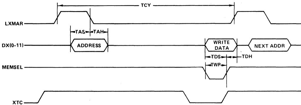
FIGURE 1-2 — Write Cycle Timing
