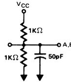
**OUTPUT TEST CIRCUIT
