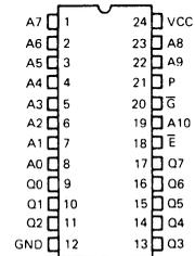
A Address Input                       $\bar{G}$  Output Enable
