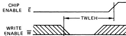
The example shows Write pulse setup time defined as TWLEH—Time from Write enable Low to chip Enable High.
