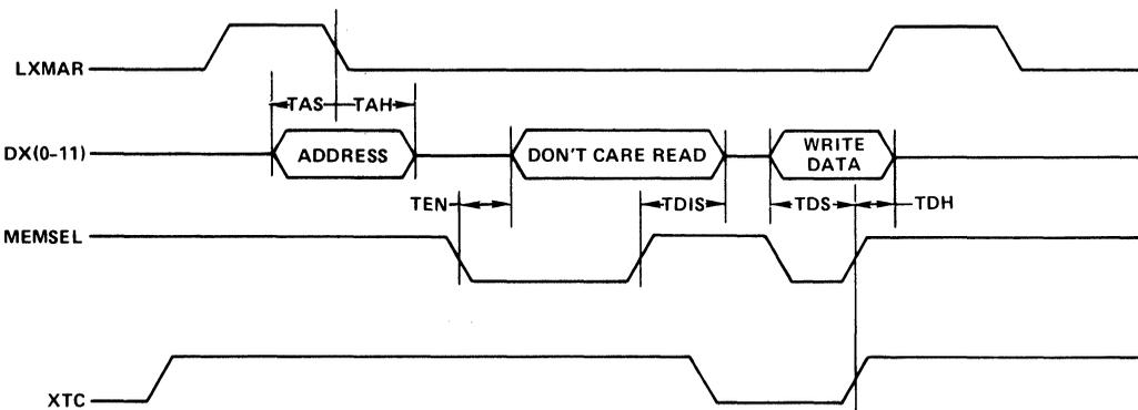
FIGURE 1-3 — MICRO-12 Compatible Timing Read Modify Write Cycle
