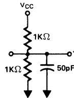
OUTPUT TEST CIRCUIT
