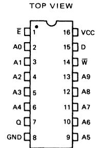
A – Address Input      D – Data Input
