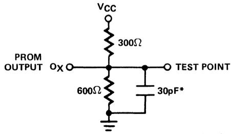
\* Includes jig & probe total capacitance
