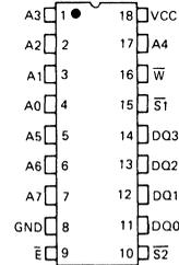
A – Address Input       $\bar{W}$  – Write Enable
