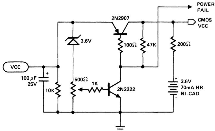
FIGURE 3 – A Typical Battery Back-Up Circuit
