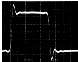
Small-Signal Transient ( A_V = 1 )
