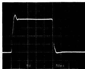
Large-Signal Transient (AV = -1)
