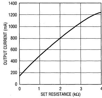
Figure 15. LTC1142-ADJ Output Current vs Trickle Charge Set Resistance ( R_X ) for the Circuit in Figure 14 Using a 0.1Ω Current Sense Resistor R_{SENSE1}
