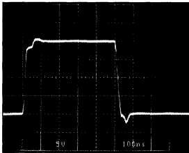
Large-Signal Transient ( A_V = 1 )
