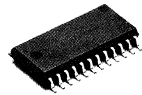
Outline 24P2N-B 1.27mm pitch 300mil SOP (5.3mm × 15.02mm × 1.8mm)
