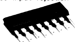
Outline 8P5(L) 2.54mm pitch 340mil SIP (2.8mm × 19.0mm × 6.4mm)
