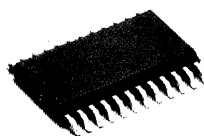
Outline 24P2W-A(FP) 1.27mm pitch 450mil SOP (8.4mm × 15.0mm × 2.0mm)
