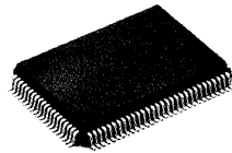
Outline 100P6S-A 0.65mm pitch QFP (20.0mm × 14.0mm × 2.8mm)
