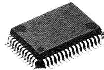
Outline 56P6N-A 0.8mm pitch QFP (14.0mm × 10.0mm × 2.8mm)
