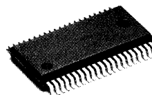
Outline 42P2R-A 0.8mm pitch 450mil SSOP (8.4mm x 17.5mm x 2.0mm)
