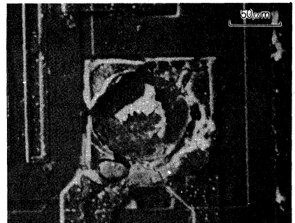
Fig.7 Enlarged micrograph of corroded Aluminum bonding pad
