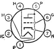
Miniature type used in compact radio equipment as a local oscillator in FM and other high-frequency circuits. It may also be used as a class C rf amplifier. In such service, it delivers
