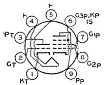
unit is used in low-frequency oscillator or sync circuits. Outline 14, OUTLINES SECTION. Heater volts (ac/dc), 8.4; amperes, 0.45; warm-up time (average) 11 seconds. Except for heater rating, this type is identical with miniature type 6AW8-A.
