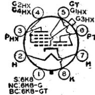
OUTLINES SECTION. Types 6K8-G and 6K8-GT are DISCONTINUED types listed for reference only. Tubes require octal socket and may be mounted in any position.
