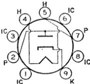
Novar type used as damper tube in horizontal-deflection circuits of black-and-white television receivers employing series-connected heater strings. Outline 54, OUTLINES SECTION.
