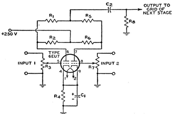
$C_1=10 \mu\text{f}$ , electrolytic, 25 v.
