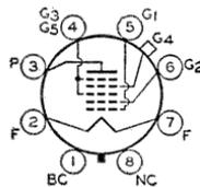
ohm; plate resistance (approx.), 0.6 megohm; plate ma., 0.6; grids-No.3-and-No.5 ma., 0.7; grid-No.2 ma., 1.2; grid-No.1 ma., 0.035; total cathode ma., 2.5 (4 max); conversion transconductance, 250  $\mu$ mhos. This type is used principally for renewal purposes.
