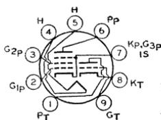
Miniature type used in television-receiver applications; the pentode unit is used as a video amplifier; the triode unit is used as a sync separator. Outline 12, OUTLINES SECTION. Tube
