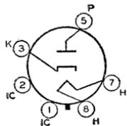
Glass octal type used as damper tube in magnetic-deflection circuits of television receivers. Outline 22, OUTLINES SECTION. This type may be supplied with pin No.1 omitted. Tube requires octal socket and may be mounted in any position. It is especially important that this tube, like other power-handling tubes, be adequately ventilated. Type 25W4-GT is used principally for renewal purposes.
