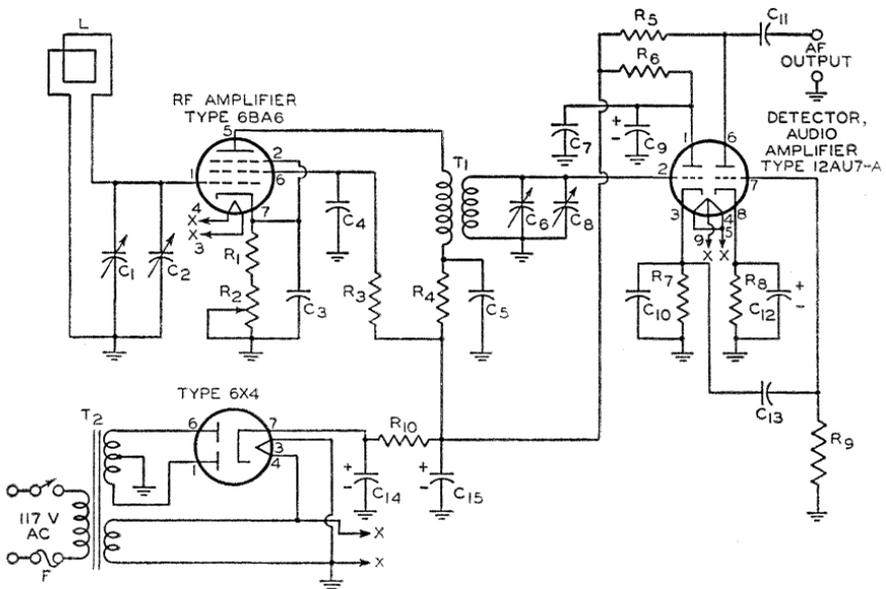
C<sub>1</sub>, C<sub>6</sub>=Ganged tuning capacitors, 10-365  $\mu\mu\text{f}$
