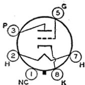
Glass octal type used in single-ended or push-pull audio-frequency power amplifiers of the direct-coupled type in which a driver tube develops positive grid bias for the 6AC5-GT output stage. Outline 22, OUTLINES SECTION. This type may be supplied with pin No. 1 omitted. Tube requires octal socket. Heater
