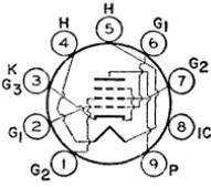
Novar type used in horizontal-deflection-amplifier circuits of television receivers employing series-connected heater strings. Outline 54, OUTLINES SECTION, except vertical dimensions
