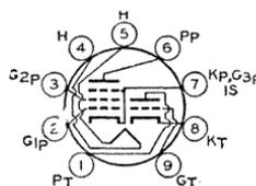
Heater volts (ac/dc), 4.7; amperes, 0.6; warm-up time (average), 11 seconds. Except for heater rating, this type is identical with miniature type 6U8-A.
