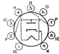
Heater volts (ac/dc), 22.4; amperes, 0.450; warm-up time (average), 11 seconds. Except for heater rating, this type is identical with novar type 6BH3.
