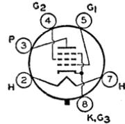
in any position. Heater volts (ac/dc), 50; amperes, 0.15. Peak heater-cathode volts, heater negative with respect to cathode, 200 *max*. Except for heater ratings and heater-cathode voltage, this type is identical with glass octal type 6FE5.
