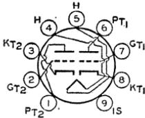
Miniature type used in direct-coupled, cathode-drive, rf amplifier circuits in vhf television tuners. In such circuits, one triode unit is used as the direct-coupled, grounded-cathode driver for the other unit. Outline 12, OUTLINES SECTION. Tube requires miniature nine-contact socket and may be mounted in any position. Heater volts (ac/dc), 6.3; amperes, 0.4. Type 6BZ8 is used principally for renewal purposes.
