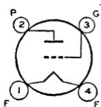
Glass type used as rf voltage amplifier in ac-operated receivers. Outline 43, OUTLINES SECTION. Tube requires four-contact socket. Filament volts (ac/dc), 1.5; amperes, 1.05. Typical operation as class A<sub>1</sub> amplifier: plate volts, 180 max; grid volts, -14.5, plate ma., 6.2; plate resistance, 7300 ohms; transconductance, 1150 μmhos; amplification factor, 8.3. This is a DISCONTINUED type listed for reference only.
