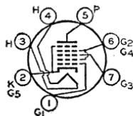
Miniature type used as rf amplifier in low B+ voltage automobile radio receivers operating directly from 12-volt storage-battery systems. Outline 11, OUTLINES SECTION. Grid No.1 and grid No.3 are independent control electrodes. Tube requires miniature seven-contact socket and may be mounted in any position. This type is used principally for renewal purposes.
