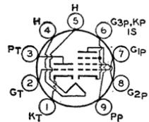
arator, sync-amplifier, and sync-clipper circuits. Outline 14, OUTLINES SECTION. Tube requires miniature nine-contact socket and may be mounted in any position.
