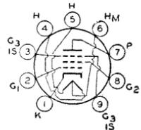
OUTLINES SECTION. Tubes require miniature nine-contact socket and may be mounted in any position. Type 12BY7 is a DISCONTINUED type listed for reference only.
