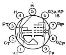
oscillator and phase-splitter circuits. Outline 14, OUTLINES SECTION. Tube requires miniature nine-contact socket and may be operated in any position. Heater volts (ac/dc), 8.4; amperes, 0.45. Except for heater ratings, the 8BA8-A is identical with miniature type 6BA8-A.
