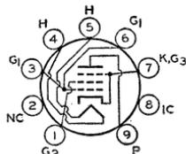
and operating at ultor voltages up to 18 kilovolts. Also used in the audio output stage of television and radio receivers. This type has a controlled heater warm-up time for use in receivers employing series-connected heater strings. Outline 18, OUTLINES SECTION. Tube requires miniature nine-contact socket and may be mounted in any position.
