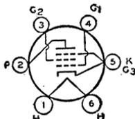
Glass type used in audio output stage of ac/dc receivers. Outline 43, OUTLINES SECTION. Tube requires six-contact socket. Heater volts (ac/dc), 25; amperes, 0.3. This type is electrically identical with type 25A6. Type 43 is used principally for renewal purposes.
