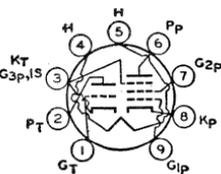
Miniature type used as a combined vhf oscillator and mixer tube in television receivers employing a series-connected heater string. Outline 12, OUTLINES SECTION. Heater volts (ac/dc), 4.7; amperes, 0.6; warm-up time (average), 11 seconds. Tube requires miniature nine-contact socket and may be operated in any position. This type is used principally for renewal purposes.
