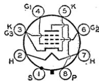
up to 18 megacycles per second (approx.). Two separate cathode terminals enable the input and output circuits to be effectively isolated from each other. Outline 3, OUTLINES SECTION. Tube requires octal socket and may be mounted in any position.
