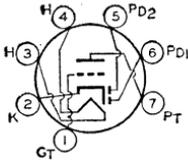
Miniature type used as combined detector, amplifier, and avc tube primarily in automobile radio receivers operating from a 12-volt storage battery. Outline 11, OUTLINES SECTION. Heater volts (ac/dc), 12.6; amperes, 0.15. Except for heater rating, this type is identical with miniature type 6BF6.
