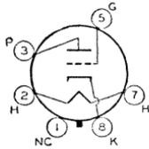
Glass octal type used as detector, amplifier, or oscillator in ac/dc radio equipment. Outline 24, OUTLINES SECTION. This type may be supplied with pin No.1 omitted. Heater volts (ac/dc), 12.6; amperes, 0.15. Except for heater rating and base, this type is identical with glass-octal type 6J5-GT. Type 12J5-GT is used principally for renewal purposes.
