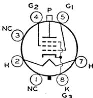
Glass octal type used in horizontal-deflection-amplifier circuits of high-efficiency deflection circuits of television receivers employing series-connected heater strings. Outline 37, OUT-
