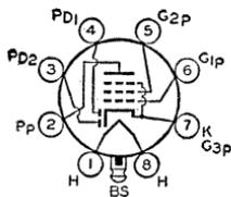
Glass lock-in type used as combined detector, amplifier, and avc tube. Outline 15, OUTLINES SECTION. Tube requires lock-in socket. Heater volts (ac/dc), 6.3; amperes, 0.3. Characteristics and maximum ratings of pentode unit as class A<sub>1</sub> amplifier: plate volts, 250 (300 *max*); grid-No.2 supply volts, 300 *max*; grid-No.2 volts, 100 *max*; grid-No.1 volts, -3
