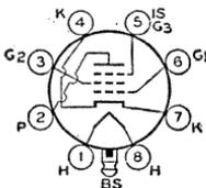
Glass lock-in type used as rf or if amplifier in radio receivers. Outline 15, OUTLINES SECTION. Tube requires lock-in socket. Heater volts (ac/dc), 6.3; amperes, 0.45. This type is the same as type 7V7 except for socket connections. Type 7W7 is used principally for renewal purposes.
