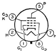
prox.) 27000 ohms; for plate volts, 200; grid-No.2 volts, 125; grid-No.1 volts, -17; plate ma., 40; grid-No.2 ma., 1.1.
