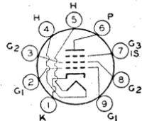
SECTION. Tube requires miniature nine-contact socket and may be mounted in any position.
