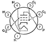
SECTION. Tube requires miniature seven-contact socket and may be mounted in any position. Heater-voltage range (ac/dc), 10.0 to 15.9; amperes (approx.) at 12.6 volts, 0.4. Maximum ratings and characteristics are the same as those of the tetrode unit of miniature type 12DL8.
