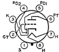
Maximum ratings and typical operation of triode unit as class A<sub>1</sub> amplifier: plate volts, 250 *max*; grid volts, -9; amplification factor, 16; plate resistance (approx.), 8500 ohms; transconductance, 1900 μmhos; plate ma., 9.5; plate dissipation, 2.5 *max* watts; peak heater-cathode volts, 90 *max*. For diode-operation curves, refer to type 6AV6. Type 6SR7 is used principally for renewal purposes.
