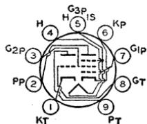
unit is used in low-frequency oscillator, sync-separator, sync-clipper, and phase-splitter circuits. Outline 12, OUTLINES SECTION. Tube requires miniature nine-contact socket and may be mounted in any position. For curves of average plate characteristics, refer to type 6AN8. The pentode-unit curve for the 6AN8 applies for this type except that grid No.3, heater, and internal shield (pin 5) are connected to ground.
