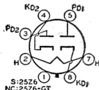
either the ac/dc type or the voltage-doubler type. Outlines 6 and 22, respectively, OUTLINES SECTION. Type 25Z6-GT may be supplied with pin No.1 omitted. Tubes require octal socket and may be mounted in any position. Type 25Z6 is a DISCONTINUED type listed for reference only.
