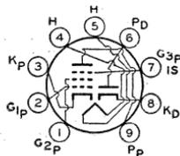
used as an audio detector, video detector, or dc restorer. Outline 12, OUTLINES SECTION. Tube requires miniature nine-contact socket and may be mounted in any position.
