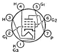
OUTLINES SECTION. Tube requires miniature seven-contact socket and may be mounted in any position.
