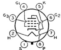
plate resistance (approx.), 1 megohm; transconductance, 1850 μmhos; plate ma., 9; grid-No.2 ma., 2; plate dissipation, 2.25 *max* watts; grid-No.2 input, 0.35 *max* watts. Type 6SS7 is used principally for renewal purposes.
