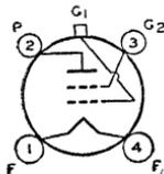
Glass type used as rf amplifier or biased detector in battery-operated receivers. Maximum over-all length, 5-1/32 inches; maximum diameter, 1-13/16 inches. Tube requires four-contact socket. Filament volts (dc), 2.0; amperes, 0.06. Typical operation as class A<sub>1</sub> amplifier: plate volts, 180 max; grid-No.2 ma., 0.4 max; plate resistance, greater than 1 megohm; plate ma., 1.7; transconductance, 650 μmhos. This is a DISCONTINUED type listed for reference only.
