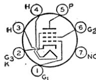
peak heater-cathode volts, 90 *max*. Within its maximum ratings, type 6AR5 is equivalent in performance to glass-octal type 6K6-GT. Type 6AR5 is used principally for renewal purposes.
