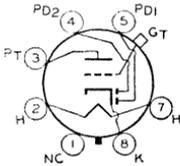
Glass octal type used as combined detector, amplifier, and avc tube in radio receivers. Outline 39, OUTLINES SECTION. Heater volts (ac/dc), 6.3; amperes, 0.15. Typical operation as class A<sub>1</sub> amplifier: plate volts, 250 *max*; grid volts, -3; plate ma., 1.2; plate resistance (approx.), 62000 ohms; amplification factor, 65; transconductance, 1050 μmhos. For diode operation curves, refer to type 6AV6. Type 6T7-G is a DISCONTINUED type listed for reference only.
