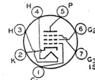
0.6; warm-up time (average), 11 seconds. Peak heater-cathode volts: heater negative with respect to cathode, 300 *max*; heater positive with respect to cathode, 200 *max* (the dc component must not exceed 100 volts). Except for heater and heater-cathode ratings, this type is identical with miniature type 6CF6.
