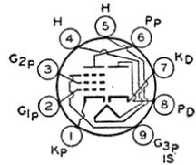
The pentode unit is used as an if amplifier, video amplifier, or agc amplifier. The high-perveance diode is used as an audio detector, video detector, or dc restorer. Outline 12, OUTLINES SECTION. Tubes require miniature nine-contact socket and may be mounted in any position. Type 6AM8 is a DISCONTINUED type listed for reference only.
