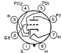
unit as class A<sub>1</sub> amplifier: plate volts, 250 *max*; plate dissipation, 2.5 *max* watts. For diode operation curves, refer to type 6AV6. Type 6ST7 is a DISCONTINUED type listed for reference only.
