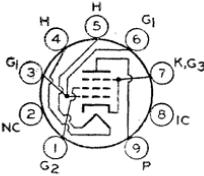
Miniature type used as a vertical-deflection-amplifier tube in television receivers employing 110-degree picture-tube systems. Outline 14, OUT-LINES SECTION. Tube requires miniature nine-contact socket and may be operated in any position.
