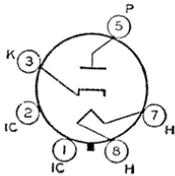
Glass octal types used as damper tubes in horizontal deflection circuits of television receivers employing series-connected heater strings. Outline 22, OUTLINES SECTION. Heater volts (ac/dc), 16.8; amperes, 0.45; warm-up time (average), 11 seconds. Except for heater rating, these types are identical with glass octal types 6AX4-GT and 6AX4-GTB, respectively.
