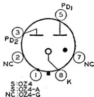
Metal types OZ4 and OZ4-A and glass octal type OZ4-G are used in vibrator-type B-supply units. Both have ionically heated cathodes, require octal sockets, and may be mounted in any position. OZ4 and OZ4-A, Outline 2, OUTLINES SECTION. OZ4-G dimensions: maximum over-all length, 2-5/8 inches; maximum diameter, 1-1/16 inches; T-7 bulb; dwarf-shell octal 5-pin base. Base of OZ4-G has no pin No. 2. Shell of OZ4
