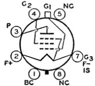
in avc circuits, the 1N5-GT should be only partially controlled to avoid excessive reduction in receiver sensitivity with large signal input. Filament volts (dc), 1.4; amperes, 0.05. Characteristics as class A<sub>1</sub> amplifier: plate and grid-No.2 volts, 90 (110 max); grid-No.1 volts, 0; plate resistance (approx.), 1.5 megohms; transconductance, 750 μmhos; plate ma., 1.2; grid-No.2 ma., 0.3.
