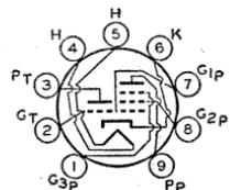
Heater volts (ac/dc), 4.7; amperes, 0.6; warm-up time (average), 11 seconds. Except for heater rating, this type is identical with miniature type 6X8.
