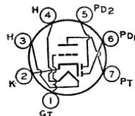
11, OUTLINES SECTION. Tube requires miniature seven-contact socket and may be mounted in any position.
