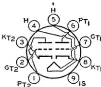
Miniature type used as rf amplifier and self-oscillating mixer in FM/AM radio receivers. Outline 12, OUTLINES SECTION. Tube requires nine-contact socket and may be operated in any position. Heater volts (ac/dc), 6.3; amperes, 0.435. With plate volts of 250 and grid volts of -2.3, class A<sub>1</sub> characteristics of each unit are: plate ma, 10; plate resistance (approx.), 9700 ohms; transconductance, 5900  $\mu$ mhos; amplification factor, 57.
