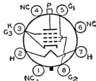
plate-voltage rating (*Absolute Maximum*) of 6600 volts, a maximum plate-dissipation rating of 15 watts, and a maximum bulb-temperature rating (at hottest point) of 210°C. Type 6CD6-G is a DISCONTINUED type listed for reference only.
