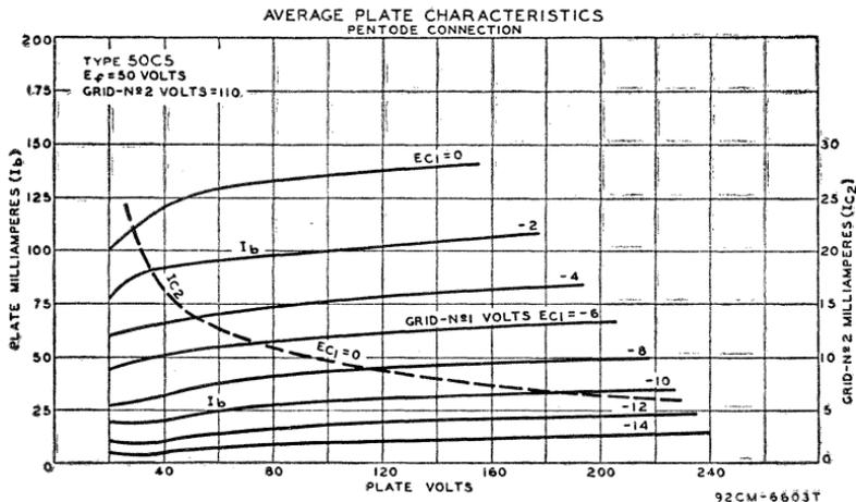
As a power amplifier (class  $A_1$ ), the 50C5 is recommended for use either singly or in push-pull combination in the power-output stage of "ac/dc" receivers. The operating values shown under typical operation have been determined on the basis that grid-No.1 current does not flow during any part of the input cycle.
