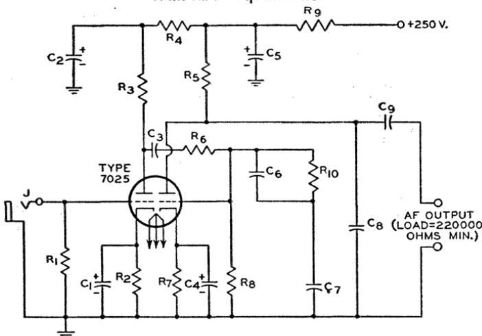
$C_1 C_4=25 \mu\text{f}$ , electrolytic, 25 v.
