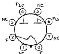
octal socket. Either type may be supplied with pins 3, 5, and 7 omitted. Vertical mounting is preferred but horizontal mounting is permissible if pins 1 and 4 are in vertical plane. The coated filament is designed to operate from the ac line through a step-down transformer. The voltage at the filament terminals should be 5.0 volts at an average line voltage of 117 volts. It is especially important that these tubes,
