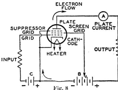
its negative potential with respect to the plate, the suppressor grid retards the flight of secondary electrons and diverts them back to the plate.
