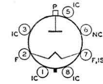
Glass octal type used as high-voltage rectifier in television receivers. Maximum over-all length, 3-9/16 inches; maximum seated length, 3 inches; maximum diameter, 1-9/16 inches. Tube requires octal socket and may be operated in any position. For installation and application considerations, refer to type 1B3-GT.
