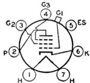
Glass type used as detector or amplifier in radio receivers. Outline 45, OUTLINES SECTION. Heater volts (ac/dc), 6.3; amperes, 0.3. For electrical characteristics, refer to type 6J7. Type 6D7 is a DISCONTINUED type listed for reference only.
