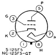
Heater volts (ac/dc), 12.6; amperes, 0.15. Except for heater rating, these types are identical with metal type 6SF5 and glass octal type 6SF5-GT, respectively. Type 12SF5-GT is a **DISCONTINUED** type listed for reference only.
