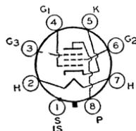
Metal type used in rf and if stages of picture amplifier of television receivers particularly those employing automatic-gain control. Outline 3, OUTLINES SECTION. Tube requires octal socket. Heater volts (ac/dc), 6.3; amperes, 0.45. Maximum ratings as class A<sub>1</sub> amplifier: plate and grid-No.2 supply volts, 300 *max*; grid No.3, connect to cathode at socket; grid-
