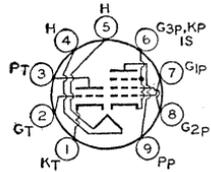
Miniature type used in television receivers employing series-connected heater strings. Pentode unit is used as video amplifier; triode unit is used in sound if amplifier, sweep-oscillator, sync-separator, sync-amplifier, and sync-clipper circuits. Outline 14, **OUTLINES SECTION**. Heater volts (ac/dc), 8; amperes, 0.6; warm-up time (average), 11 seconds. Except for heater rating, this type is identical with type 6CX8.
