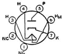
plate circuit. This heater section is not to be used as a panel-lamp shunt. Outline 13, OUTLINES SECTION. Tubes require miniature seven-contact socket and may be operated in any position.
