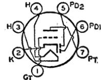
0.15. Except for heater rating, this type is identical with miniature type 6AV6.
