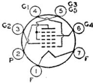
Miniature type used in low-drain battery-operated receivers. Outline 11, OUTLINES SECTION. Tube requires miniature seven-contact socket and may be mounted in any position. Filament volts (dc), 1.4; amperes, 0.05. Typical operation as converter: plate and grid-No.2 volts, 90 (110 *max*); grids-No.3-and-No.5 supply volts, 110 *max*; grids-No.3-and-No.5 volts, 45 (65 *max*); grid-No.4 volts, 0; grid-No.1
