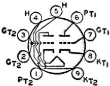
vertical-deflection circuits, and unit No.2 is a low-mu triode unit used as a vertical-deflection amplifier. Outline 14, OUTLINES SECTION. Tube requires miniature nine-contact socket and may be mounted in any position. For curve of average plate characteristics, Unit No.2, refer to type 6DR7.
