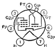
Glass type adaptable to circuit design in several ways. Outline 40, OUTLINES SECTION. Heater volts (ac/dc), 6.3; amperes, 0.3. Typical operation as class A<sub>1</sub> amplifier: pentode unit—plate volts, 250 max; grid-No.2 volts, 100; grid-No.1 volts, -3; plate resistance, 0.85 megohm; transconductance, 1100 μmhos; plate ma., 6.5; grid-No.2 ma., 1.5; triode unit—plate volts,
