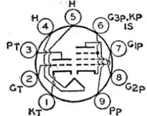
heater strings. The pentode unit is used as an if amplifier, video amplifier, agc amplifier, or reactance tube. The triode unit is used in low-frequency oscillator, sync-separator, sync-clipper, and phase-splitter circuits. Outline 14, OUTLINES SECTION. Tubes require miniature nine-contact socket and may be mounted in any position. Type 6AW8 is a discontinued type listed for reference only.
