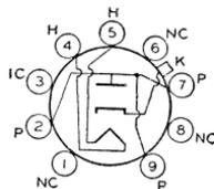
maximum seated length 2-25/32 inches. Tube requires miniature nine-contact socket and may be mounted in any position. It is especially important that this tube, like other power-handling tubes, be adequately ventilated.
