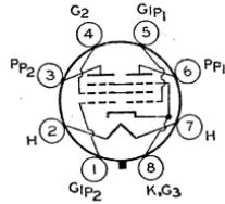
It is especially important that this tube, like other power-handling tubes, be adequately ventilated. Heater voltage (ac/dc), 6.3; amperes, 1.52.
