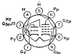
Miniature type used in television receivers having series-connected heater strings. Pentode used as video or audio if amplifier; triode used as sync amplifier, sync clipper, sync separator, or vertical oscillator. Outline 12, OUTLINES SECTION. Tube requires miniature nine-contact socket and may be operated in any position. Heater volts (ac/dc), 5.2; amperes, 0.6; heater warm-up time (average), 11 seconds.
