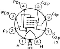
Glass lock-in type used as combined detector, amplifier, and avc tube in ac/dc radio receivers. Outline 15, OUTLINES SECTION. Tube requires lock-in socket. Heater volts (ac/dc), 12.6; amperes, 0.15. Except for heater rating, this type is electrically identical with lock-in type 7R7. Type 14R7 is used principally for renewal purposes.
