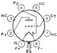
Glass lock-in type used as combined detector and amplifier in battery-operated receivers. Outline 15, OUTLINES SECTION. Tube requires lock-in socket. Filament volts (dc), 1.4; amperes, 0.05. For electrical characteristics, refer to glass-octal type 1H5-GT. Type 1LH4 is used principally for renewal purposes.
