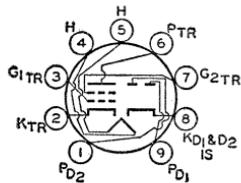
units are used for AM signal detection and automatic-volume control; the tetrode unit is used as the driver for a transistorized power-output stage. Outline 14, OUTLINES SECTION. Tube requires miniature nine-contact socket and may be mounted in any position.
