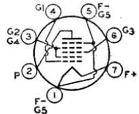
may be mounted in any position. For general discussion of pentagrid types, see *Frequency Conversion* in ELECTRON TUBE APPLICATIONS SECTION.
