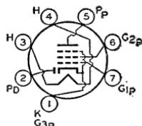
automatic-volume-controlled audio amplifier. Outline 11, **OUTLINES SECTION**. Tube requires miniature seven-contact socket and may be mounted in any position.
