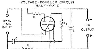
$R_1$  = PROTECTIVE RESISTOR
