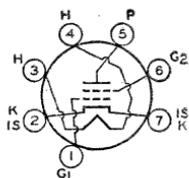
peres, 0.6; warm-up time (average), 11 seconds. Except for heater rating, this type is identical with miniature type 6CY5.
