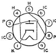
Miniature type used as damper tube in horizontal-deflection circuits of television receivers employing series-connected heater strings. Outline 14, OUTLINES SECTION. Tube requires miniature nine-contact socket and may be mounted in any position. Socket terminals 2, 6, 7, and 9 should not be used as tie points. It is especially important that this tube, like other power-handling tubes, be adequately ventilated.
