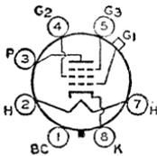
Glass octal type used as biased detector or high-gain audio amplifier in ac/dc radio receivers. Outline 23, OUTLINES SECTION. Heater volts (ac/dc), 12.6; amperes, 0.15. Except for heater rating, this type is identical with glass-octal type 6J7-GT. Type 12J7-GT is used principally for renewal purposes.
