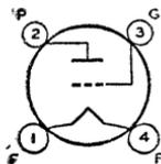
Glass type used as voltage amplifier or detector in battery-operated receivers. Outline 34 or 35, OUTLINES SECTION. Tube requires four-contact socket. Filament volts (dc), 2.0; amperes, 0.06. Except for interelectrode capacitances, this type is electrically identical with glass-octal type 1H4-G. Type 30 is a DISCONTINUED type listed for reference only.
