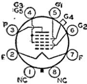
Glass octal type used in battery-operated receivers. Outline 39, OUTLINES SECTION. Tube requires octal socket. Filament volts (dc), 2.0; amperes, 0.06. Typical operation as converter: plate volts, grids-No.3-and-No.5 volts, grid-No.2 supply volts, grid-No.4 volts, and grid-No.1 resistor are same as for type 1C7-G; plate ma., 1.3; grids-No.3-and-No.5 ma., 2.4; grid-No.2 ma., 2.3; grid-No.1 ma., 0.2. This is a DISCONTINUED type listed for reference only.
