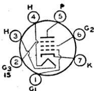
Miniature type used as rf amplifier in low B+ voltage automobile radio receivers operating directly from 12-volt storage-battery systems. Outline 11, OUTLINES SECTION. Tube requires miniature seven-contact socket and may be mounted in any position. Heater voltage range (ac/dc), 10.0 to 15.9; amperes (approx.) at 12.6 volts, 0.19. This type is used principally for renewal purposes.
