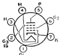
Tube requires miniature seven-contact socket and may be mounted in any position.
