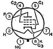
Tube requires octal socket and may be mounted in any position. For typical operation as push-pull class A<sub>1</sub>, class AB<sub>1</sub> (within maximum ratings), and class AB<sub>2</sub> amplifier, and for curves of average plate characteristics, refer to type 6L6-GC.
