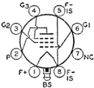
Glass lock-in type used as rf or if amplifier in battery-operated receivers. Outline 15, OUTLINES SECTION. Tube requires lock-in socket. Filament volts (dc), 1.4; amperes, 0.05. Typical operation as class A<sub>1</sub> amplifier: plate and grid-No.2 (screen-grid) volts, 90 (110 max); grid-No.1 volts, 0; plate ma., 1.6; grid-No.2 ma., 0.35; plate resistance (approx.), 1.1 megohms; transconductance, 800 μmhos. This type is used principally for renewal purposes.
