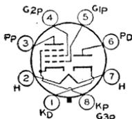
μmhos; load resistance, 4500 ohms; output watts, 0.77. Maximum ratings of rectifier unit: peak inverse plate volts, 350; peak plate ma., 450; dc output ma., 75; peak heater-cathode volts, 175. This is a DISCONTINUED type listed for reference only.
