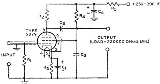
$C_1=25 \mu\text{f}$ , electrolytic, 25 v.
