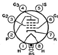
max watts; grid-No.2 input, 0.75 max watt; grid No.3 and internal shield connected to cathode at socket; plate resistance (approx.), greater than 1 megohm; transconductance, 4200  $\mu$ hos; cathode-bias resistor, 250 ohms; plate ma., 6; grid-No.2 ma., 2; peak heater-cathode volts, 90 max. This type is used principally for renewal purposes.
