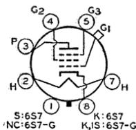
No.2 volts, see curve page 66; grid-No.2 supply volts, 300 max; grid-No.1 volts, -3 (0 max); grid No.3 connected to cathode at socket; plate ma., 8.5; grid-No.2 ma., 2; plate resistance (Approx.), 1.0 megohm; transconductance, 1750 μmhos; plate dissipation, 2.25 max watts; grid-No.2 input: for grid-No.2 voltages up to 150 volts, 0.25 max watt; for grid-No.2 voltages between 150 and 300 volts, see curve page 66. Peak heater-cathode volts, 90 max.
