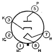
29, OUTLINES SECTION. Tubes require octal socket and may be mounted in any position. These types may be supplied with pin No.1 omitted. Socket terminals 1, 2, 4, and 6 should not be used as tie points. It is especially important that these tubes, like other power-handling tubes, be adequately ventilated. Type 6AU4-GT is a **DISCONTINUED** type listed for reference only. For curve of average plate characteristics for 6AU4-GTA, see page 67.
