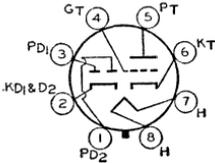
Glass octal type used as FM detector and audio amplifier in circuits which require diode and triode units with separate cathodes. Outline 22, OUTLINES SECTION. Tube requires octal socket. Heater volts (ac/dc), 6.3; amperes, 0.3. Ratings and characteristics of triode unit as class A<sub>1</sub> amplifier: plate volts, 250 *max.*; grid volts, -2; amplification factor, 70; plate resistance (approx.), 44000 ohms; transconductance,
