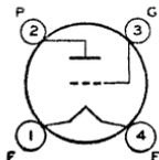
Glass type used in output stage of radio receivers. Outline 43, OUTLINES SECTION. Tube requires four-contact socket. Filament volts (ac/dc), 2.5; amperes, 1.5. Typical operation as class A<sub>1</sub> amplifier: plate supply volts, 275 *max*; grid volts, -56; cathode-bias resistor, 1550 ohms; amplification factor, 3.5; plate resistance, 1700 ohms; transconductance, 2050
