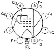
Lock-in type used as rf or if amplifier in battery-operated receivers. Outline 15, OUTLINES SECTION. Tube requires lock-in socket. Filament volts (dc), 1.4; amperes, 0.05. Typical operation as class A<sub>1</sub> amplifier: plate volts, 90 (110 max); grid-No.2 volts, 45 (110 max); grid-No.1 volts, 0; plate resistance (approx.), greater than 1 megohm; transconductance, 800 μmhos; plate ma., 1.7; grid-No.2 ma., 0.4. This type is used principally for renewal purposes.
