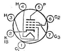
TION. Tube requires miniature seven-contact socket and may be operated in any position. For curves of average characteristics, refer to type 6EX6.
