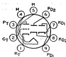
controlled warm-up time for use in series-connected heater strings. Outline 12, OUT-LINES SECTION. Tube requires miniature nine-contact socket and may be operated in any position.
