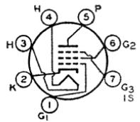
Tube requires miniature seven-contact socket and may be mounted in any position.
