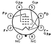
0.8 megohm; transconductance, 800 μmhos; load resistance, 25000 ohms; output watts, 0.1. This is a DISCONTINUED type listed for reference only.
