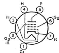
6SG7. The low value of grid-No.1-to-plate capacitance minimizes regenerative effects, while the high transconductance makes possible high signal-to-noise ratio.
