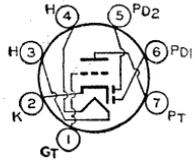
max); grid volts, 0; amplification factor, 55; plate resistance (approx.), 45000 ohms; transconductance, 1200 μmhos; plate ma., 0.75; total cathode ma., 20 max; peak heater-cathode volts, 30 max. Maximum rating of each diode unit: plate ma., 1 max. This type is used principally for renewal purposes.
