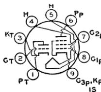
Miniature type used in diversified applications in television receivers employing series-connected heater strings. The pentode unit is used as a general-purpose amplifier tube; the triode unit is used in vertical-deflection-oscillator, sync-separator, sync-clipper, and sync-amplifier circuits. Outline 12, OUTLINES SECTION. Tube requires miniature nine-contact socket and may be mounted in any position.
