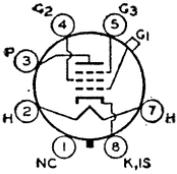
connected to cathode at socket; grid-No.1 volts, -3; plate resistance (approx.), 0.8 megohm; transconductance, 1600  $\mu$ mhos; plate ma., 8.2; grid-No.2 ma., 2; plate dissipation, 2.25 *max* watts; grid-No.2 input, 0.25 *max* watt. This is a DISCONTINUED type listed for reference only.
