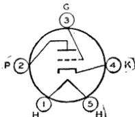
Glass type used as voltage amplifier or detector in ac-operated receivers. Outline 34 or 35, OUTLINES SECTION. Tube requires five-contact socket. Heater volts (ac/dc), 2.5; amperes, 1.75. Maximum ratings and characteristics as class A<sub>1</sub> amplifier: plate volts, 250 max; grid volts, -21; amplification factor, 9; plate resistance, 9250 ohms; transconductance, 975 μmhos; plate ma., 5.2. This type is used principally for renewal purposes.
