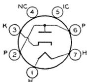
Miniature type used as detector tube in portable FM receivers and in portable high-frequency measuring equipment. Outline 11, OUTLINES SECTION. Tube requires miniature seven-contact socket. Heater volts (ac/dc) 1.4; amperes, 0.15.
