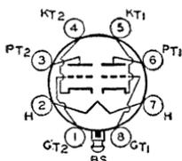
Glass lock-in type used as amplifier or oscillator in radio equipment. Outline 15, OUTLINES SECTION, except over-all length is 2-9/32 *max* inches and seated length is 1-3/4 inches. Tube requires lock-in socket. Heater volts (ac/dc), 6.3; amperes, 0.3. Characteristics and maximum ratings as class A<sub>1</sub> amplifier (each unit): plate supply volts, 250 (300 *max*); grid
