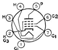
Miniature type used as audio amplifier in television receivers employing series-connected heater strings. Outline 13, OUTLINES SECTION. Heater volts (ac/dc), 4.7; amperes, 0.6;
