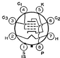
Metal type used in rf and if stages of picture amplifier and the first stages of the video amplifier of television receivers. It is also used as a mixer or oscillator tube in low-frequency applications. Outline 3, OUTLINES SECTION. Tube requires octal socket. When tube
