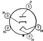
Heater volts (ac/dc), 22.4; amperes, 0.45; warm-up time (average), 11 seconds. Except for heater rating, this type is identical with glass octal type 6DE4.
