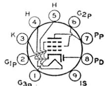
and may be operated in any position. Heater volts (ac/dc), 20; amperes, 0.1. Except for heater rating, this type is identical with miniature type 6EQ7.
