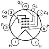
Glass type used in ac-operated receivers. Outline 40, OUTLINES SECTION. Tube requires small seven-contact (0.75-inch, pin-circle diameter) socket. Except for its heater rating (2.5 volts ac/dc; 0.8 ampere) and its interelectrode capacitances, the 2A7 has electrical characteristics identical with type 6A8. Complete shielding of this tube is generally necessary. Type 2A7 is a DISCONTINUED type listed for reference only.
