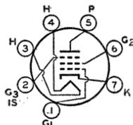
TION. This type is identical with miniature type 6AU6 except that it has a controlled hum characteristic.
