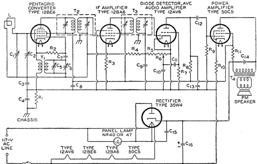
C<sub>1</sub> C<sub>5</sub>=Ganged tuning capacitors; C<sub>1</sub>, 10-365  $\mu$ f; C<sub>5</sub>, 7-115  $\mu$ f
