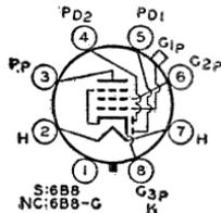
300 *max*; grid-No.2 volts, 125 *max*; grid-No.2 supply volts, 300 *max*; grid-No.1 volts, positive-bias value, 0 *max*; plate dissipation, 3.0 *max* watts (6B8), 2.25 *max* watts (6B8-G); grid-No.2 input, 0.3 *max* watt.
