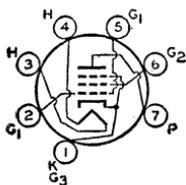
Miniature type used in audio output stage of compact ac/dc radio receivers. Outline 13, OUTLINE SECTION. Tube requires miniature seven-contact socket and may be mounted in any position. Heater volts (ac/dc), 32; amperes, 0.1.
