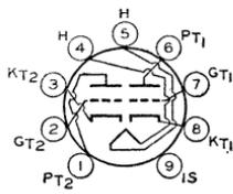
for the other unit. This type is also used in push-pull cathode-drive rf amplifiers. Outline 12, **OUTLINES SECTION**. Tube requires miniature nine-contact socket and may be mounted in any position. For typical operation as a resistance-coupled amplifier, refer to **RESISTANCE-COUPLED AMPLIFIER SECTION**.
