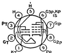
Miniature type used in color and black-and-white television receivers employing series-connected heater strings. Triode unit is used in high-gain, sound-if stages and in sync-separator,
