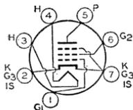
**OUTLINES SECTION**. Tube requires miniature seven-contact socket and may be mounted in any position.
