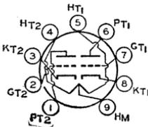
Miniature type used as push-pull cathode-drive amplifier or frequency converter in the FM and television broadcast bands. Outline 12, **OUTLINES SECTION**. Tube requires
