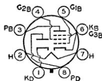
plate-supply impedance, 15 ohms. Typical operation and maximum ratings of beam power unit as class A<sub>1</sub> amplifier: plate and grid-No.2 volts, 110 (117 *max*); grid-No.1 volts, -7.5; plate ma., 40; grid-No.2 ma., 3; plate resistance, 15000 ohms; transconductance, 7500  $\mu$ hos; load resistance, 2000 ohms; output watts, 1.8; plate dissipation, 5 *max* watts; grid-No.2 input, 1 *max* watt. This type is used principally for renewal purposes.
