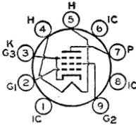
Miniature type used as power amplifier tube in high-fidelity audio equipment. Outline 18, OUTLINES SECTION. Tube requires miniature nine-contact socket and may be mounted in any position. Heater volts (ac/dc), 6.3; amperes, 0.76.
