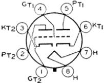
Glass octal types used as combined vertical oscillators and vertical deflection amplifiers, and as horizontal deflection oscillators in television receivers. May also be used in multivibrator
