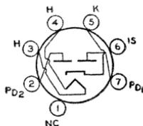
heater is positive with respect to cathode, the dc component of the heater-cathode voltage must not exceed 100 volts. Type 2EN5 is used principally for renewal purposes.
