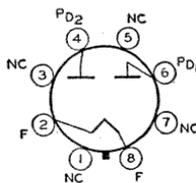
Vertical mounting is preferred, but horizontal mounting is permissible if pins 2 and 4 are in vertical plane. It is especially important that these tubes, like other power-handling tubes, be adequately ventilated. For discussion of Rating Chart, refer to INTERPRETATION OF TUBE DATA.
