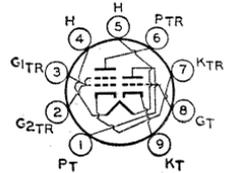
function in automatic station-selection circuits. The triode unit is also used for AM-signal detection and af amplification; the tetrode unit is used as a driver for a transistorized af power-output stage. Outline 14, OUTLINES SECTION. Tube requires miniature nine-contact socket and may be mounted in any position.
