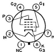
is desirable. Outlines 6, 22, and 22, respectively, **OUTLINES SECTION**. Type 6V6-GT may be supplied with pin No.1 omitted. Tubes require octal socket and may be mounted in any position. These tubes are equivalent in performance to type 6AQ5-A. Refer to type 6AQ5-A for average plate characteristic curves. Except for heater warm-up time, the 6V6-GTA is identical with type 6V6-GT.
