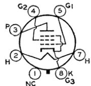
may be supplied with pin No.1 omitted. Refer to miniature type 35C5 for installation, application information, and curves.
