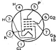
11 seconds, Peak heater-cathode volts: heater negative with respect to cathode, 300 max; heater positive with respect to cathode, 200 max (the dc component must not exceed 100 volts). Except for heater and heater-cathode ratings, this type is identical with miniature type 6DK6.
