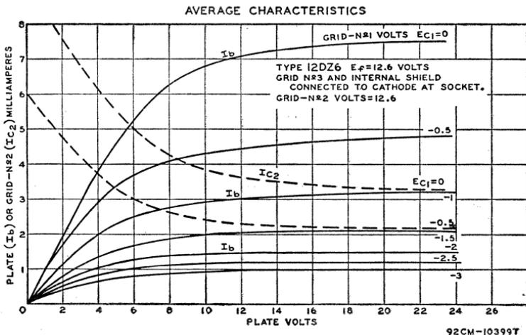
**Characteristics with 12.6 Volts on Heater:**
