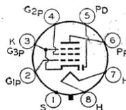
300 *max*; grid-No.2 volts, 100 *max*; grid-No.1 volts, 0 *max*; plate dissipation, 3.5 *max* watts; grid-No.2 input, 0.5 *max* watt; peak heater-cathode volts, 90 *max*. For diode operation curves, refer to type 6AV6. Type 6SF7 is used principally for renewal purposes.
