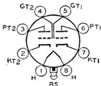
Glass lock-in type used as phase inverter or resistance-coupled amplifier. Outline 15, OUTLINES SECTION. Tube requires lock-in socket. Heater volts (ac/dc), 6.3; amperes, 0.3. For maximum ratings, typical operation as class A<sub>1</sub> amplifier, and curves, refer to glass-octal type 6SL7-GT. Type 7F7 is used principally for renewal purposes.
