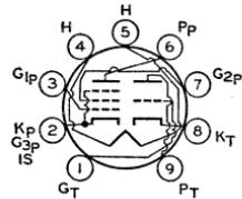
SECTION but maximum seated length is 2 7/8 inches and other vertical dimensions are 1/16 inch shorter than shown. Tube requires miniature nine-contact socket and may be operated in any position.
