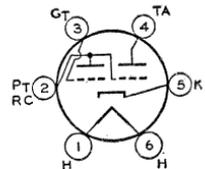
receiver tuning. Outline 34, OUTLINES SECTION. Tube requires six-contact socket. Heater volts (ac/dc), 6.3; amperes, 0.3. For additional considerations, refer to *Tuning Indication with Electron-Ray Tubes* in ELECTRON TUBE APPLICATIONS SECTION.
