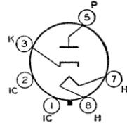
Tube requires octal socket and may be mounted in any position. Socket terminals 1, 2, 4, and 6 should not be used as tie points. It is especially important that this tube, like other power-handling tubes, be adequately ventilated. Power-rectifier operation of this type is not recommended. For curve of average plate characteristics, see page 67.
