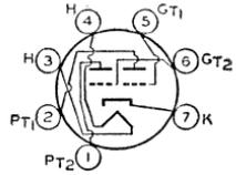
ances, ratings, and typical operation as a class A<sub>1</sub> amplifier, and curves, refer to type 6J6. Maximum ratings and characteristics for mixer service (each unit): plate volts, 150 (300 *max*); cathode-bias resistor, 810 ohms; peak oscillator volts, 3; plate resistance, 10200 ohms; conversion transconductance, 1900  $\mu$ mhos; plate ma., 4.8; plate dissipation, 1.5 *max* watts; peak heater-cathode volts, 90 *max*. Type 19J6 is used principally for renewal purposes.
