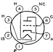
11, OUTLINES SECTION. Tube requires miniature seven-contact socket and may be mounted in any position. Heater volts (ac/dc), 6.3; amperes, 0.15. For maximum ratings, characteristics, and curves, refer to type 12AT7.
