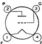
Glass type used as an audio-frequency amplifier. Outline 51, OUTLINES SECTION. Tube requires four-contact socket. Filament volts (ac/dc), 7.5; amperes, 1.25. Typical operation as class A<sub>1</sub> af power amplifier: plate volts, 425 *max*; grid volts, -40; peak af grid volts, 35; plate ma., 18; plate resistance, 5000 ohms; transconductance, 1600  $\mu$ mhos; load resistance,
