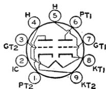
vertical deflection circuits, and unit No.2 is a low-mu triode unit used as a vertical deflection amplifier. Outline 14, OUTLINES SECTION. Tube requires miniature nine-contact socket and may be mounted in any position.
