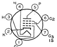
cause of its plate-current cutoff characteristic, this type is used in gain-controlled stages of video if amplifiers. This type is electrically similar to miniature type 6BC6. Outline 11, OUTLINES SECTION. Heater volts (ac/dc), 6.3; amperes, 0.3.
