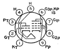
cuits; pentode unit is used as video-output amplifier. Outline 14, **OUTLINES SECTION**. Tube requires miniature nine-contact socket and may be operated in any position. For curves of average characteristics, refer to type 6AW8-A for the triode unit and to type 6EB8 for the pentode unit.
