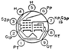
Miniature types used as combined oscillator and mixer tubes in television receivers utilizing an intermediate frequency in the order of 40 megacycles per second. Type 6U8-A has a controlled heater warm-up time for use in television receivers employing series-connected heater strings. Outline 12, OUTLINES SECTION. Tubes require miniature nine-contact socket and may be mounted in any position. Type 6U8 is a DISCONTINUED type listed for reference only.
