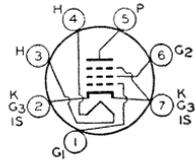
seven-contact socket and may be mounted in any position. For typical operation as resistance-coupled amplifier, refer to RESISTANCE-COUPLED AMPLIFIER SECTION.
