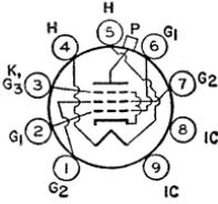
Novar type used in horizontal-deflection-amplifier circuits of television receivers employing series-connected heater strings. Outline 55, OUTLINES SECTION. Tube requires novar nine-contact socket and may be operated in any position. Heater volts (ac/dc), 16.8; amperes, 0.45; warm-up time (average), 11 seconds. Except for heater ratings, this type is identical with type 6GJ5.
