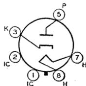
TION. Tubes require octal socket and may be mounted in any position. These types may be supplied with pin 1 omitted. Socket terminals 1, 2, 4, and 6 should not be used as tie points. It is especially important that these tubes, like other power-handling tubes, be adequately ventilated. Heater volts (ac/dc), 18.9; amperes, 0.6; warm-up time (average), 11 seconds. Type 19AU4-GTA is used principally for renewal purposes.
