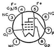
grid-No.1 volts, 0; plate resistance, 0.7 megohm; transconductance, 735  $\mu$ mhos; total cathode ma., 4 max; plate ma., 1.85; grid-No.2 ma., 0.75. This is a DISCONTINUED type listed for reference only.
