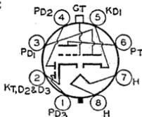
unit as class A<sub>1</sub> amplifier: plate volts, 250 (300 max); grid volts, -2; amplification factor, 100; plate resistance (Approx.), 91000 ohms; transconductance, 1100 μmhos; plate dissipation, 0.5 max watt; plate ma., 0.9; peak heater-cathode volts, 90 max. Maximum plate ma. for diode units, 1.0 max (each unit). Peak heater-cathode volts (diode unit No.1), 90 max. For diode operation curves, refer to type 6AV6. Type 6S8-GT is used principally for renewal purposes.
