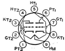
OUTLINES SECTION. Tube requires miniature nine-contact socket and may be mounted in any position. Each triode unit is independent of the other except for the common heater. Use of the 12.6-volt connection with an ac heater supply is not recommended for applications involving low hum. For typical operation as a resistance-coupled amplifier, refer to RESISTANCE-COUPLED AMPLIFIER SECTION.
