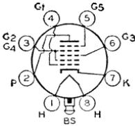
Glass lock-in type used as converter in ac/dc radio receivers. Outline 15, OUTLINES SECTION. Tube requires lock-in socket. Heater volts (ac/dc), 12.6; amperes, 0.15. Except for heater ratings and capacitances, this type is electrically identical with metal type 6SA7 and lock-in type 7Q7. Type 14Q7 is used principally for renewal purposes.
