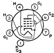
high power output at low plate and screen-grid voltages with a low af grid-No.1 driving voltage. Outline 13, OUTLINES SECTION. Tube requires miniature seven-contact socket and may be mounted in any position.
