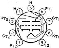
Miniature type used in direct-coupled cathode-drive rf-amplifier circuits of vhf television tuners. In such circuits, one triode unit is used as the direct-coupled grounded-cathode driver for the other unit. Outline 12, OUTLINES SECTION. Tube requires nine-contact socket and may be mounted in any position. Heater voltage (ac/dc), 6.3; amperes, 0.4. This type is used principally for renewal purposes.
