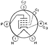
Glass type used as rf amplifier in battery-operated receivers. Outline 40, OUTLINES SECTION. Tube requires five-contact socket. Heater volts (dc), 2.0; amperes, 0.22. Typical operation as class A<sub>1</sub> amplifier: plate volts, 135 max; grid-No.2 (screen-grid) volts, 67.5 max; grid-No.1 volts, -1.5; plate ma., 1.85; grid-No.2 ma., 0.3; plate resistance, 0.80 megohm; transconductance, 750 μmhos. This is a DISCONTINUED type listed for reference only.
