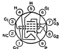
low heater power, and is capable of delivering high power output at low distortion. Double base-pin connections for both grid No.1 and grid No.2 provide cool operation of grids and thus minimize grid emission and permit use of high values of grid-circuit resistance to reduce driving power. Outline 18, OUTLINES SECTION. Tube requires miniature nine-contact socket and may be mounted in any position.
