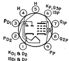
Miniature type used in television receivers employing series-connected heater strings. The pentode unit is used as a video amplifier and the diodes are used as a horizontal phase inverter. Outline 14, **OUTLINES SECTION**. Tube requires miniature nine-contact socket and may be operated in any position.
