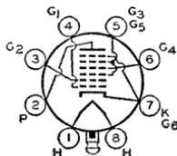
dropping resistor (300 max); grid-No.2 volts, 200 max; plate dissipation, 1 max watt; grids-No.3-and-No.5 input, 0.3 max watt; grid-No.2 input, 0.75 max watt; grid-No.4 volts, -3 (0 max); grid-No.1 resistor, 50000 ohms; plate ma., 3; grids-No.3-and-No.5 ma., 3.2; grid-No.2 ma., 4.2; grid-No.1 ma., 0.4; plate resistance (approx.), 0.7 megohm; conversion transconductance, 550  $\mu$ hos; peak heater-cathode volts, 90 max. This type is used principally for renewal purposes.
