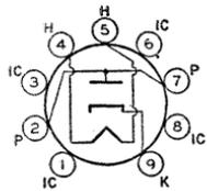
Outline 54, OUTLINES SECTION. Heater volts (ac/dc), 12.6; amperes, 0.6; warm-up time (average), 11 seconds. Except for heater rating, this type is identical with novar type 6AY3.
