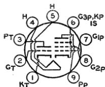
output stage of video amplifier. Outline 14, OUTLINES SECTION. Tube requires miniature nine-contact socket and may be operated in any position. For direct interelectrode capacitances, refer to type 6EB8; curve for average plate characteristics of triode unit is same as for type 6EB8.
