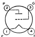
Glass type used as resistance-coupled or impedance-coupled amplifier in battery-operated receivers. Outline 43, OUTLINES SECTION. Filament volts (dc), 5; amperes, 0.25. Characteristics as class A<sub>1</sub> amplifier: plate-supply volts, 180; load resistance, 250000 ohms; grid volts, -3; plate ma., 0.2; plate resistance, 150000 ohms; amplification factor, 30; transconductance, 200  $\mu$ mhos. This is a DISCONTINUED type listed for reference only.
