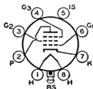
volts, see curve page 69; grid-No.1 volts, positive-bias value, 0 max; grid-No.2 input, for grid-No.2 voltages up to 150 volts, 1.2 max watts (for grid-No.2 voltages between 150 and 300 volts, see curve page 66); plate dissipation, 10 max watts; cathode-bias resistor, 68 ohms; plate ma., 28; grid-No.2 ma., 7; plate resistance (approx.), 0.3 megohm; transconductance, 9500  $\mu$ hos; peak heater-cathode volts, 90 max. Type 7AD7 is a DISCONTINUED type listed for reference only.
