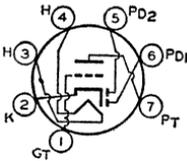
Miniature type used as combined detector, amplifier, and avc tube in compact ac/dc radio receivers. Outline 11, **OUTLINES SECTION**. Heater volts (ac/dc), 12.6; amperes, 0.15. Except for heater rating, this type is identical with miniature type 6A T6.
