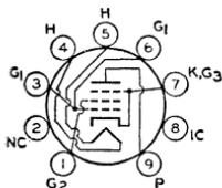
Miniature type used as vertical deflection amplifier and as audio output tube in television and radio receivers employing series-connected heater strings. Outline 18, OUTLINES SECTION.
