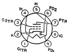
Miniature type used in low B+ voltage automobile radio receivers operating directly from 12-volt storage-battery systems; tetrode unit is used for relay service in a signal-seeker.
