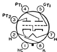
Glass octal type used as class A<sub>1</sub> power amplifier. Heater volts (ac/dc), 25; amperes, 0.3. Characteristics as class A<sub>1</sub> amplifier—input triode: plate volts, 100 (180 max); grid volts, 0; peak af grid volts, 29.7; plate ma., 5.8. Output triode: plate volts, 180 max; plate ma., 46; load resistance, 4000 ohms; output watts, 3.8. This is a DISCONTINUED type listed for reference only.
