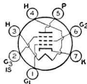
position. Heater volts (ac/dc), 18; amperes, 0.1; warm-up time (average), 18-FW6-A, 20 seconds.
