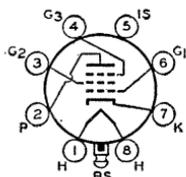
Glass lock-in type used in video amplifiers of television receivers and in other applications requiring high transconductance. Outline 15, OUTLINES SECTION. Tube requires lock-in socket. Heater volts (ac/dc), 6.3; amperes, 0.45. Characteristics and maximum ratings as class A<sub>1</sub> amplifier: plate volts, 250 (300 *max*); grid-No.2 supply volts, 300 *max*; grid-No.2 volts,
