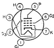
Heater volts (ac/dc), 6.3; amperes, 0.45. Maximum ratings as class A<sub>1</sub> amplifier: plate and grid-No.2 (screen-grid) supply volts, 300 *max*; grid-No.2 volts, see curve page 66; plate dissipation, 3.2 *max* watts; grid-No.2 input, 0.4 *max* watt for grid-No.2 voltages up to 150 volts, see curve page 66 for grid-No.2 voltages between 150 and 300 volts; total cathode current, 13 *max* ma; peak heater-cathode volts, 90 *max*.
