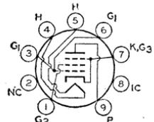
Miniature type used as vertical deflection amplifier in television receivers utilizing picture tubes having diagonal deflection angles of 110 degrees and employing series-connected heater strings. Outline 18, **OUTLINES SECTION**. Heater volts (ac/dc), 8.4; amperes, 0.6; warm-up time (average), 11 seconds. Except for heater rating, this type is identical with miniature type 6EM5.
