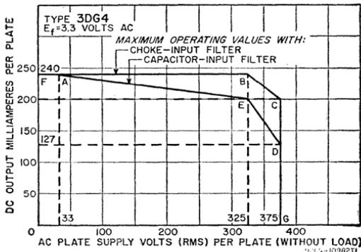
**Typical Operation with Capacitor Input to Filter:**
