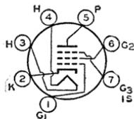
LINE SECTION. Tube requires seven-contact miniature socket and may be mounted in any position.
