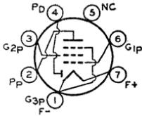
Miniature type used in battery-operated portable radio receivers as combined AM detector and af voltage amplifier. Outline 11, OUTLINES SECTION. Tube requires miniature seven-contact socket and may be mounted in any position. Filament volts (dc), 1.4; amperes, 0.05. This type is used principally for renewal purposes.
