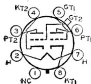
Glass octal type used as voltage amplifier or phase inverter in radio equipment. Outline 39, OUTLINES SECTION. Tube requires octal socket. Except for the heater rating of 6.3 volts (ac/dc) and 0.6 ampere and interelectrode capacitances, each triode unit is identical electrically with type 6J5. Type 6F8-G is used principally for renewal purposes.
