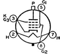
and should be operated vertically (base down or up) or horizontally with pins 2 and 7 in a vertical plane. Heater volts (ac/dc), 21.5; amperes, 0.6; warm-up time (average), 11 seconds. Except for heater ratings, this tube is identical with glass octal type 6EX6.
