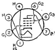
Miniature type used as combined limiter, discriminator, and audio-voltage amplifier in intercarrier television and FM receivers, Outline 13, OUTLINES SECTION. Tube requires
