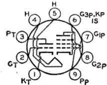
Miniature type used in color and black-and-white television receivers employing series-connected heater strings. The pentode unit is used as a video output amplifier; the triode unit is used in sync-separator, sync-clipper, and phase-inverter circuits. Outline 14, **OUTLINES SECTION**. Heater volts (ac/dc), 8; amperes, 0.6; warm-up time (average), 11 seconds. Except for heater rating, this type is identical with miniature type 6EB8.
