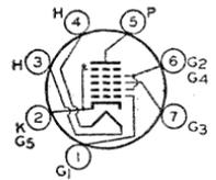
Tube requires miniature seven-contact socket and may be mounted in any position.
