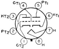
Glass octal type used as phase inverter or resistance-coupled amplifier in ac/dc radio equipment. Outline 22, OUTLINES SECTION. Heater volts (ac/dc), 12.6; amperes, 0.15. Except for heater rating, this type is identical with glass octal type 6SL7-GT.
