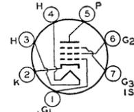
amperes, 0.6; warm-up time (average), 11 seconds. Peak heater-cathode volts when heater is negative with respect to cathode, 300 *max* (the dc component must not exceed 200 volts). Except for heater and heater-cathode ratings, this type is identical with miniature type 6BZ6.
