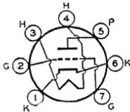
Miniature types used as rf amplifier in vhf television tuners employing series-connected heater strings. Outline 11, OUTLINES SECTION. Heater volts (ac/dc), 2BN4: 2.3, 2BN4-A: 2.35; amperes, 0.6; warm-up time (average), 11 seconds. Except for heater rating, these types are identical with miniature types 6BN4 and 6BN4-A, respectively. Types 2BN4 and 2BN4-A are used principally for renewal purposes.
