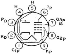
Miniature type used in automobile radio receivers; pentode unit is used as rf or if amplifier. Outline 12, OUTLINES SECTION. Tube requires miniature nine-contact socket and may be operated in any position.
