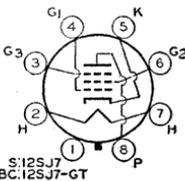
Heater volts (ac/dc), 12.6; amperes, 0.15. Except for heater rating, these types are identical with metal type 6SJ7 and glass-octal type 6SJ7-GT. Type 12SJ7-GT is a **DISCONTINUED** type listed for reference only.
