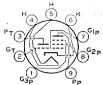
and may be mounted in any position. Heater volts (ac/dc), 18.9; amperes, 0.15. Except for heater rating, this type is identical with miniature type 6X8.
