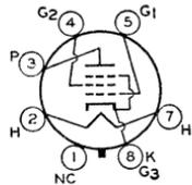
LINES SECTION. This type may be supplied with pin No.1 omitted. Tube requires octal socket and may be mounted in any position.
