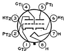
vision receivers. Outline 19, OUTLINES SECTION. Tube requires octal socket and may be operated in any position. Heater volts (ac/dc), 6.3; amperes, 1.05.
