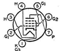
Heater volts (ac/dc), 25; amperes, 0.3. Except for heater rating, this type is identical with miniature type 50C5.
