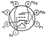
OUTLINES SECTION. Tube requires miniature seven-contact socket and may be mounted in any position. For typical operation as resistance-coupled amplifier, refer to Chart 3, RESISTANCE-COUPLED AMPLIFIER SECTION.
