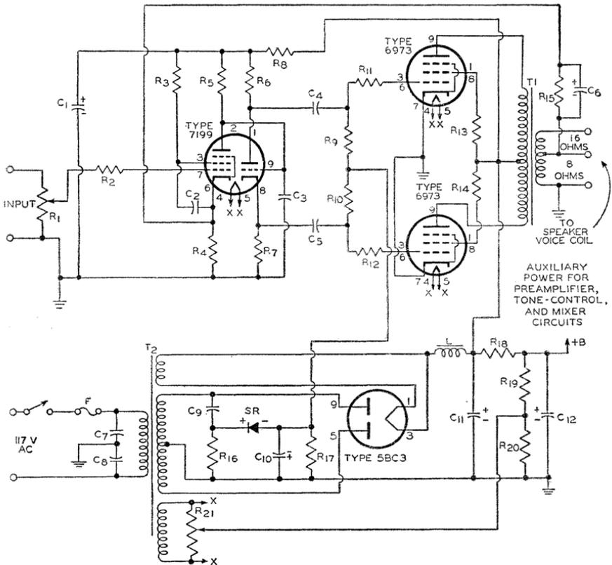
$C_1 = 40 \mu\text{f}$ , electrolytic, 450 v.
