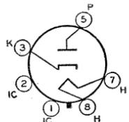
Glass octal type used as damper tube in horizontal-deflection circuits of television receivers. Outline 22, OUTLINES SECTION. Tube requires octal socket and may be mounted in any
