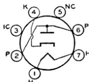
Miniature type used in power supply of small, portable, ac/dc/battery receivers where small size and low heat dissipation are important. Outline 11, OUTLINES SECTION. Tube requires miniature seven-contact socket and may be mounted in any position. Heater volts (ac/dc), 45; amperes, 0.075. Maximum ratings: peak inverse plate volts, 350 *max*; peak plate
