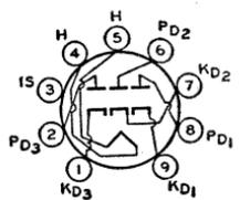
Tube requires miniature nine-contact socket and may be mounted in any position.
