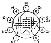
Miniature type used in the output stage of automobile radio receivers operating from a 12-volt storage battery. Outline 14, OUTLINES SECTION. Tube requires miniature nine-contact socket and may be mounted in any position.
