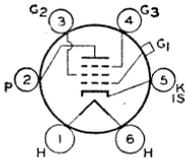
Glass type used in rf and if stages of radio receivers employing avc. Outline 45, OUTLINES SECTION. Tube requires six-contact socket. Except for interelectrode capacitances, this type is identical electrically with type 6U7-G. Refer to type 6SK7 for application information. Heater volts (ac/dc), 6.3; amperes, 0.3. This type is used principally for renewal purposes.
