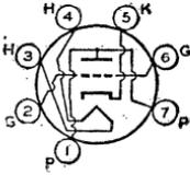
Miniature type used as oscillator in tuners of uhf television receivers. Outline 9, OUTLINES SECTION. Tube requires miniature seven-contact socket and may be mounted in any position. Heater volts (ac/dc), 6.3; amperes, 0.225. This type is used principally for renewal purposes.
