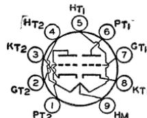
volts, -50 *max*; plate dissipation, 2.7 *max* watts; peak heater-cathode volts, 90 *max*. This type is used principally for renewal purposes.
