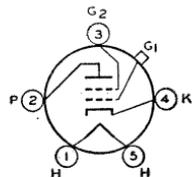
Heater volts (ac/dc), 2.5; amperes, 1.75. Typical operation and maximum ratings as class A<sub>1</sub> amplifier: plate volts, 250 (275 *max*); grid-No.2 volts, 90; grid-No.1 volts, -3; plate resistance, 0.6 megohm; transconductance, 1050  $\mu$ hos; plate ma., 4; grid-No.2 ma., 1.7 *max*. This type is used principally for renewal purposes.
