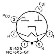
GT may be supplied with pin No.1 omitted. Both types require octal socket. Type 6X5 should be mounted in vertical position, but horizontal operation is permissible if pins 3 and 5 are in horizontal plane. Type 6X5-GT may be operated in any position. For maximum ratings, and typical operation, refer to type 6X4. Type 6X5 is a DISCONTINUED type listed for reference only.
