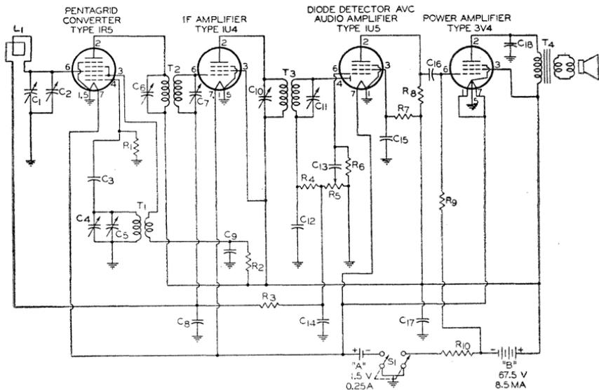
**C<sub>1</sub> C<sub>4</sub>** = Ganged tuning capacitors: C<sub>1</sub>, 10-274  $\mu\mu\text{f}$ ; C<sub>4</sub>, 7.5-122.5  $\mu\mu\text{f}$
