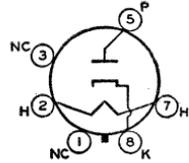
(rms), 117; minimum total effective plate-supply impedance, 30 ohms; dc output ma., 90. This is a DISCONTINUED type listed for reference only.
