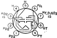
Miniature types used as combined audio amplifier, AM detector, and FM detector in AM/FM radio receivers. Diode unit No.1 is used for AM detection, and diode units No.2 and No.3
