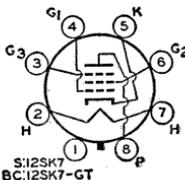
(ac/dc), 12.6; amperes, 0.15. Except for heater rating, these types are identical with metal type 6SK7 and glass octal type 6SK7-GT. Type 12SK7-GT is used principally for renewal purposes.
