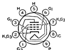
Tube requires miniature nine-contact socket and may be operated in any position. Heater volts (ac/dc), 6.3; amperes, 1.2. Except for heater rating this type is identical with miniature type 12DB5.
