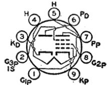
controlled heater warm-up time for use in receivers employing series-connected heater strings. Outline 14, OUTLINES SECTION. Tube requires miniature nine-contact socket and may be mounted in any position.
