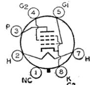
put with relatively small input voltage. Tube may be used singly or in push-pull. This type may be supplied with pin No.1 omitted. Tube requires octal socket and may be mounted in any position. Outline 22, OUTLINES SECTION. It is especially important that this tube, like other power-handling tubes, be adequately ventilated.
