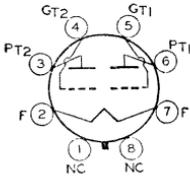
Glass octal types used in output stage of battery-operated receivers. Type 1J6-G, Outline 36; type 1J6-GT, Outline 26, OUTLINES SECTION. Tubes require octal socket. Filament volts (dc), 2.0; amperes, 0.24. Typical operation as class B power amplifier: plate volts, 135 *max*; peak plate ma. per plate, 50 *max*; grid volts, 0; zero-signal plate ma. per plate, 5; effective plate-to-plate load resistance, 10000
