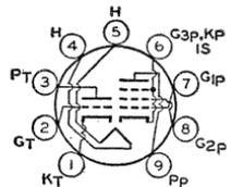
an age amplifier. The triode unit is used in sync-amplifier, sync-separator, sync-clipper, and phase-inverter circuits. Outline 14, OUTLINES SECTION. Heater volts (ac/dc), 8.4; amperes, 0.45. Except for heater rating, this type is identical with type 6AU8.
