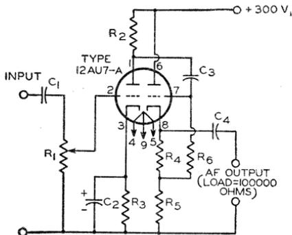
$C_1$   $C_3=0.1 \mu\text{f}$ , paper, 400 v.
