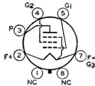
No.1 volts, 4.5; plate ma., 4.0; grid-No.2 ma., 1.1; plate resistance (approx.), 0.3 megohm; transconductance, 850  $\mu$ mhos; load resistance, 25000 ohms; power output, 115 milliwatts. Type 1A5-GT is used principally for renewal purposes.
