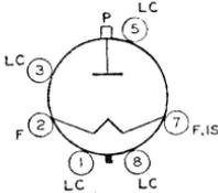
Glass octal type used as a rectifier of high-voltage pulses produced in the scanning systems of black-and-white television receivers. For curve of average plate characteristics, see page 67.
