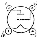
Glass type used in output stage of battery-operated receivers. Outline 34 or 35, OUTLINES SECTION. Tube requires four-contact socket. Filament volts (dc), 2.0; amperes, 0.13. Typical operation as class A<sub>1</sub> amplifier: plate volts, 180 max; grid volts, -30; plate ma., 12.3; plate resistance, 3600 ohms; amplification factor, 3.8; transconductance, 1050 μmhos; load resistance, 5700 ohms; output watts, 0.375. This is a DISCONTINUED type listed for reference only.
