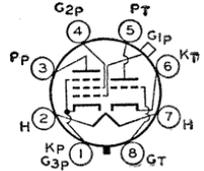
Heater volts (ac/dc), 25; amperes, 0.15. Typical operation of pentode unit as class A<sub>1</sub> amplifier: plate and grid-No.2 volts, 100; grid-No.1 volts, -3; plate ma., 7.6; grid-No.2 ma., 2; plate resistance, 185000 ohms; transconductance, 2000 μmhos. Triode unit: plate volts, 100; grid volts, -1; plate ma., 0.6; amplification factor, 112; plate resistance, 75000; transconductance, 1500 μmhos. This is a DISCONTINUED type listed for reference only.
