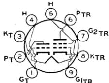
Miniature type used as combined vhf oscillator and mixer in television receivers employing series-connected heater strings. Outline 12, OUTLINES SECTION. Tube requires miniature
