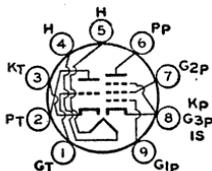
Miniature type used as a combined vhf oscillator and mixer in low B+ voltage automobile radio receivers operating directly from 12-volt storage-battery systems. Outline 12, OUT-
