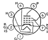
warm-up time (average), 11 seconds. Except for heater rating, this type is identical with miniature type 6CE5.
