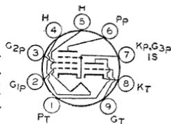
OUTLINES SECTION. Tube requires miniature nine-contact socket and may be mounted in any position.
