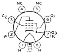
grid-No.1 volts, -7.5; peak af grid-No.1 volts, 7.5; plate resistance (approx.), 16,000 ohms; transconductance 5800  $\mu$ mhos; plate ma., zero-signal, 40 (maximum-signal, 41); grid-No.2 ma., zero-signal, 3 (maximum-signal, 7); load resistance, 2500 ohms; total harmonic distortion, 10 per cent; maximum-signal power output, 1.5 watts; peak heater-cathode volts, 90 max. This type is used principally for renewal purposes.
