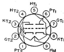
and as horizontal deflection oscillator, in television receivers. The 12AU7-A is also useful in applications critical as to microphonics. Outline 12, OUTLINES SECTION. Tubes require miniature nine-contact socket and may be mounted in any position. Each triode unit is independent of the other except for the common heater. For typical operation as a resistance-coupled amplifier, refer to RESISTANCE-COUPLED AMPLIFIER SECTION. Type 12AU7 is a DISCONTINUED type listed for reference only.
