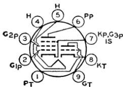
Miniature type used as combined oscillator and mixer in television receivers employing series-connected heater strings and using an intermediate frequency in the order of 40 megacycles
