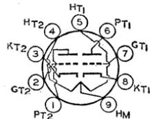
12, OUTLINES SECTION. This type is identical with miniature type 12AX7 except that it has a controlled equivalent noise and hum characteristic. For operation as resistance-coupled amplifier, RESISTANCE-COUPLED AMPLIFIER SECTION.
