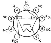
and may be mounted in any position. Heater volts (ac/dc), 12.6; amperes 0.45. It is especially important that this tube, like other power-handling tubes, be adequately ventilated. Except for heater rating, this type is identical with miniature type 6BW4.
