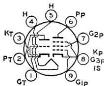
television tuners. Type 6BR8-A has a controlled heater warm-up time for use in receivers employing series-connected heater strings. Outline 12, OUTLINES SECTION. Except for basing arrangement and grid-No.1-to-plate capacitance of pentode unit, these types are identical with miniature types 6U8 and 6U8-A, respectively.
