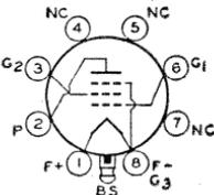
Glass lock-in type used in output stage of battery-operated receivers. Outline 15, OUTLINES SECTION. Tube requires lock-in socket. Filament volts (dc), 1.4; amperes, 0.05. For electrical characteristics and typical operation, refer to glass-octal type 1A5-GT. Type 1LA4 is a DISCONTINUED type listed for reference only.
