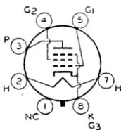
Glass octal type used in output stage of radio receivers where moderate power output is required. Outline 36, OUTLINES SECTION. Tube requires octal socket. Except for inter-electrode capacitances and a plate resistance of 175000 ohms, this type is electrically identical with type 6AK6. Heater volts (ac/dc), 6.3; amperes, 0.15. Type 6G6-G is used principally for renewal purposes.
