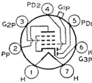
Glass type used as combined detector, avc tube, and amplifier. Outline 40, OUTLINES SECTION. Tube requires small seven-contact (0.75-inch, pin-circle diameter) socket. Except for its heater rating (2.5 volts ac/dc; 0.8 ampere) and its interelectrode capacitances, the 2B7 has electrical characteristics identical with type 6B8-G. Type 2B7 is a DISCONTINUED type listed for reference only.
