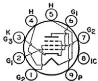
TION, except that tube is 0.6 inch shorter in vertical dimensions. Tube requires novar nine-contact socket and may be operated in any position. It is especially important that this tube, like other power-handling tubes, be adequately ventilated.
