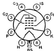
max watt; grid No.1 volts, -3; grid No.3 connected to cathode at socket; plate resistance, greater than 1 megohm; transconductance, 1575  $\mu$ mhos; plate ma., 2.2; grid-No.2 ma., 0.7. Within the limits of its maximum ratings, this type is similar in performance to metal types 6SJ7 and 12SJ7. Type 14C7 is used principally for renewal purposes.
