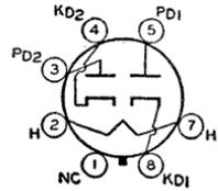
cathode volts, 350 *max*. Typical operation as half-wave rectifier with capacitor-input filter or as half-wave or full-wave voltage doubler: ac plate supply volts per plate (rms), 117; filter-input capacitor, 50  $\mu\text{f}$ ; minimum total effective plate-supply impedance per plate, 15 (30 for half-wave doubler service); dc output ma. per plate, 60. This type is used principally for renewal purposes.
