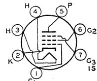
0.6; warm-up time (average), 11 seconds. Peak heater-cathode volts: heater negative with respect to cathode, 300 *max*; heater positive with respect to cathode, 200 *max* (the dc component must not exceed 100 volts). Except for heater and heater-cathode ratings, this type is identical with miniature type 6CB6.
