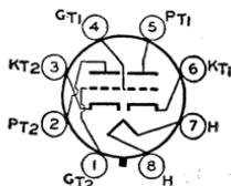
vision receivers employing picture tubes having 110-degree deflection angles and high ultr voltages. Outline 19, OUTLINES SECTION, except vertical dimensions are  $\frac{1}{8}$  inch less. Tube requires octal socket and may be mounted in any position. For curve of average plate characteristics, Unit No.1, refer to type 6DR7.
