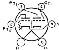
ma., 8. Output triode: plate volts, 300 *max*; plate ma., 45; plate resistance, 24000 ohms; load resistance, 7000 ohms; output watts, 4. This is a DISCONTINUED type listed for reference only.
