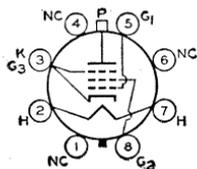
Glass octal types used as output amplifiers in horizontal deflection circuits of television equipment of the "transformerless" type where high pulse voltages occur during short duty cycles. Outlines 52 and 46, respectively, OUTLINES SECTION. Tubes require octal socket. Vertical tube mounting is preferred but horizontal operation is permissible if pins No.2 and No.7 are in vertical plane. Heater volts (ac/dc),
