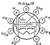
Miniature type used in a wide variety of applications in television receivers. The pentode unit is used as an if amplifier, video amplifier, age amplifier, or reactance tube. The triode
