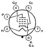
Glass octal type used as vertical deflection amplifier in television receivers employing series-connected heater strings. Outline 26, OUTLINES SECTION. Tube requires octal socket
