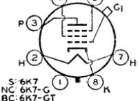
Metal type 6K7 and glass octal types 6K7-G and 6K7-GT used in rf and iaf stages of radio receivers, particularly in those employing avc. Outlines 4, 39, and 23, respectively, OUTLINES SECTION. These tubes require octal socket and may be mounted in any position. For electrode voltage supplies and application, refer to type 6SK7. Heater volts (ac/dc), 6.3;
