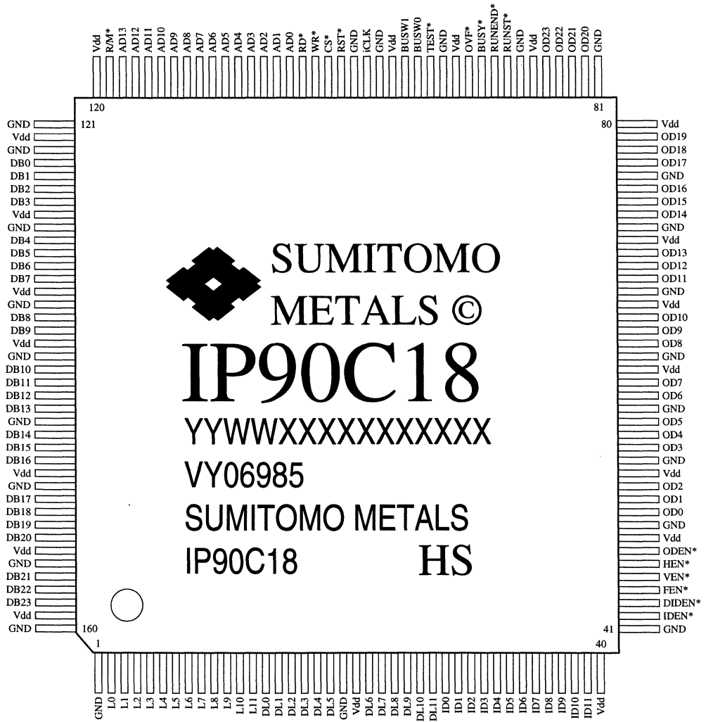
160-pin QFP package (molded area 28 mm 2 , pin pitch = 0.65 mm)
