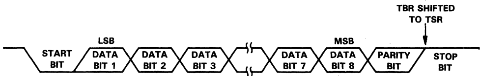
Figure 3-32. Asynchronous Transmission of Eight Bits Plus Parity
