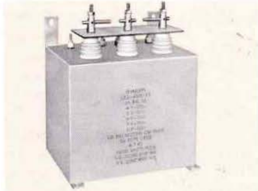
Sonar Output Transformer. 36 KW pulses, 100 millisecc @ 5% duty cycle. Input 4K \Omega CT, output 120-180 \Omega , Hipot 29 KV. Hermetic, MIL-T-27C Grade 4, 6 1/2 x 9 x 8", 37 lbs.
