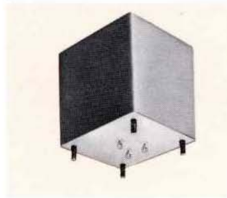
High pass filter, 30 Hz, used to eliminate from the output, 25 Hz sine wave pulses which control automatic programming on audio tracks of music tapes. Flat to 1 db from 50 Hz to 15 kHz, within 3 db to 30 Hz. Attenuation of at least 35 db from 25 Hz to 20 Hz. Source and load 600 ohms. Wt. approx. 6 lbs. MIL-F-18327C.
