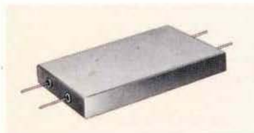
Ultra-miniature low pass filter only 1/4" high. DC to 40 kHz within ± 0.1 db, within 1 db to 60 kHz, 3 db to 70 kHz. Attenuation of at least 40 db above 81 kHz. Source and load 1K ohms. MIL-F-18327C. Wt. 1.2 ounces.
