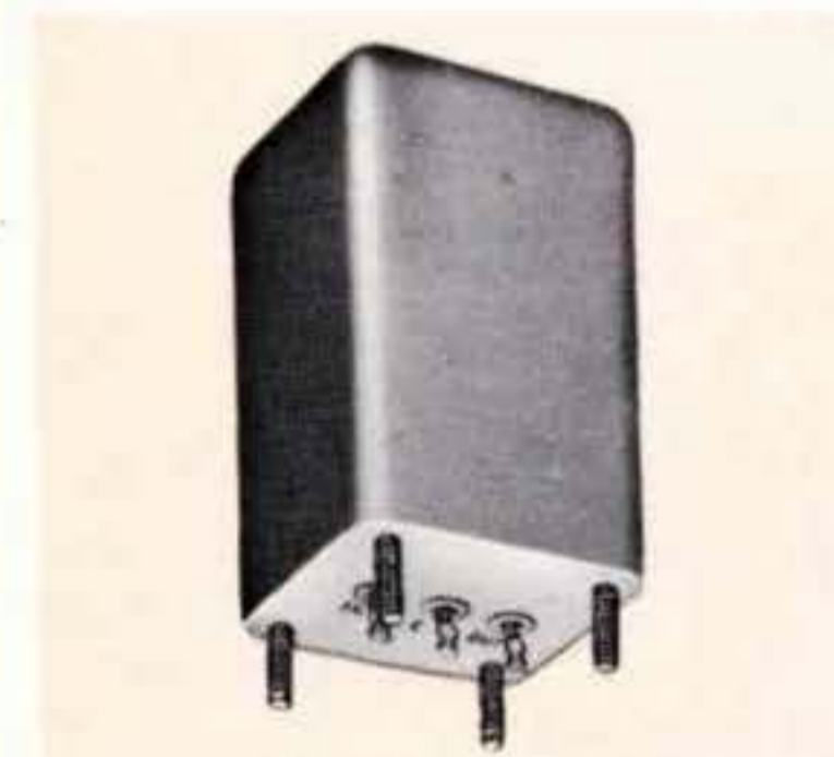
Band reject filters (two shown). The 1050 Hz filter has 50 db attenuation at center frequency and is only 3 db down at 950 and 1150 Hz. The 12.75 kHz filter has more than 100 db attenuation at center frequency and is only 3 db down at 10.8 kHz and 15 kHz. Source and load for each filter 600 ohms, both are MIL-F-18327C. Wt. 0.7 lbs.
