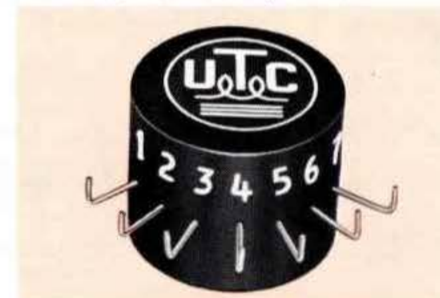
Instrument reference transformer. To operate from 15 kHz to 20 kHz with 12.5 V on one half of primary and to deliver 9.0 V on each half of secondary; secondary halves loaded with different impedances. Size: 1.1 Dia. max. x .79" high max. Weight: 34 gms.
