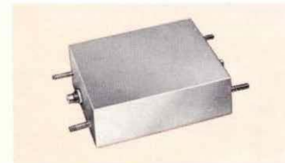
Low pass filter, 6 MHz. DC to 6 MHz within ± 0.1 db. Attenuation at least 40 db at 8.5 MHz and higher. Source and load 75 ohms. Wt. approx. 8 oz.
