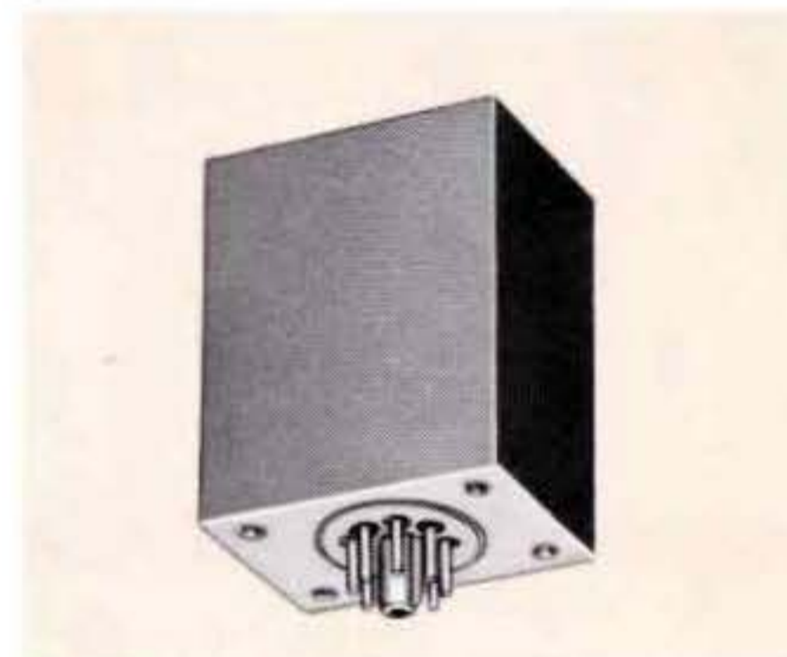
Magamp for 11 watt, 115 V., 400 Hz servomotor. Standard octal plug. MIL-T-27C; 1¾ x 2½ x 3, 1.7 lb.
