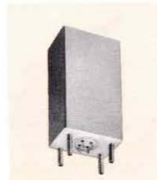
Miniaturized receiving filters, available from 425 Hz to 3315 Hz. Within 3 db at ± 42.5 Hz and attenuation of at least 36 db at ± 130 Hz. Source and load 600 ohms. Wt. approx. 3/4 lbs.
