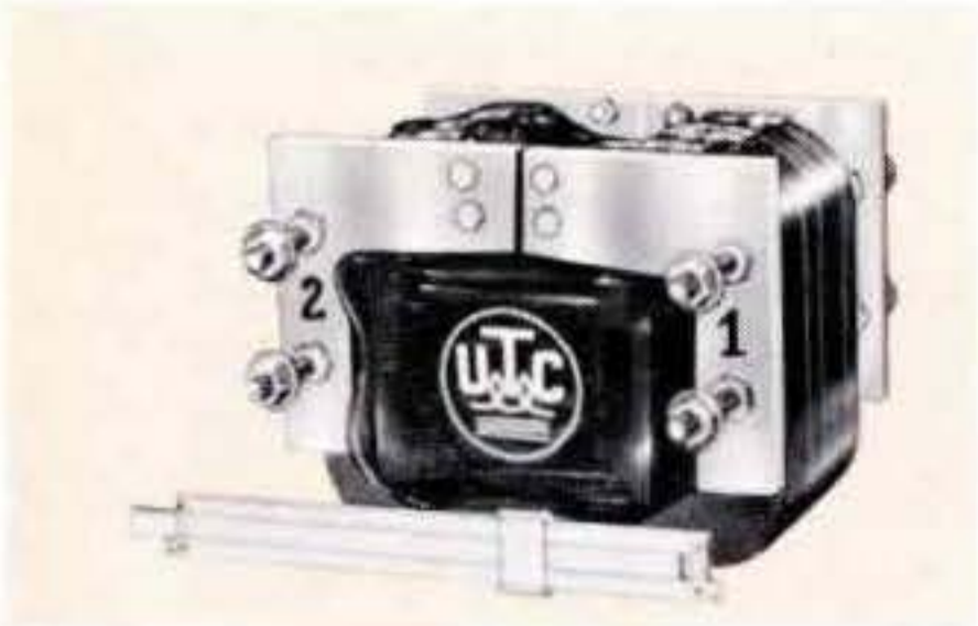
Impulse Transformer, discharge 37.5 mfd. Capacitor @ 5 KV DC, Peak Current 167,000 amps. Pulse width 2 \mu sec, Rise time .2 \mu sec, Energy level 470 watt-sec. MIL-T-27C Grade 5, Size 10 x 12 x 9 1/2", 135 lbs.
