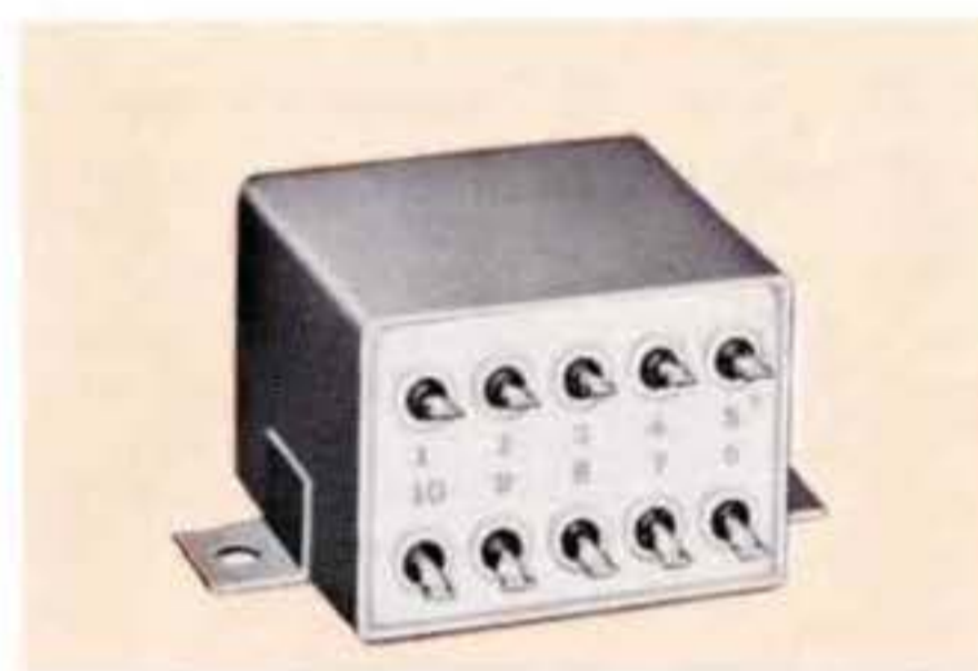
Thirty Hz cathode follower output transformer to provide equal voltages to 4 loads and supply a half-wave rectifier. Primary inductance maintained to 5% with 20% change in DC unbalance and 30% change in AC voltages.
