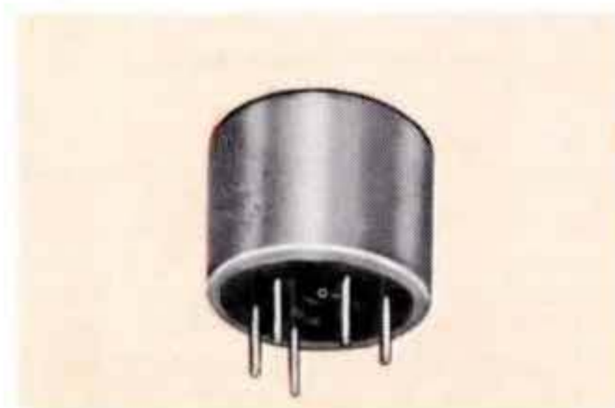
Molded carrier frequency transformer, + 8 dbm level. Within 3 db from 100 Hz to 100 kHz. 4000:4000 ohms. 3/4 Dia. x 5/8 inches, 1/3 oz.
