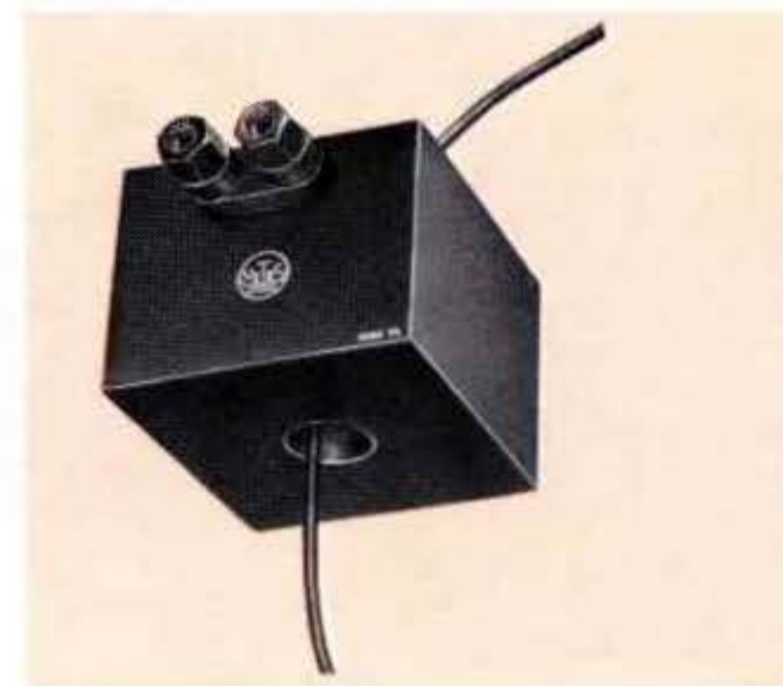
Current Transformer with 1 K load exhibits 1 V/amp/turn sensitivity. From 400 Hz to 30 kHz, ±0.1 db. Good linearity with both current, 1 mA-10 A; and turns, 1-5 T.
