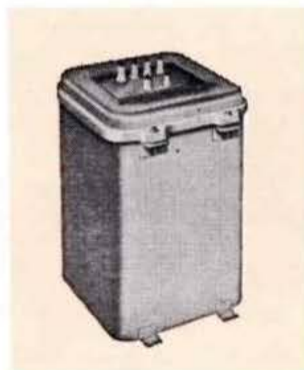
Low distortion 2.5 KW output transformer, PP 450 TH's 18,500 ohms CT to 24/6 ohms, 20 KV hipot. 520 lbs.
