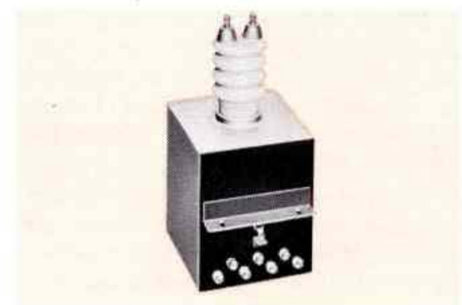
Low capacity current limiting filament transformer. Primary 118 V. 60 Hz to 6.3 V. at 3 A., 8 A. at short circuit. 25 MMFD capacity, 30 KV hipot and 200:1 capacity divider; 5 x 3¾ x 4½", 9 lbs.
