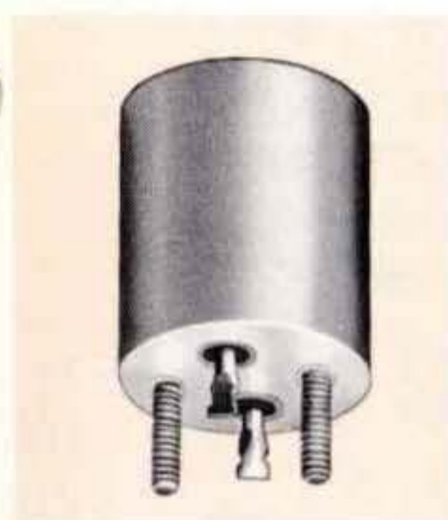
High Q, 5 millihenries inductor. High Q in the 10 kHz to 300 kHz frequency range. Grade 4, MIL-T-27C. Weight approximately 1.5 oz.
