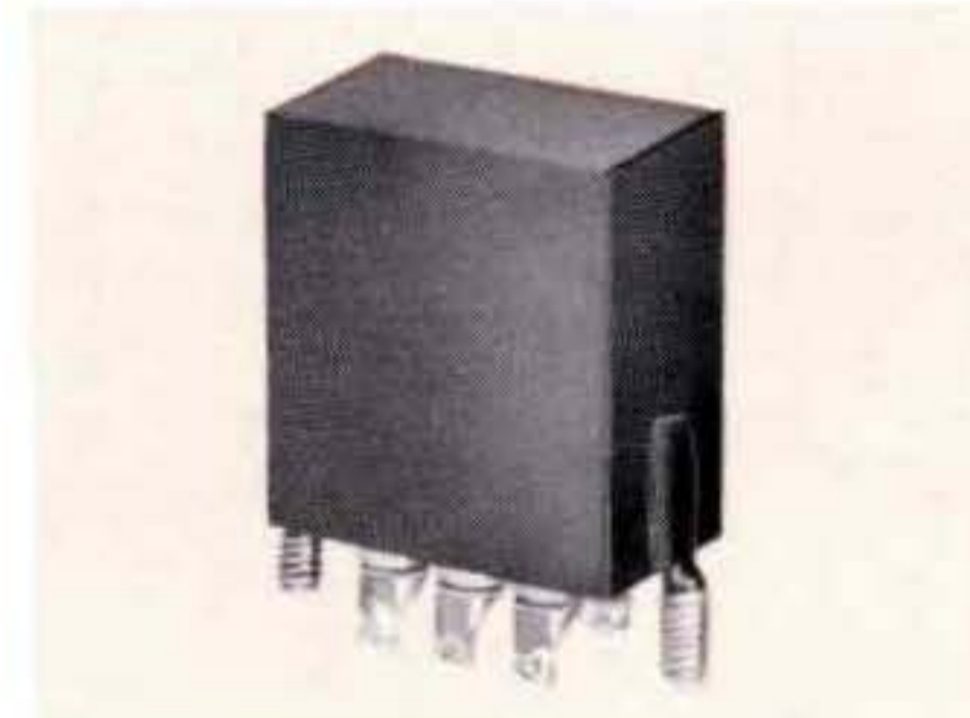
Free running blocking oscillator transformer. 600 ohms, 1:1:1, 5 \mu sec. \pm 1, 12000 \pm 10% PPS. Output 600 V. \pm 10%. Temperature stable -62° C. to 85° C. MIL-T-27C; 3/4 x 1 1/4 x 1 1/8; 1 1/2 oz.
