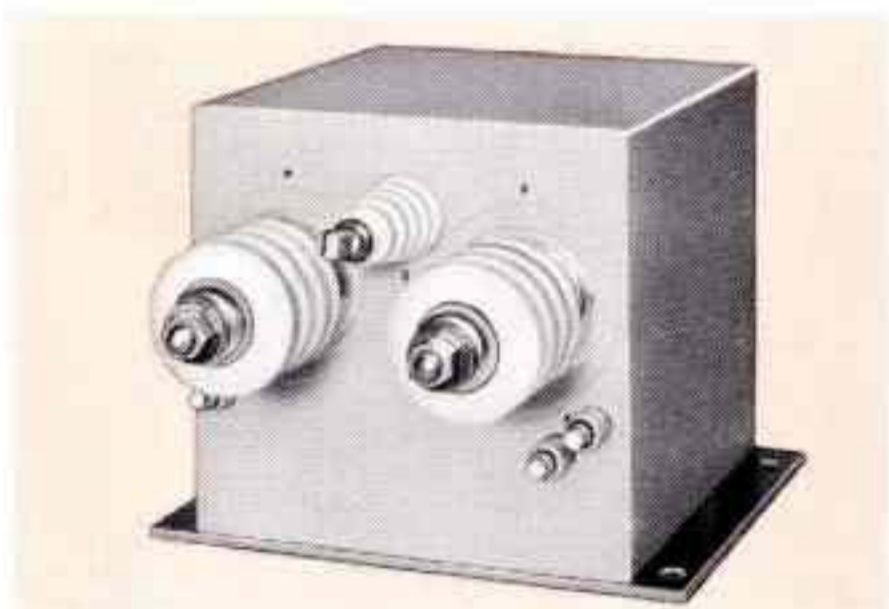
High Current and High Voltage Transformer. Input 115 V 400 Hz to 7.5 V CT-51A, 22 KV hipot. MIL-T-27C, Grade 4; 6½ x 6¾ x 6¾", 30 lbs.
