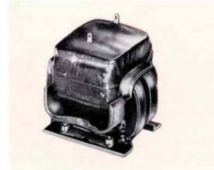
Linear charging reactor for line type pulser. 20 Hys., .11A. DC, 5 KV, 1000 PPS, 11 KV hipot. MIL-T-27C, 200° C.; 3 1/4 x 4 x 3 3/4, 3 lb.
