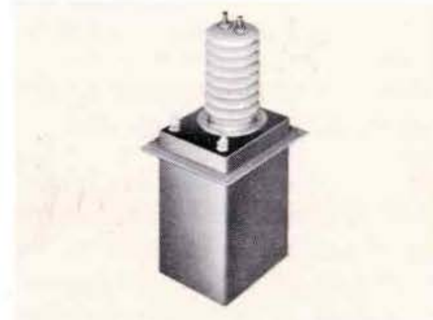
Output to Klystron. 3.5 \mu sec. pulses in group of pulse trains at high rep. rate. 1% droop over pulse train. 43 KV Hipot. MIL-T-27C; NA case; 4 1/4 x 5 x 6 3/4, 11 1/2 lb.
