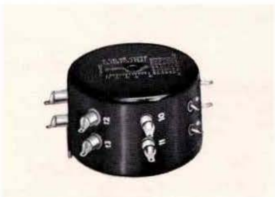
Toroidal Transistor inverter transformer. Input 24 V DC, outputs 4 windings 150 V to 1050 V DC. Hipot 3800 V. Hermetically sealed, MIL-T-27C, 2½ dia. x 1½", 15 oz.
