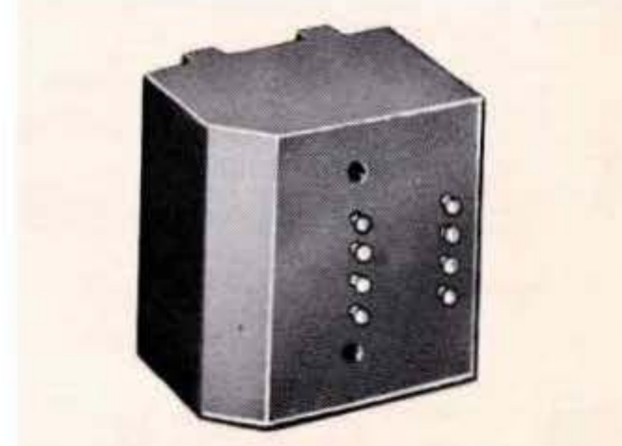
Dual saturable reactor. Input 10 V. - 1 kHz. Output 3.5 V. 2 MA DC control current. 130° C. MIL-T-27C; 1¾ x 1¾ x 1¼, 5 oz.
