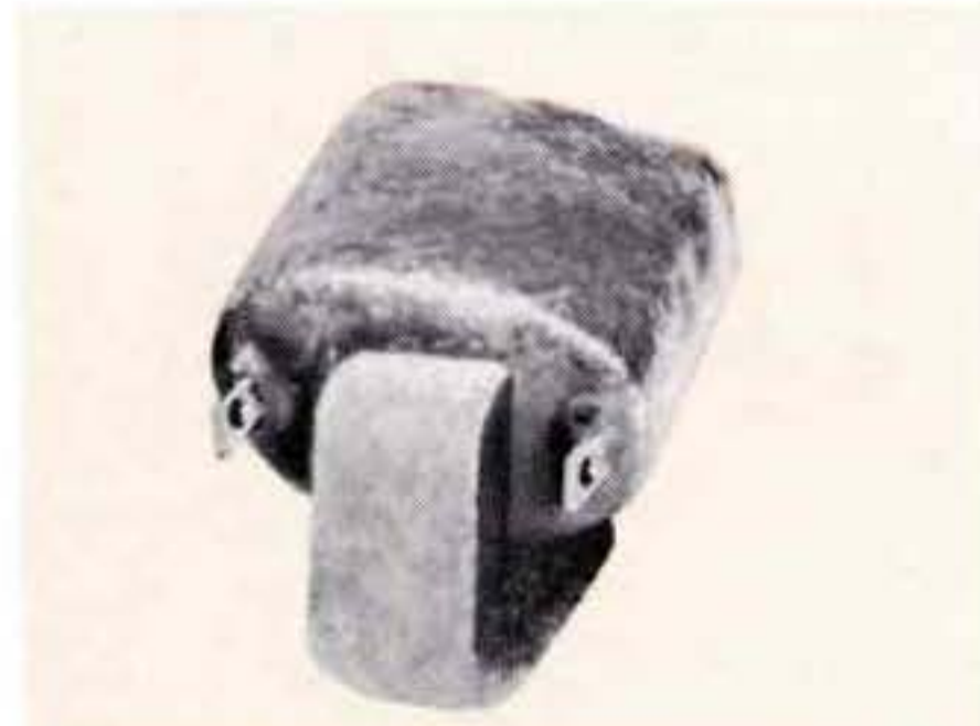
Pulse current transformer, Thyatron cathode to 50 ohms. Input 100A. Output 200 V. to 50 ohms. .5/2.4 \mu sec. 2000 PPS. MIL-T-27C; 1 3/4 x 1 1/4 x 1 1/4, 2 oz.
