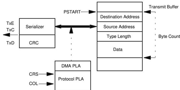
**Figure 5. Packet Transmission**
