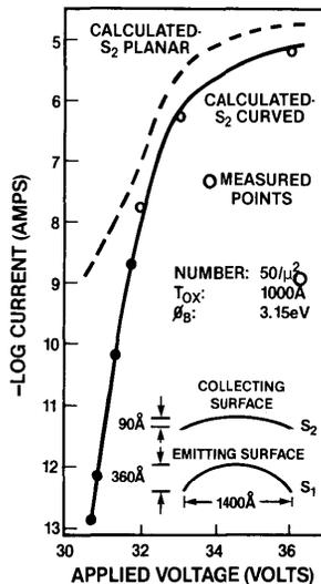
Figure 14: Reverse tunneling characteristic comparing the measured data with curves calculated for a concave and planar emitting surface.
