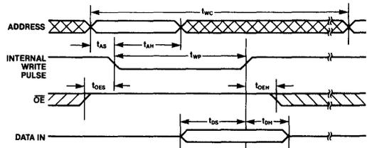
Figure 5) Timing diagram for the Xicor EEPROM byte write cycle.
