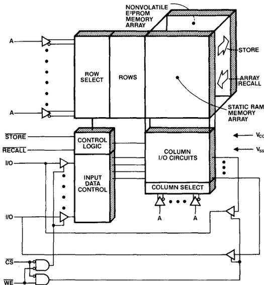
Figure 1) NOVRAM memory block diagram.
