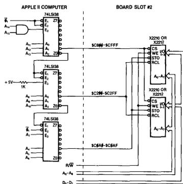
Figure 8) Connections for operating the NOVDRAM on the I/O Bus of an APPLE II computer.
