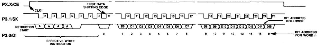
Figure 4. Write Cycle Sequence
