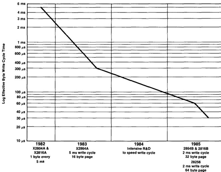
**Figure 1: Xicor's E<sup>2</sup>PROM Write Cycle Time Reduction.**
