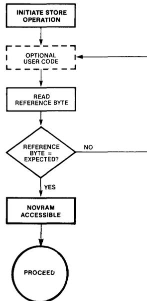
Figure 2: Early Write Completion Flowchart
