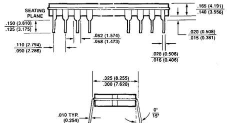
Figure 3a: Package outline drawing for memories in cerdip
