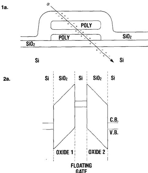
Figure 1: Cross section and potential diagram of a typical floating gate memory transistor; a) the cross section is cut through in the direction of current flow; b) the potential diagram is shown for the case that the floating gate is programmed and the access gate grounded.
