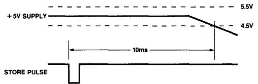
Figure 4: Initiate Store to Power-down Condition Timing
