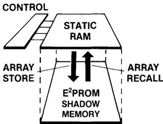
Figure 1: Xicor NOVRAM SRAM Functionality with Nonvolatile E<sup>2</sup>PROM
