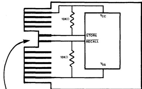
Figure 5: Typical Cartridge Write Protect Scheme
