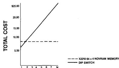
Figure 4) Relative costs of using NOVRAM memories as opposed to DIP switches as a function of packages of 8 switches required.
