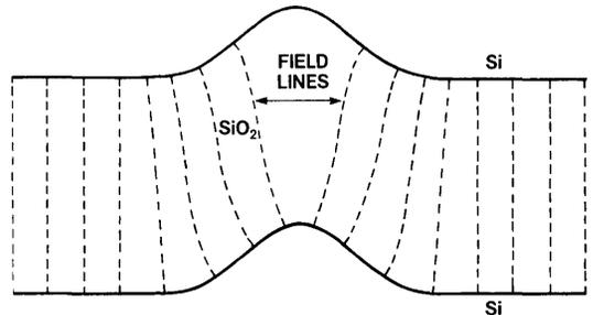
Figure 12: Sketch illustrating the manner in which field lines converge near convex feature and diverge near concave features.
