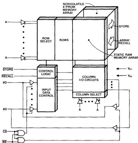
Figure 1) Block diagram of the XICOR NOVRAM family.
