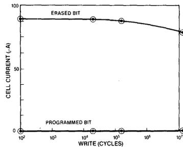
Figure 4. Endurance of a "Typical" E<sup>2</sup>PROM.
