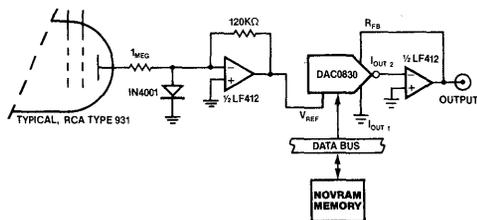
Figure 15) Gain trimming for photomultiplier tubes.
