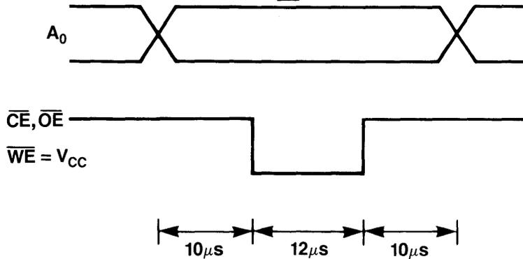
Figure 10: Static life test bias diagram
