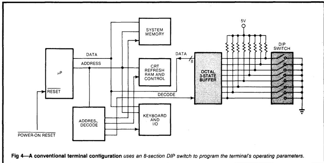
Fig 4—A conventional terminal configuration uses an 8-section DIP switch to program the terminal's operating parameters.
