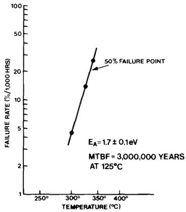
Figure 8:  $E^2$  cell endurance data for a typical cell
