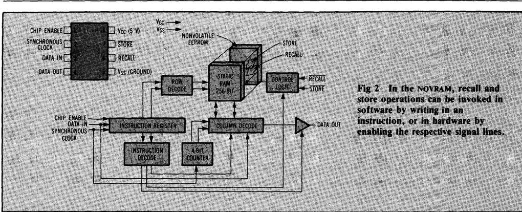
**Fig 2** In the NOVDRAM, recall and store operations can be invoked in software by writing in an instruction, or in hardware by enabling the respective signal lines.
