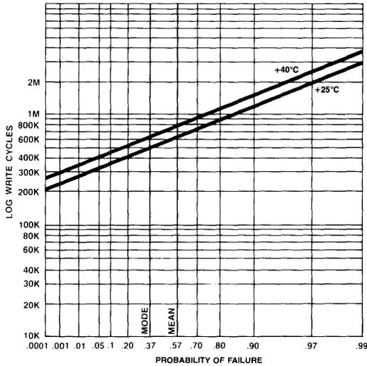
Figure 2: Affect of Ambient Temperature on Endurance
