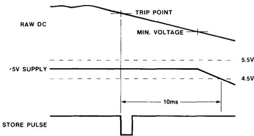
Figure 3) Falling dc is detected to trigger a STORE pulse at least 10ms before the +5 Volt supply drops below 4.5 Volts.
