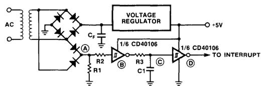
Figure 12) Two CMOS Schmitt Triggers are used to detect the absence of ac.
