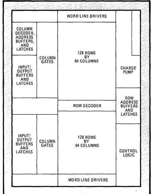
**1. All aboard.** This 16-K electrically erasable programmable read-only memory integrates all its support circuits. A charge pump generates the programming voltage from a 5-V supply; latches hold addresses and data during the internally timed write cycle.
