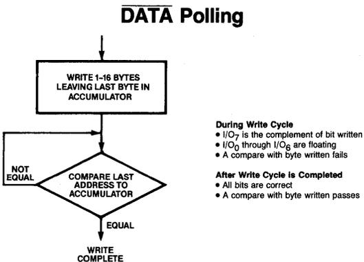
Figure 1: Testing for Nonvolatile Write Cycle Completion
