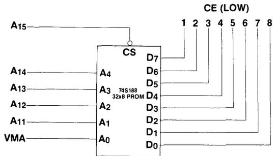
Figure 5. Bipolar PROM Mapping
