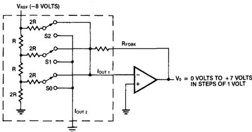
Figure 7) A simplified 3-switch CMOS DAC.
