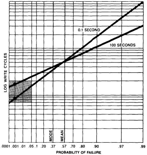
Figure 3: Affect of Write Cycle Frequency on Endurance
