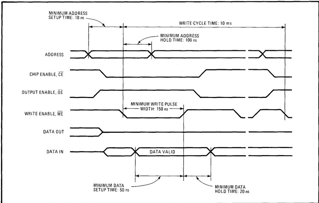
**2. Like a static RAM.** The write-cycle timing for the X2816A EE-PROM looks much like that for a static random-access memory. Although the write cycle takes a maximum of 10 ms, latches hold the address and data signals, freeing the processor for other tasks.
