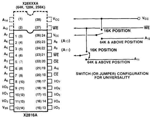
Figure 1. Universal Socket for 16K Thru 256K E<sup>2</sup>PROMs
