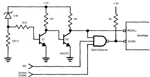
Figure 10) The Zener power supply detector is used in combination with the open collector on the **STORE** pin to provide protection against an inadvertent STORE operation during power up and power down.
