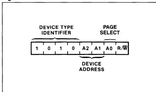
The next two significant bits address a particular device. A system could have up to four X2404 devices on the bus (see Figure 10). The four addresses are defined by the state of the A<sub>1</sub> and A<sub>2</sub> inputs.
