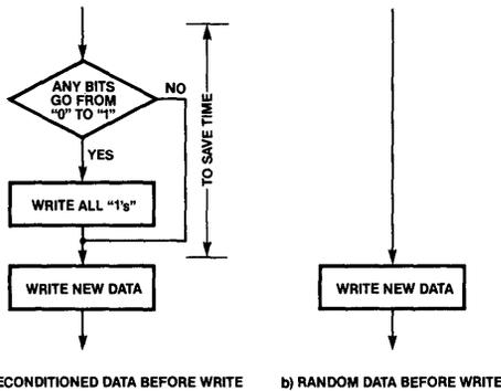
Figure 9) Comparison of software requirements for minimum write time systems between a) preconditioned data and b) random data prior to the write cycle.
