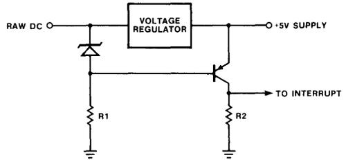
Figure 15) A dropping unregulated dc turns on the PNP transistor.
