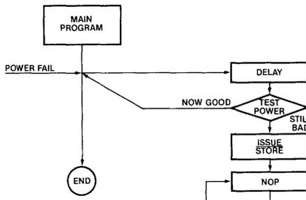
Figure 17) The program branches to a STORE subroutine when a power failure is detected.
