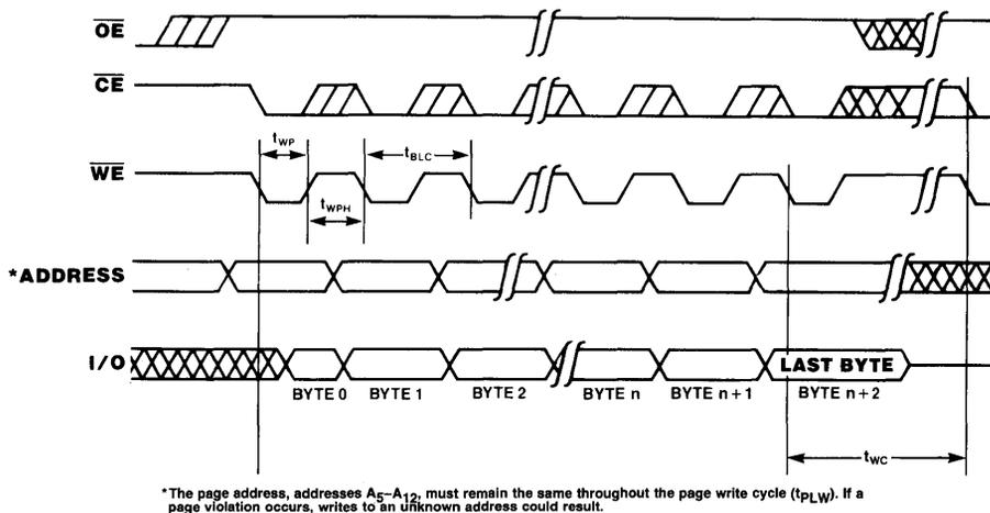
Figure 5: X2864B Page Write Timing Diagram
