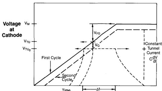
Figure 4: Voltage vs. Time Relationships at Floating Gate
