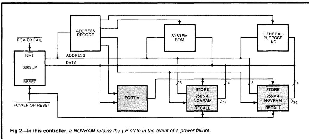
**Fig 2—In this controller, a NOVRAM retains the μP state in the event of a power failure.**
