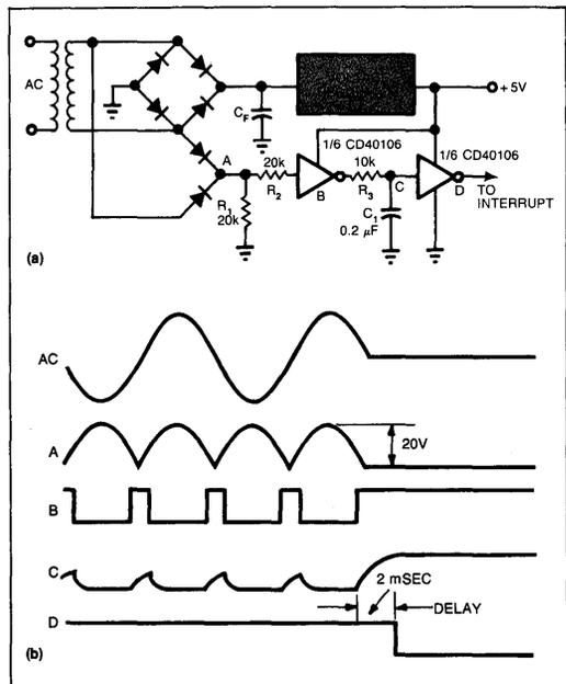
Fig 6—When you use two Schmitt triggers to detect ac loss (a), the delay produced by  $R_3$  and  $C_1$  must be longer than the first gate's output pulse width. The timing diagram (b) shows the circuit waveforms.
