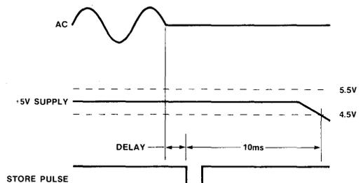
Figure 2) Missing ac must trigger a STORE pulse at least 10ms prior to the regulated dc dropping below specification.
