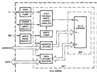
Figure 2. X2816A Block Diagram.
