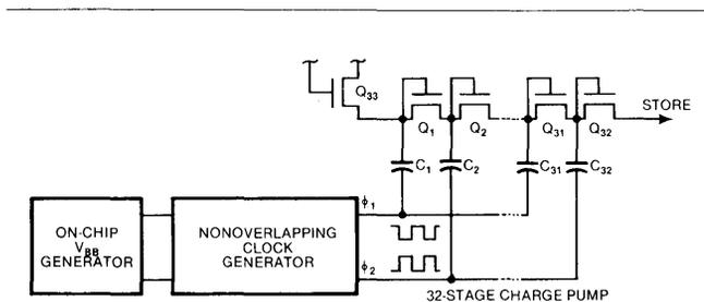
**Fig B—A 32-stage charge pump internally generates a NOVRAM's high Store voltage, allowing the device's NOVRAM and EEPROM sections to operate from 5V.**
