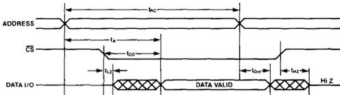
Figure 5) Timing diagram for Reading from the RAM.
