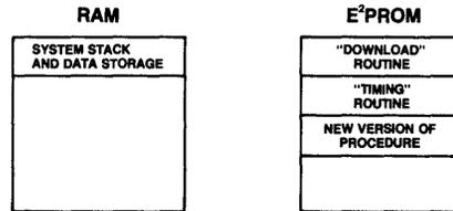
Figure 5c: Memory Map RAM Erased After Transfer Complete
