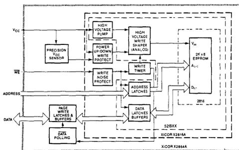
Figure 3. X2864A Block Diagram.
