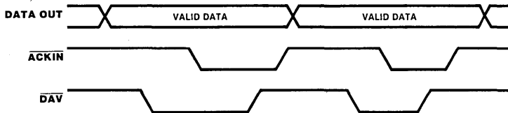
Figure 5. Two-Wire Interlocked Handshake Timing (output)
