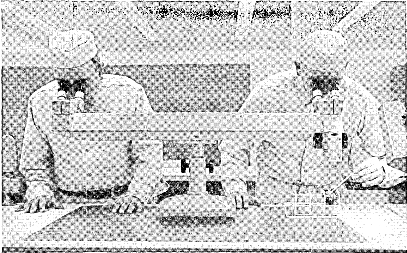
Fig. 3—Dual microscope used to instruct a Laboratory Technician as to the quality of a soldered connection.
