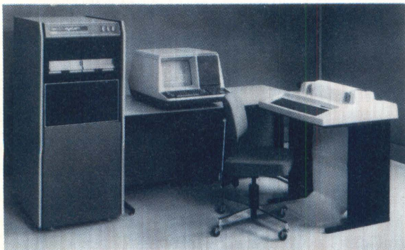
DEC Datasystem 352, lowest configuration of the disc-based 350 series business time-sharing systems, consists of PDP-11/10 central processor unit with 32 thousand characters of core, two floppy discs with 500 thousand characters, CRT terminal with keyboard, and 30-char/s printer
