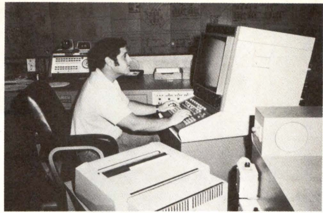
Fig 3 Master control center of Central Power and Light Co SEMS installation in Corpus Christi, Texas. Status of transmission and distribution functions is displayed on CRT in 7-color display, in either tabular or schematic format. Command to alter status of any control point is entered through keyboard
