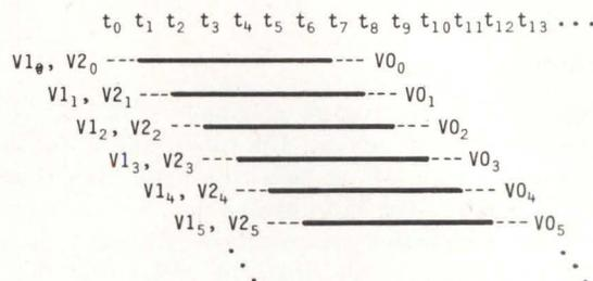
Fig 3 Vector instruction timing example ( $V0 \leftarrow V1 + V2$ ). New pair of operands is sent to functional unit each clock period. After first result emerges from functional unit, new result is sent to result register each clock period
