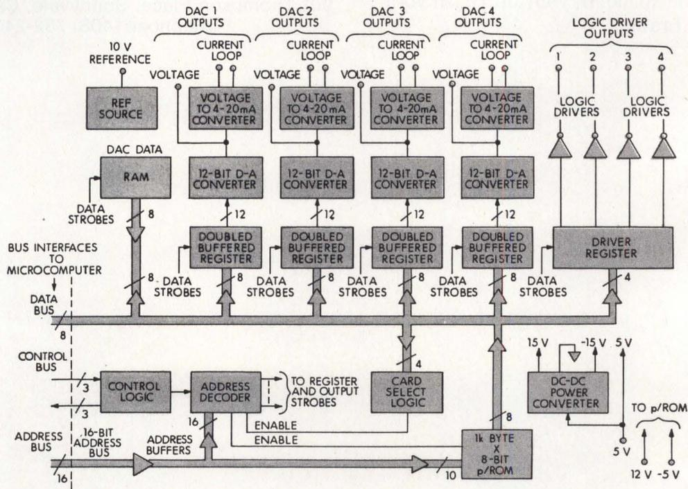
Analog Devices' RTI-1201 Intel SBC 80 compatible output subsystem contains four digital and four analog channels. Components are contained on single board to reduce hardware and software efforts required to interface microcomputers
