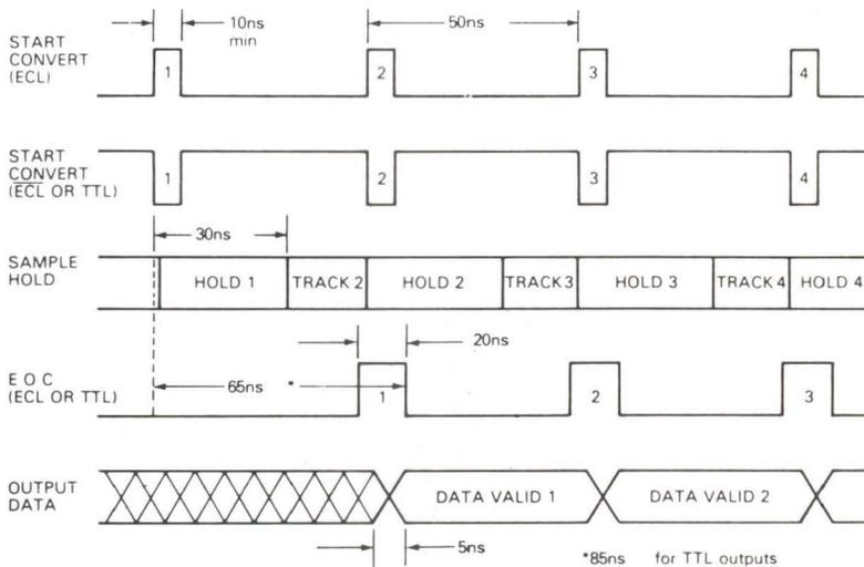
Timing diagram of ADC-TV8B. 50-ns max time between conversions provides 20-MHz conversion rate. Conversion delay (time from start convert pulse to time data are valid) is 6.5 ns for ECL version and 85 ns for TTL
