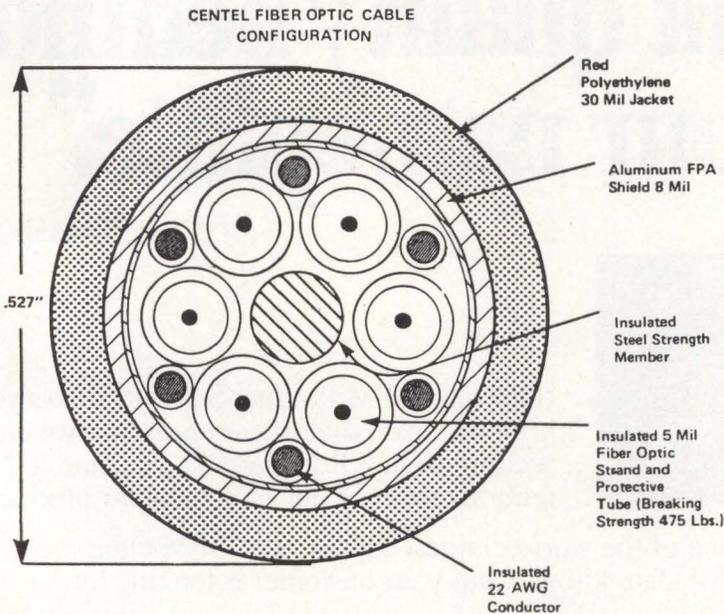
Optical cable cutaway shows center insulated with 0.09" (2.3-mm) steel strength member (also used to pull cable through duct) fitted with polyethylene jacket. Surrounding steel are six fibers, each covered with polypropylene tubing and then by flame-resistant strength member. Copper wires surround six subcables; wires are covered by mylar tape for thermal barrier. Aluminum sheeting serves as strength member and moisture/rodent barrier. Covering is water-resistant red polyethylene shield
