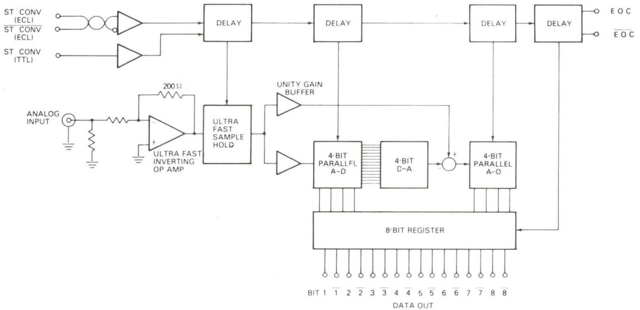
Block diagram of Datal Systems' 8-bit, 20-MHz video ADC. Analog input comes from terminated rf connector to ultrafast inverting op amp which scales input to desired level for sample hold and ADC
