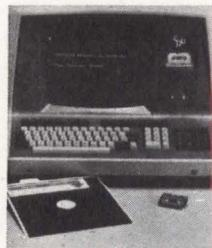
Operating within the text management system, the Ph.D. offers 16-bit processing power and architectural compatibility with large minis. System is based on the DEC PDP-11/03 processor with 4k 16-bit words of random access storage, serial I/O interface, and CRT for use as standalone system and component in distributed network. Std software includes PDP-11 operating systems and languages.
