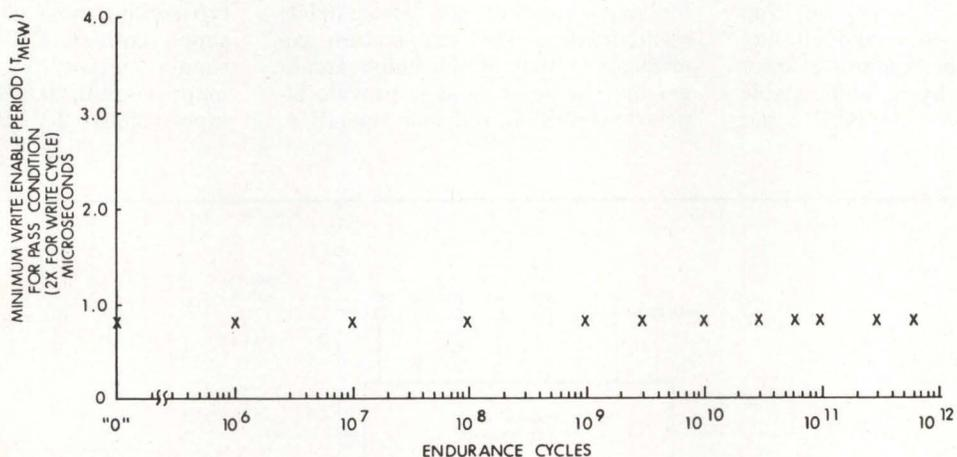
Fig 2. Endurance data for minimum write enable period. Endurance stress was for 2.2- $\mu\text{s}$  write cycle at 30 V with alternating bit pattern on word 15. Test period was 23 days
