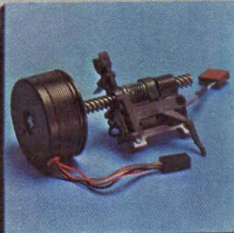
**Fast access of 30 ms track to track** is made possible by a low inertia, low friction, four-start lead screw positioning system, a field proven, high accuracy positioner technology.
