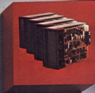
**Four-drive daisy chain capability** with unit select provides up to 2 Mbytes data capacity in a convenient system configuration. Overlap seek speeds system access.
