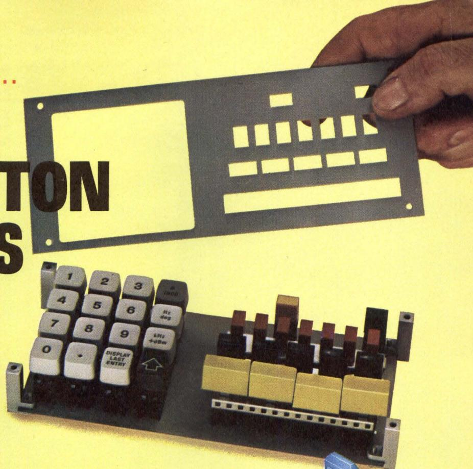
To meet the special digital and analog needs of today's  $\mu$ P-based controls, Centralab offers design engineers a whole new system of modular pushbutton switch building blocks. We call it MPS—integrated Modular Panel System. MPS saves PC board and panel area and simplifies front panel design, cuts assembly costs, reduces back-panel space requirements, and meets the digital-analog needs of  $\mu$ P-based controls. Check these space saving, cost-cutting features.
