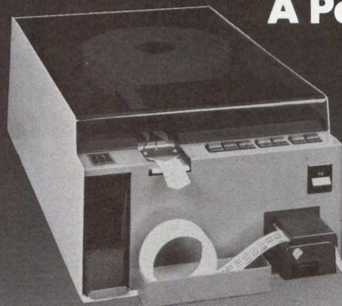
DATA SPECIALTIES' SRP-300 connects, without modification, to any 300 baud teleprinter or CRT terminal thru the RS-232 connector and provides all the features of a conventional ASR. In addition, the Combo may be used as a stand-alone computer peripheral. This whisper quiet (58 dB) unit is provided with full/half duplex, line/local, search/edit control, backspace, tape feed, remote control selection and switch selectable baud rates as standard features.
