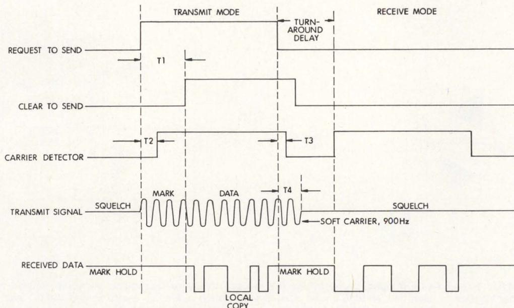
Fig 6 Basic timing diagram. Key interface signals and their interrelationships are shown for single remote modem in 4-wire multidrop network
