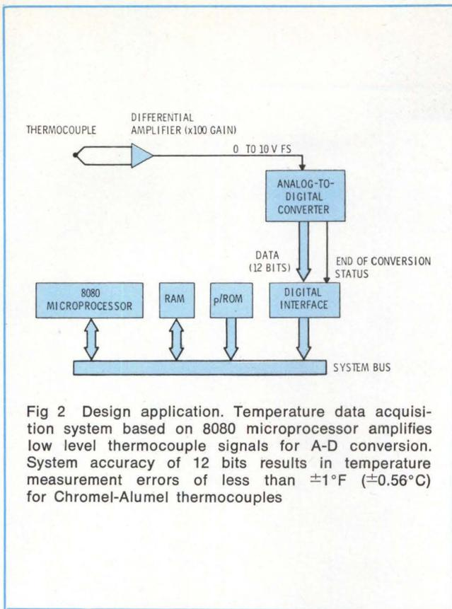
Fig 2 Design application. Temperature data acquisition system based on 8080 microprocessor amplifies low level thermocouple signals for A-D conversion. System accuracy of 12 bits results in temperature measurement errors of less than  $\pm 1^\circ\text{F}$  ( $\pm 0.56^\circ\text{C}$ ) for Chromel-Alumel thermocouples
