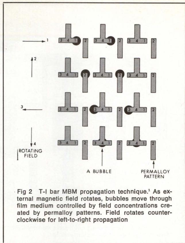
Fig 2 T-I bar MBM propagation technique.<sup>1</sup> As external magnetic field rotates, bubbles move through film medium controlled by field concentrations created by permalloy patterns. Field rotates counter-clockwise for left-to-right propagation
