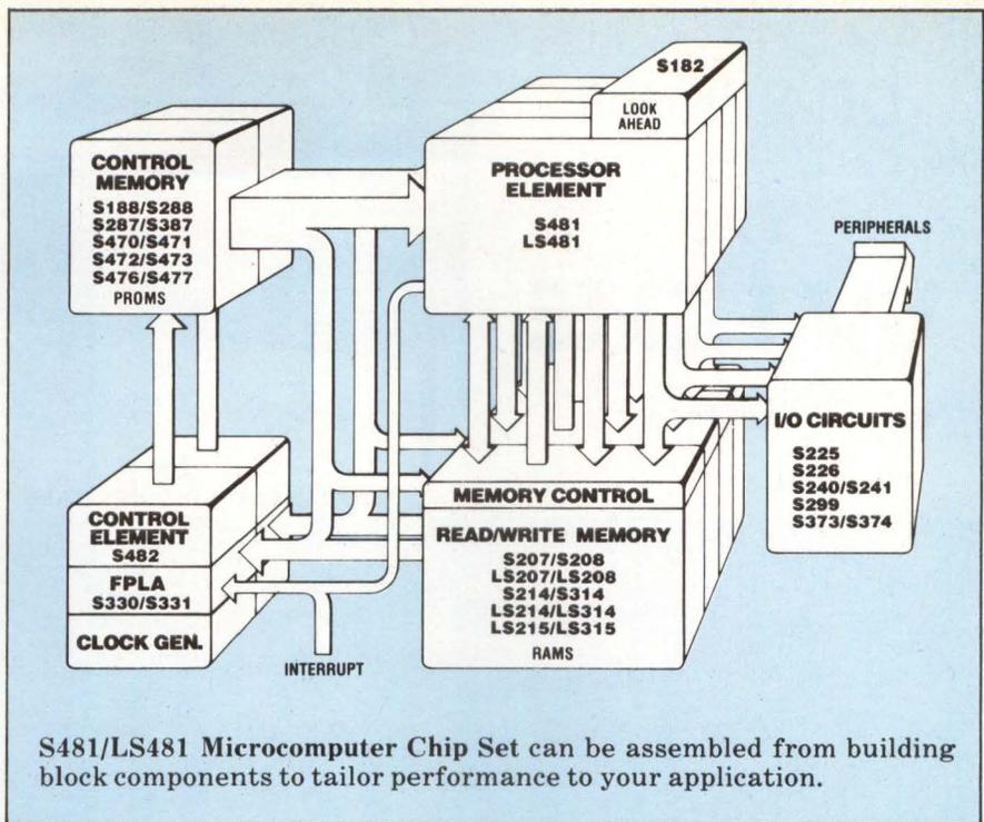
S481/LS481 Microcomputer Chip Set can be assembled from building block components to tailor performance to your application.
