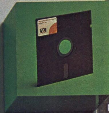
**Data capacity to 498.8 Kbytes** on one 5¼ inch diskette is achieved by exclusive 40 track recording, plus double density, plus dual sided recording. Dual index and file protect sensors permit recording on both sides of media.
