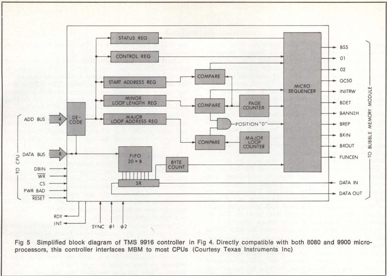
Fig 5 Simplified block diagram of TMS 9916 controller in Fig 4. Directly compatible with both 8080 and 9900 microprocessors, this controller interfaces MBM to most CPUs (Courtesy Texas Instruments Inc)
