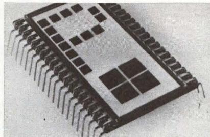
As a readout for alphanumeric applications, LCD includes a 5 x 7 dot matrix plus 4 annunciators and is used as part of point-of-sale or online terminals. Matrix viewing area is 0.9 x 0.6" (2.3 x 1.5 cm). DIP is directly solderable into PC boards. Characteristics are 3.0 V operation and reflective background. **Perkins, Inc.**, 127 E Alton Ave, Santa Ana, CA 92707.
