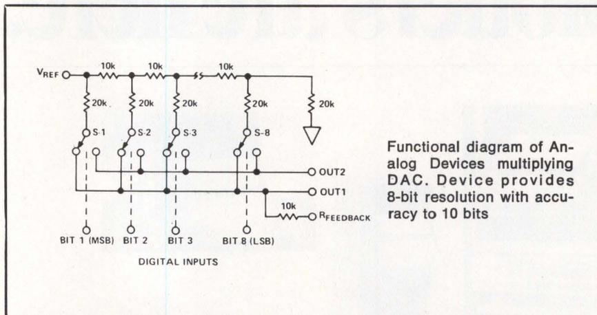
jections (gain) of 0.02%/° and 0.03%/°. Monotonicity is guaranteed over the full 0 to 70°C range. For all temperatures, power requirements are 5 V min, 16 V max, and 100  $\mu$ A max.
