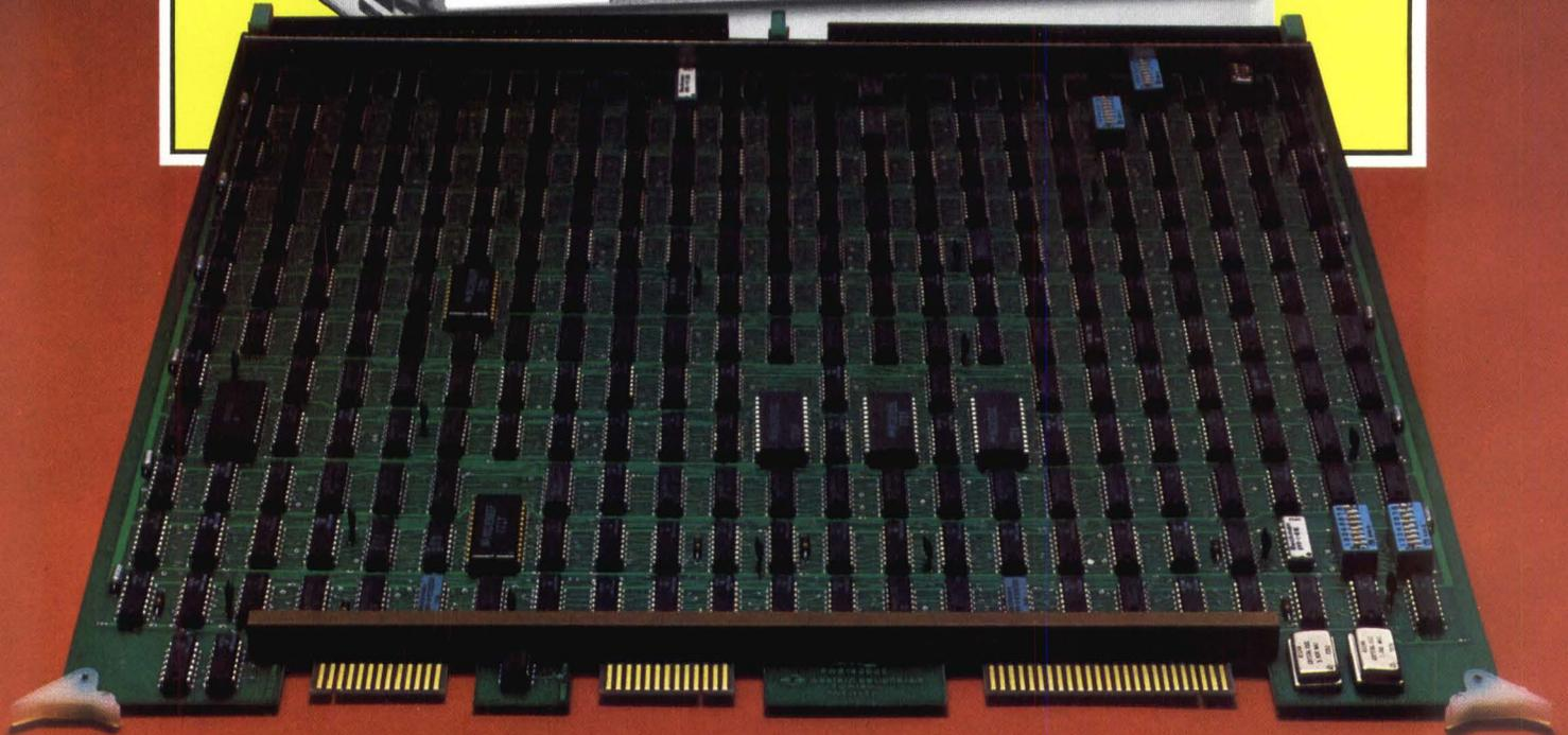
Single board, fully embedded, dual density tape system for PE and NRZ formats. Total Operating System compatibility. Allows up to 4 drives with any mix of NRZ 7 Track, NRZ 9 Track, PE and PE/NRZ to be operated from a single controller. That isn't all! You may select any two speeds in the range of 12.5 to 125 ips. Enhanced Command Set and Extended Status Register are standard in all TC-140's for those requiring a level of performance never before available.
