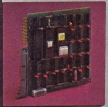
**Wangco's 5½" square, LSI based intelligent Micro-controller** mounts on the Micro-Floppy Disk Drive providing a soft-sectored, IBM type format for up to four drives. Based on the Intel MCS 8048 micro-processor, the controller has a nine macro-command structure including diagnostic and automatic diskette copy. Most overhead requirements are greatly reduced.
