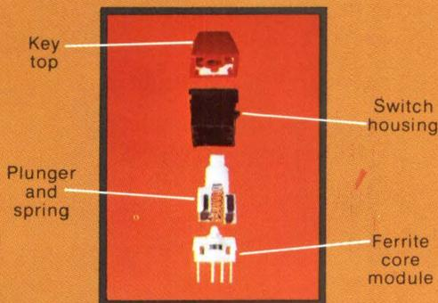
**Unique contactless key switch makes the difference.** Utilizing ferrite core switching technology, the CORTRON Key Switch is mechanically simple (only 4 basic parts!) and has an ultra reliable 100 million cycle life test rating. CORTRON Keyboard Professionals can translate what this can mean to you in cost efficiency terms of MTBF (mean time before
