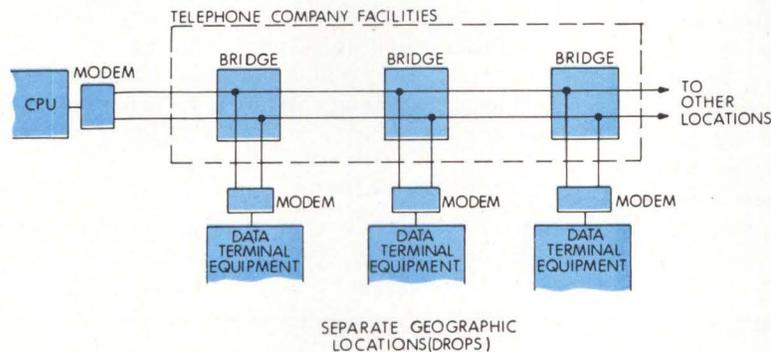
Fig 4 Leased-line multidrop network. Leased-line multidrop network is ideal for large-scale systems where CPU communicates with many modems scattered throughout large geographical area. Data terminal equipment is coupled to main line through modems and bridges
