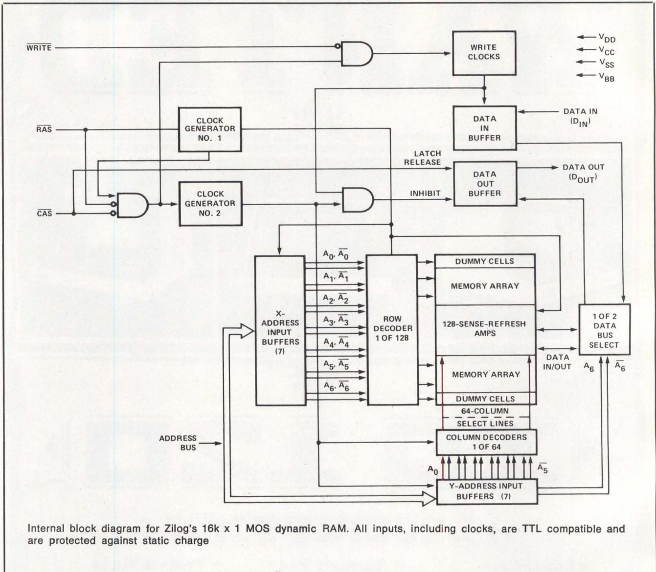
CAS and WRITE have made their negative transitions. Whichever of these signals makes its negative transition later generates the strobe for the data-in register.
