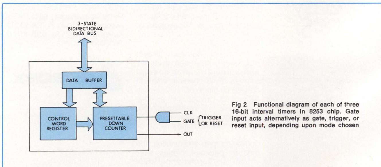
**Fig 2** Functional diagram of each of three 16-bit interval timers in 8253 chip. Gate input acts alternatively as gate, trigger, or reset input, depending upon mode chosen
