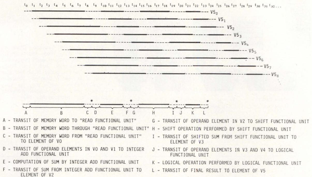
Fig 5 Timing diagram for chaining. Each horizontal line shows production of one element of V5 vector result. Time spent in passing through each functional unit used in instruction sequence is indicated by bar of corresponding length. Chain slot times for each functional unit are indicated by asterisks
