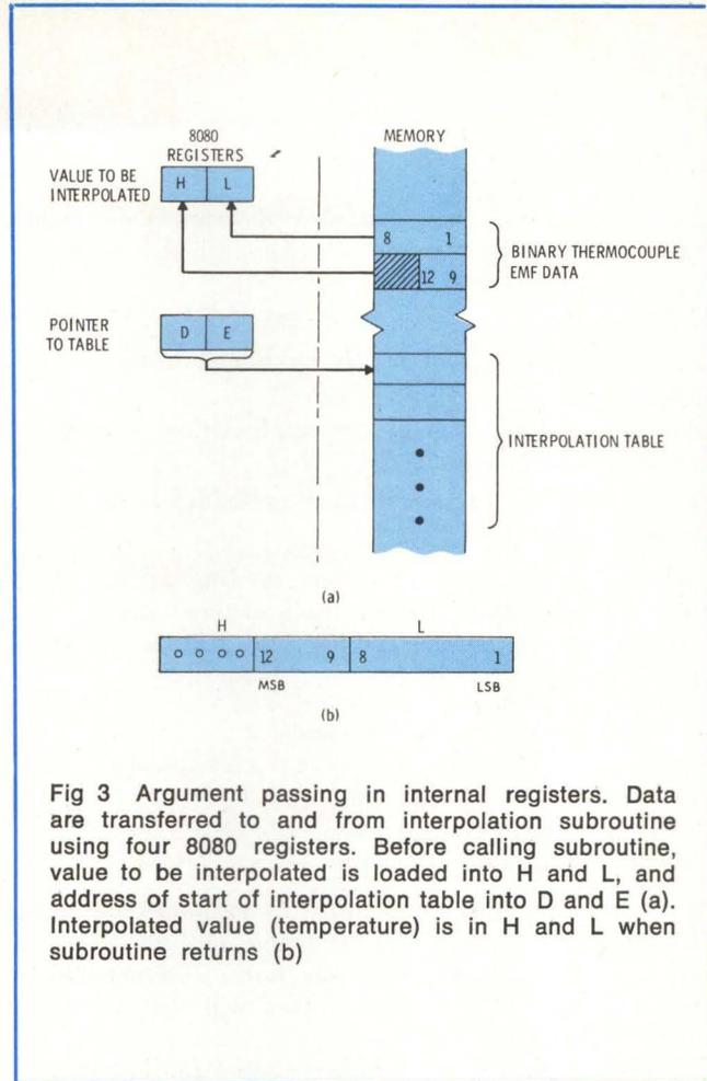
**Fig 3** Argument passing in internal registers. Data are transferred to and from interpolation subroutine using four 8080 registers. Before calling subroutine, value to be interpolated is loaded into H and L, and address of start of interpolation table into D and E (a). Interpolated value (temperature) is in H and L when subroutine returns (b)
