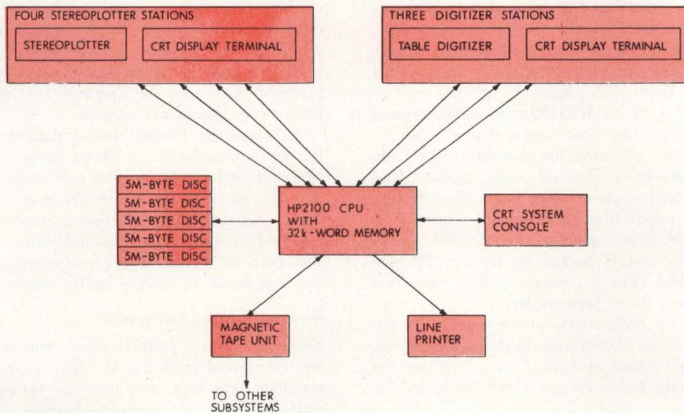
Fig 2 Detailed block diagram of input subsystem. Mapping features on aerial photographs are entered through stereoplotters. Table digitizers enter data from existing maps. Station CRTs can provide instructions to operators or can question validity of any data that control computer does not accept. Data base is maintained on 25M bytes of disc memory
