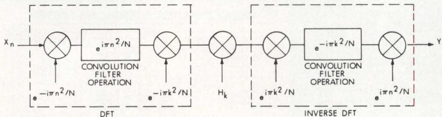
Fig 2 Chirp z-transform can be used to compute DFT in Fig 1. Time signal is multiplied by linear fm waveform, filtered in chirp convolution filter, and multiplied by another fm waveform. Inverse DFT is performed similarly
