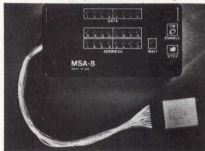
able tool for microprocessor system checkout. It connects directly to such microprocessors as the 8080A, 8085, and Z80. Data, address, and ready displays are featured. Computer System Dynamics, 2780 S Main, Salt Lake City, UT 84115 has provided single step, single step enable, trace enable, and breakpoint thumbwheel switches for control.
