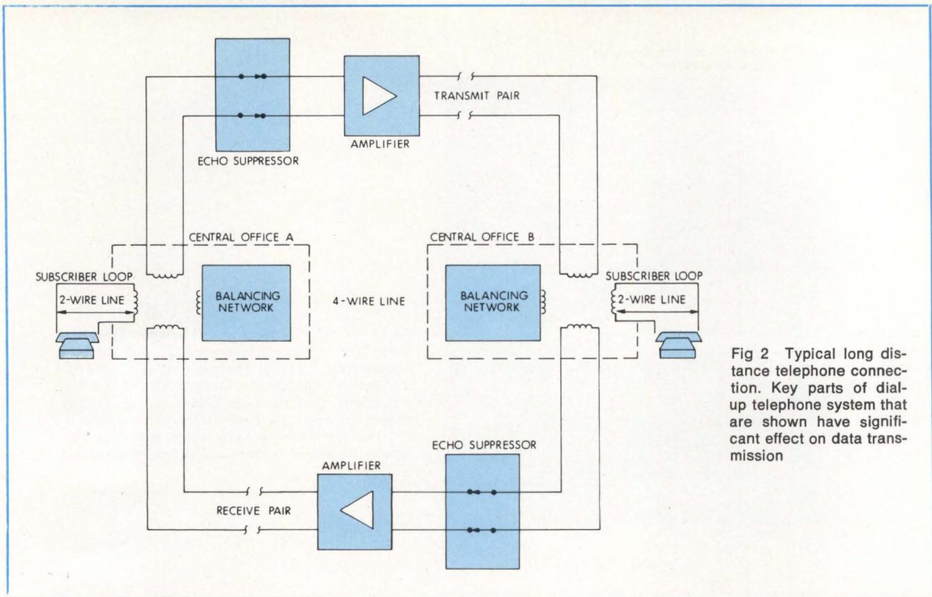
Fig 2 Typical long distance telephone connection. Key parts of dial-up telephone system that are shown have significant effect on data transmission
