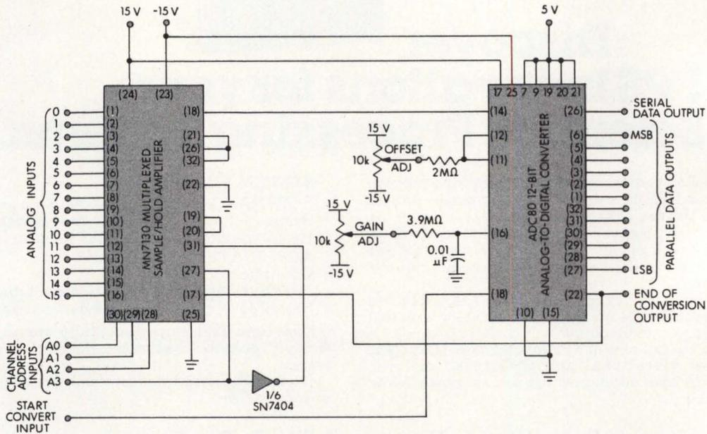
Micro Networks' MN7130 amplifier can be used in conjunction with ADC80 or MN5240 ADCs to configure an inexpensive data acquisition system in minimum board space. Throughputs of 30k channels/s are achieved with the ADC80. Typical 16-channel single-ended input data acquisition system operates in  $\pm 10$ -V input range. In data acquisition applications, sample/hold command input can usually be driven directly from ADC end-of-conversion output
