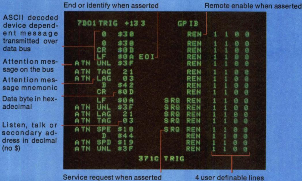
Announcing *visible* GPIB communications at the touch of a button: the new TEKTRONIX DF2 Display Formatter. The DF2 monitors and displays activity on the GPIB bus as disassembled instructions in familiar IEEE 488 mnemonics.
