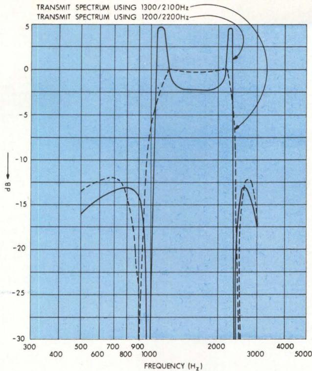
Fig 1 Transmit spectrum. Transmit spectrum (solid line) is highly peaked at 1200- and 2200-Hz frequencies. Transmit spectrum using 1300/2100 Hz, shown with dotted lines, provides 2 to 1 improvement in system performance without any impact on cost. Narrower bandwidth transmitter delivers more energy to receiver with less distortion (no peaks at mark and space frequencies)
