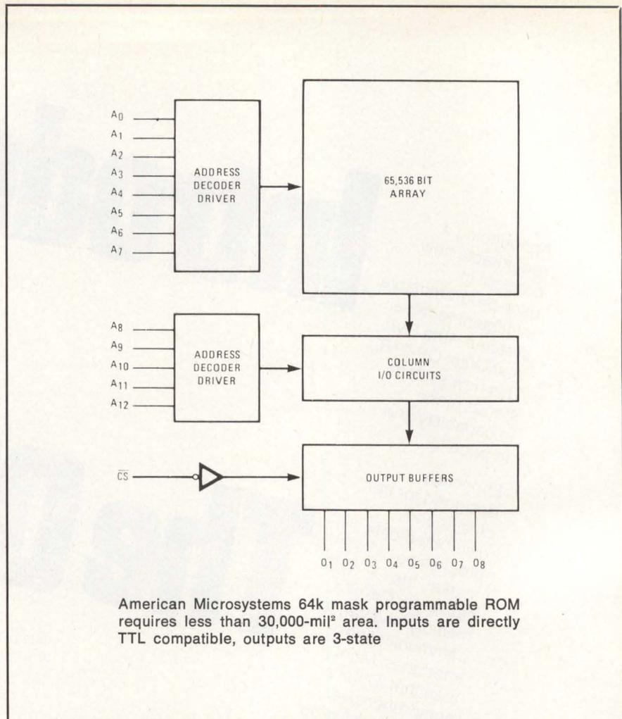
American Microsystems 64k mask programmable ROM requires less than 30,000-mil<sup>2</sup> area. Inputs are directly TTL compatible, outputs are 3-state
