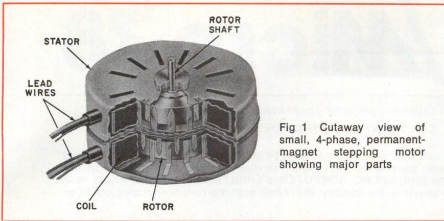
Fig 1 Cutaway view of small, 4-phase, permanent-magnet stepping motor showing major parts
