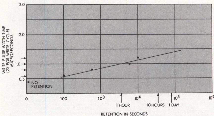
Fig 1 Retention vs write speed on a radiation hardened MNOS IC
