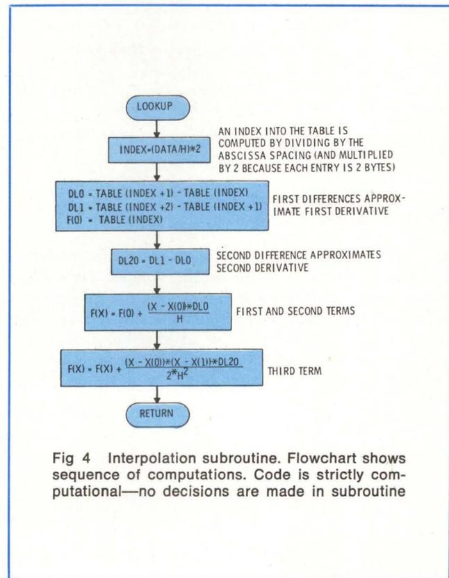
**Fig 4** Interpolation subroutine. Flowchart shows sequence of computations. Code is strictly computational—no decisions are made in subroutine
