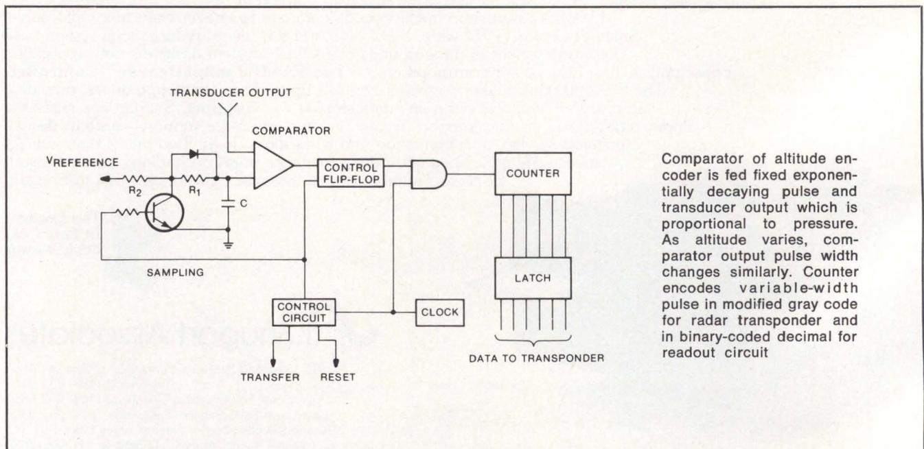
Comparator of altitude encoder is fed fixed exponentially decaying pulse and transducer output which is proportional to pressure. As altitude varies, comparator output pulse width changes similarly. Counter encodes variable-width pulse in modified gray code for radar transponder and in binary-coded decimal for readout circuit
