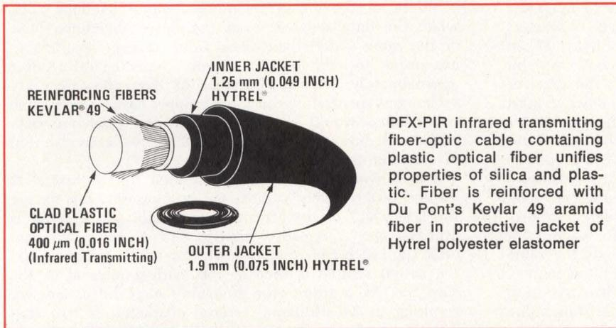
PFX-PIR infrared transmitting fiber-optic cable containing plastic optical fiber unifies properties of silica and plastic. Fiber is reinforced with Du Pont's Kevlar 49 aramid fiber in protective jacket of Hytrel polyester elastomer
