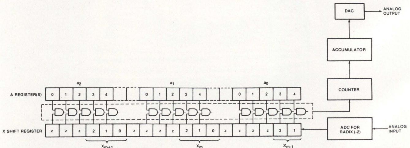
Four basic elements: fixed register (A) holds coefficients  $a_i$  prescribing filter transfer function; shift register (X) holds input words  $x_i$ ; counter computes number of TRUE gates after every shift of register X; and accumulator combines  $J$  counter outputs through shift-and-add sequence to generate output word  $y_m$
