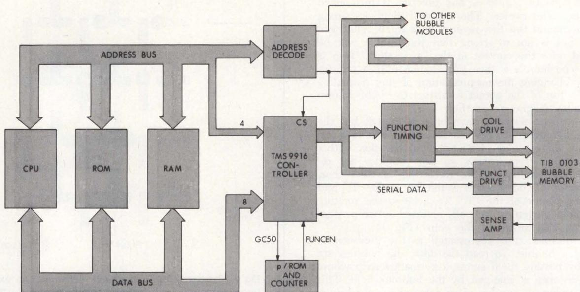
Fig 4 Block diagram of typical bubble memory interfaced to a microcomputer. Single controller handles entire system (Courtesy Texas Instruments Inc)
