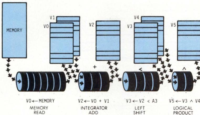
Fig 4 Chaining example. Chain of four instructions reads vector of integers from memory, adds that vector to another, shifts sum, and finally forms logical product of shifted sum and mask vector. Diagram illustrates how functional units may be considered links in chain which works as a whole to produce first result
