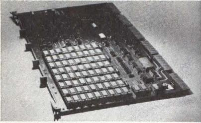
Hardware and software compatible with DEC PDP-11/04 and -11/34 computers, in-5034 add-in memory system uses high speed 8k/16k MOS RAMs to provide 32k, 48k, or 64k x 18-bit capacity on a card that measures 15.4 x 0.375 x 8.4" (39.1 x 0.95 x 21.3 cm) and fits a single hex-height card slot. Reliability features include parity checking and generation and control status register. Pretested onboard spare memory devices are provided. **Intel Memory Systems**, 1302 N Mathilda Ave, Sunnyvale, CA 94086.
