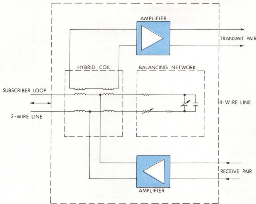
Fig 3 2/4-wire terminating set. Circuits that comprise equipment shown in Fig 2 at central office A and B are shown in greater detail
