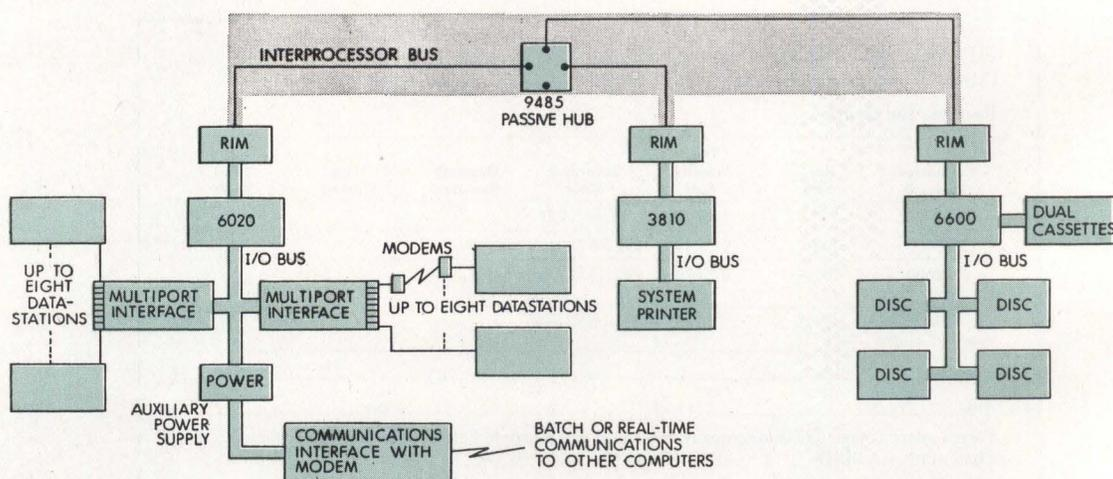
Basic configuration of Datapoint's attached resource computer (ARC) system. Key feature is modular construction. System can grow in power and tasks performed as requirements increase. Processors can be added and more disc drives can be attached when needed. If any system component fails or is otherwise taken offline, system continues to function
