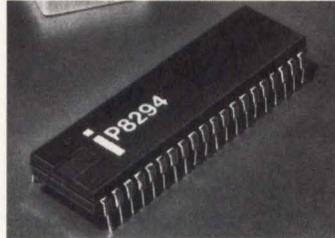
Encryption and decryption of data are carried out by the Intel Corp 8294 DEU using the NBS approved algorithm. This device, a peripheral to MCS-85, -80, and -48 microprocessors, operates on 64-bit text words using a 56-bit user-specified key to produce 64-bit cipher words. For decryption, the cipher word is operated on to produce the original text word. Although the algorithm is maintained permanently in the device, the key can be changed at any time by the user.
