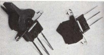
572 series includes 2 sizes of rockers and levers—0.365 x 0.648" (0.927 x 1.646 cm), and 0.595 x 1.036" (1.511 x 2.631 cm); and 0.365 x 0.740" (0.927 x 1.879 cm), and 0.595 x 1.174" (1.511 x 2.982 cm), respectively. Molded nylon actuators are available in 7 colors. Other options include 6 types of terminals, 9 different switching functions, and std, low level, or combination std/low level contact rating. **Dialight, a North American Philips Co**, 203 Harrison Pl, Brooklyn, NY 11237.
