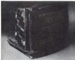
dim, and reverse video; cursor is displayed as a blinking field. RS-232 data interface is std, with 20-mA interface optional. Unit has RS-170 compatible video output. **Ann Arbor Terminals, Inc.**, 6107 Jackson Rd, Ann Arbor, MI 48103. Circle 259 on Inquiry Card
