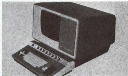
Terminal operates in English plus any other language, displaying two char sets on the same screen. Operator can enter data from right to left or vice versa. Char representation is accomplished on a 10 x 15 matrix. Terminal includes insert, delete, and text editing features; a memory of up to 73k; a 126-station keyboard; and a 15" (38-cm) diag display. Transmission rates are 50 baud to 38.4k baud serial, 10,000 char/s parallel. **Megadata Corp.**, 35 Orville Dr, Bohemia, NY 11716.
