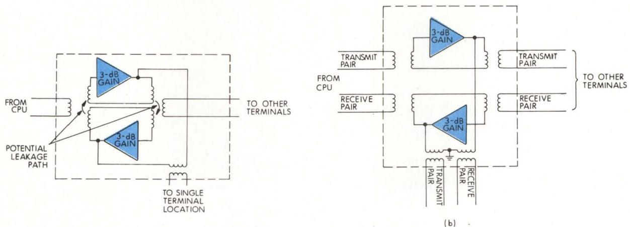
Fig 5 Simplified 2- and 4-wire bridges. 2-wire bridge (a) is used in 2-wire leased-line multidrop network to couple single terminal location to main line. (Bridge circuit is shown in detail in Fig 3.) 4-wire bridge (b) is used in 4-wire leased-line multidrop network where dedicated pair of wires is available for transmission in each direction. Completely separate amplifier is used for each direction, eliminating need for balancing network and its attendant drift problem
