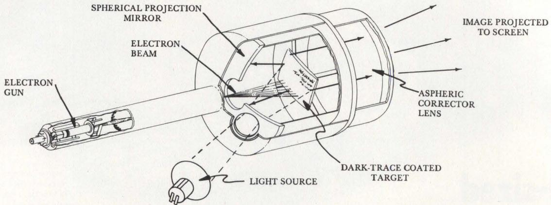
Catadioptric projection CRT used in Advent Corp's computer graphic video projector system. Normal 30-image/s flicker is not present since refresh is not required (which also eliminates need for refresh memory)
