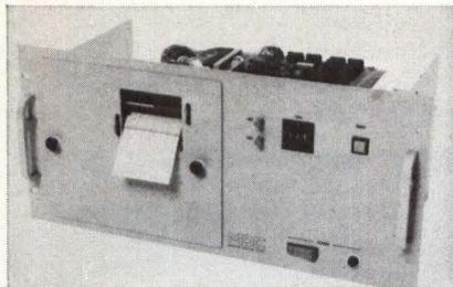
For use with Data Precision model 3400 and 3500 multimeters, 300 series 16- or 21-col printers are available in bench-top or rackmount packages. Quiet operation is achieved using a pressure printing technique; 2-color printing is provided by using an easy-to-load ink ribbon cassette. Units are available with up to 6 col of floating decimal points, and can include a date/time clock and event counter as options. **Master Digital Corp**, 1308-F Logan Ave, Costa Mesa, CA 92626.
