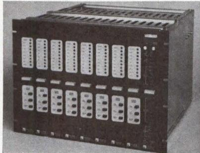
dial or 4-wire dedicated point-to-point or multidrop circuits. Size allows 9 modems to fit on 1 shelf of a std 19" (48-cm) rack, and 36 in a std 6' (1.8-m) equipment cabinet. Modems can be plugged in and removed from racks even while power supply is on without disrupting other modems in the rack. Each has separate rectifiers, filters, and power regulators, with 9-LED display and front panel pushbuttons for self-test modes. **Racal-Milgo, Inc**, 8600 NW 41st St, Miami, FL 33166.
