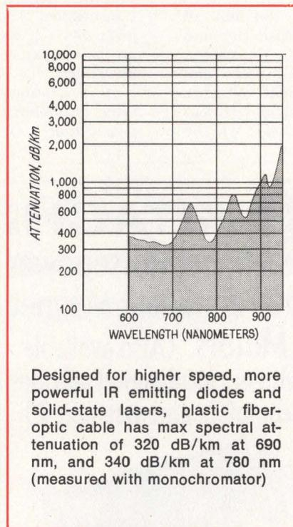
Designed for higher speed, more powerful IR emitting diodes and solid-state lasers, plastic fiber-optic cable has max spectral attenuation of 320 dB/km at 690 nm, and 340 dB/km at 780 nm (measured with monochromator)
