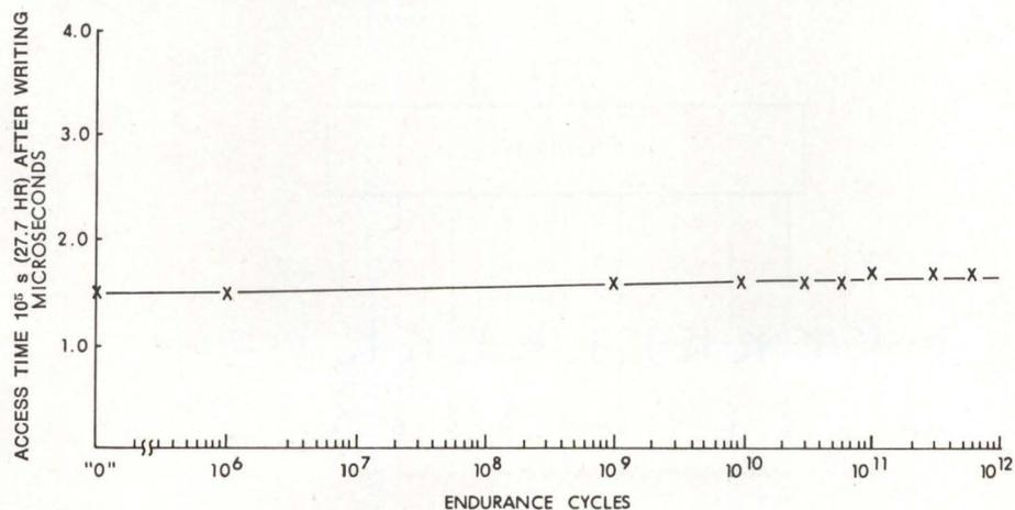
Fig 3. Endurance data after 27 hours of retention. Write cycle was 3  $\mu\text{s}$  at 30 V for retention measurement. Endurance stress was same as for Fig 2
