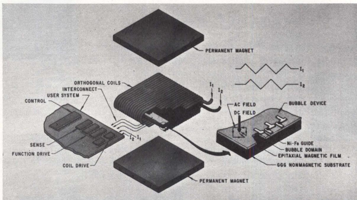
Fig 1 Construction of magnetic bubble memory (MBM). Bubbles form as flux reversals on nonmagnetic substrate positioned between two permanent magnets. They are then propagated in shift register fashion by changes in magnetization of permalloy magnets above substrate (Courtesy Texas Instruments Inc)
