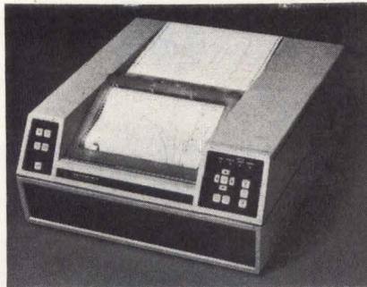
Desktop HP 7245A printer/plotter measures 19.1 x 17.5 x 7.9" (48.5 x 44.3 x 20 cm). It interfaces to systems interconnected with HPIB/IEEE-488 interface bus. 12-resistor thin-film printhead prints 7 x 9 half-shifted matrix characters; 14 x 9 matrix font is used for printing titles
