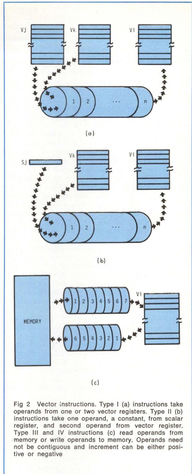
Fig 2 Vector instructions. Type I (a) instructions take operands from one or two vector registers. Type II (b) instructions take one operand, a constant, from scalar register, and second operand from vector register. Type III and IV instructions (c) read operands from memory or write operands to memory. Operands need not be contiguous and increment can be either positive or negative
