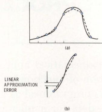
Fig 1 Linear approximation of plotted curve. Arbitrary curve (solid line) is approximated by discrete points and linear interpolation between points (a). Enlargement of one segment (b) identifies maximum error due to approximation
