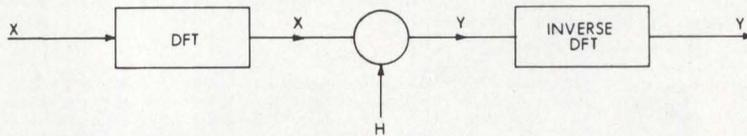
Fig 1 Convolution filtering in frequency domain can be performed using discrete Fourier transforms (DFTs). Time-domain signal is operated upon with DFT and is multiplied by transform of desired impulse response (H). Signal is reconverted to time domain by inverse DFT
