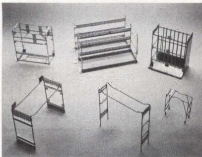
Typical minicomputer wireframe chassis illustrate open access inherent in wire construction to facilitate assembly, access, and service of electronic components. Concept is amenable to variety of computer equipment sizes and shapes and to addition of strip or sheet sections
