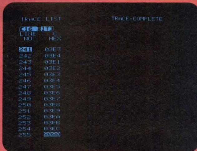
**Observing state display** shows address flow at the moment the glitch occurs and reveals that the I/O port address 8080 always occurs at the same time. This would lead you to observe I/O related signals for transitions occurring simultaneously with the glitch.
