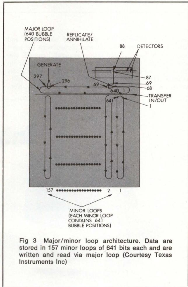
Fig 3 Major/minor loop architecture. Data are stored in 157 minor loops of 641 bits each and are written and read via major loop (Courtesy Texas Instruments Inc)
