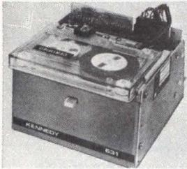
Requiring only a dual-voltage power supply, model 631 dissipates 22.6 W max during start; when running, consumption drops to 8.2 W. Transport electronics require only 1 W while a high accuracy Swiss shell-wound motor consumes 22.6 W during ramps and 7.2 W while running. The device eliminates warping on new media, while a multi-
