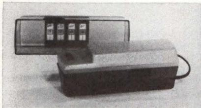
Short wave lamp features simple operation and safety features for small system user and computer hobbyist. Lamp erases up to 4 chips at a time in 14 min. Safety interlock system protects user against accidental UV exposure. Lightweight and compact system comes with holding tray for maintaining constant exposure distance of 1" (2.54 cm), and is available in 115- or 220-V models. **Ultra-Violet Products, Inc**, 5100 Walnut Grove Ave, San Gabriel, CA 91778.
