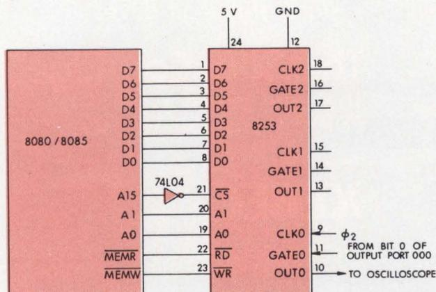
Fig 1 Interface circuit between 8253 programmable interval timer and 8080/8085 microcomputer. Timer uses four locations of memory in this memory-mapped interface circuit
