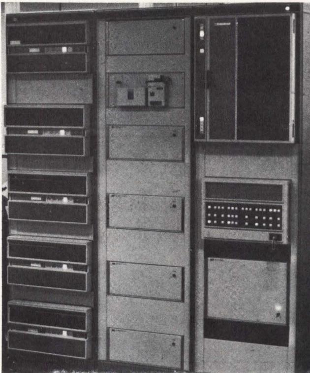
Fig 3 Portion of input subsystem hardware shown in Fig 2. HP2100 with 32k memory controls subsystem. Data base is maintained in five 5M-byte HP79000 disc drives
