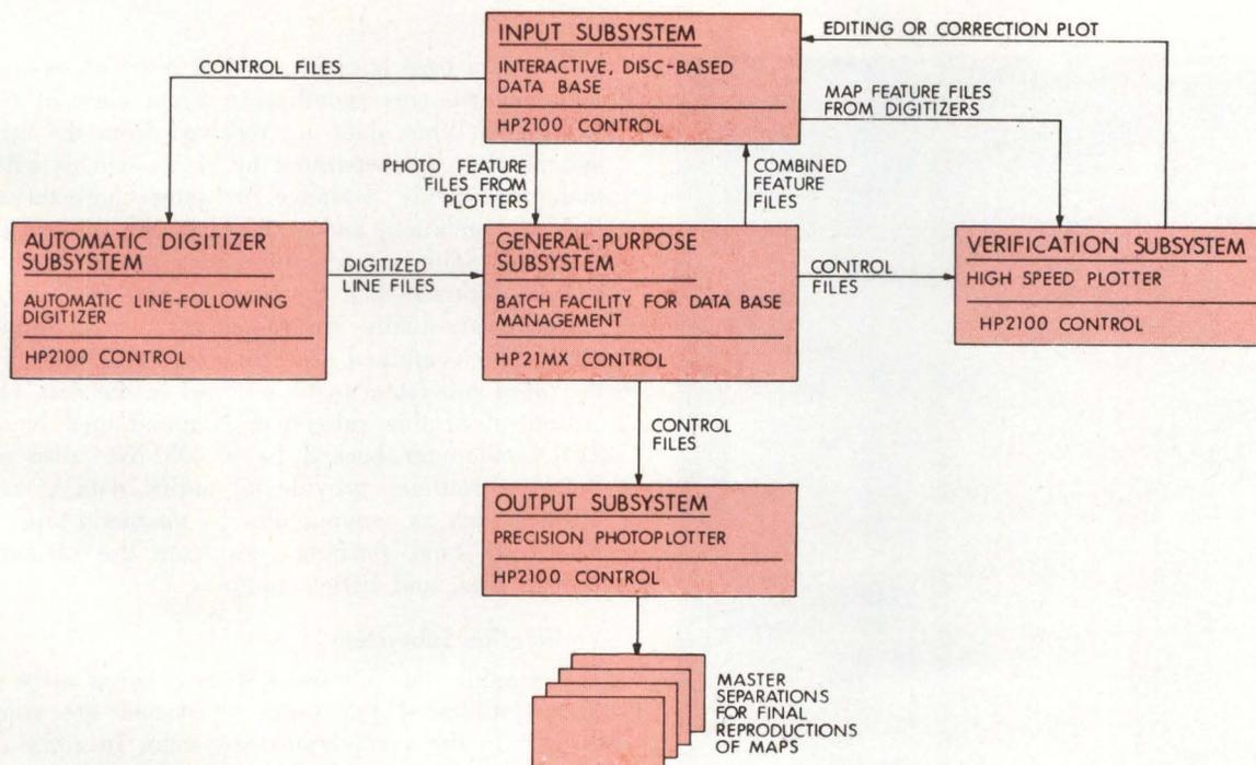
Fig 1 Overall block diagram of Automap system showing basic flow of data. Each subsystem includes magnetic tape unit which accepts data from or transfers data to other subsystems. Usual flow of data is from input to general-purpose to output subsystems; however, in some situations, flow could be directly from input subsystem to output subsystem
