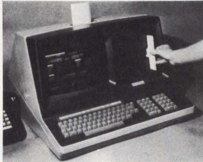
and an interactive diskette operating system. The package also holds a 24 x 80-character 12" (30-cm) CRT, a 2200-char/s nonimpact printer, and single or dual minidiskettes. Internal printer, dual diskettes, and memory expansion beyond 32k are optional. An external printer is also available.
