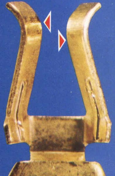
Arrows indicate contact surface still smooth, clean, free from abrasions.
