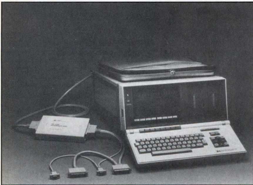
Soft key operation, BASIC programmability, and flexible protocol support are featured in the HP 4955A protocol analyzer. Internal 128k-word storage and dual 256k-byte tape drives provide mass storage for offline analysis of data streams and setup and measurement sequence storage.
