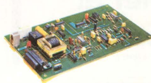
Remote Monitoring Equipment Modem
