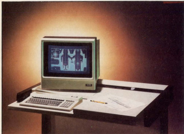
The Lundy S6100 workstation, with 448- x 1024-pixel graphics, introduces GKS functionality to the U.S.
