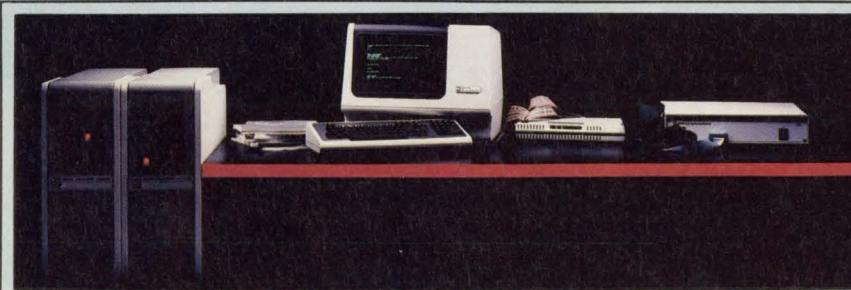
National Semiconductor's SYS 16 development system includes high level language compilers, realtime in-system emulation tools, over 3 Mbytes of RAM, and up to 140 Mbytes of hard disk for demand-paged virtual memory support.
