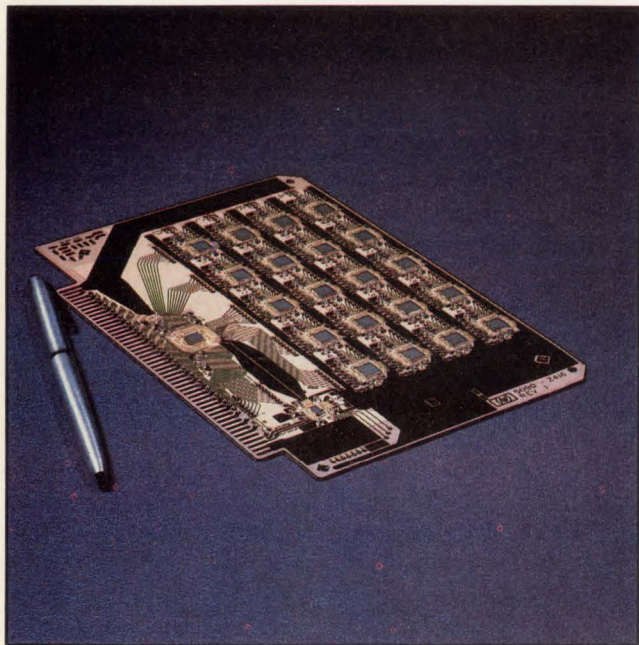
A special copper-clad circuit board was developed to deal with the power and cooling requirements of the chip sets used in the HP 9000.
