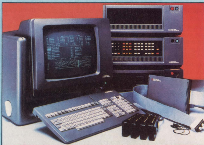
The Kontron KDS development system combines CPU, mass storage, slave in-circuit emulation, and logic analysis to integrate many design functions.
