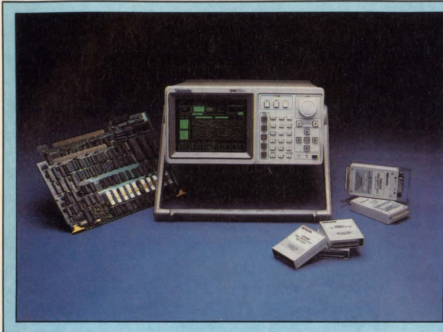
The Tektronix 1240 logic analyzer is expandable to 72 channels and offers advanced software performance analysis.
