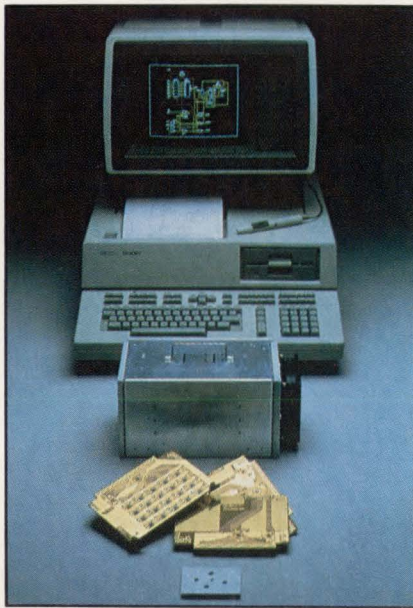
Five-chip set in foreground mounts on boards (above chip set) as nucleus of 32-bit HP 9000 computer. Module in center is rackmounted version; background unit is standalone workstation.
