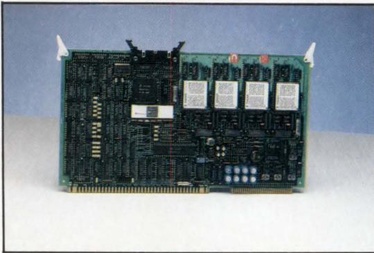
Offering built-in 1-Mbit bubble devices, the FBC504M4M series provides four different memory capacities—128, 256, 384, and 512 Kbytes. The card operates as memory-mapped I/O requiring only a 64-byte memory space. Advantages include a single 5-V power source, an internal power fail protection circuit, and data retention even without power.
