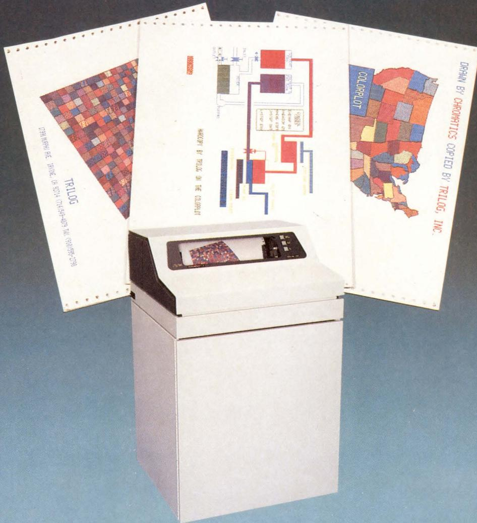
TRILOG's patented multicolor technology provides full color as well as conventional printing on plain fanfold paper at 100 dots per inch resolution.
