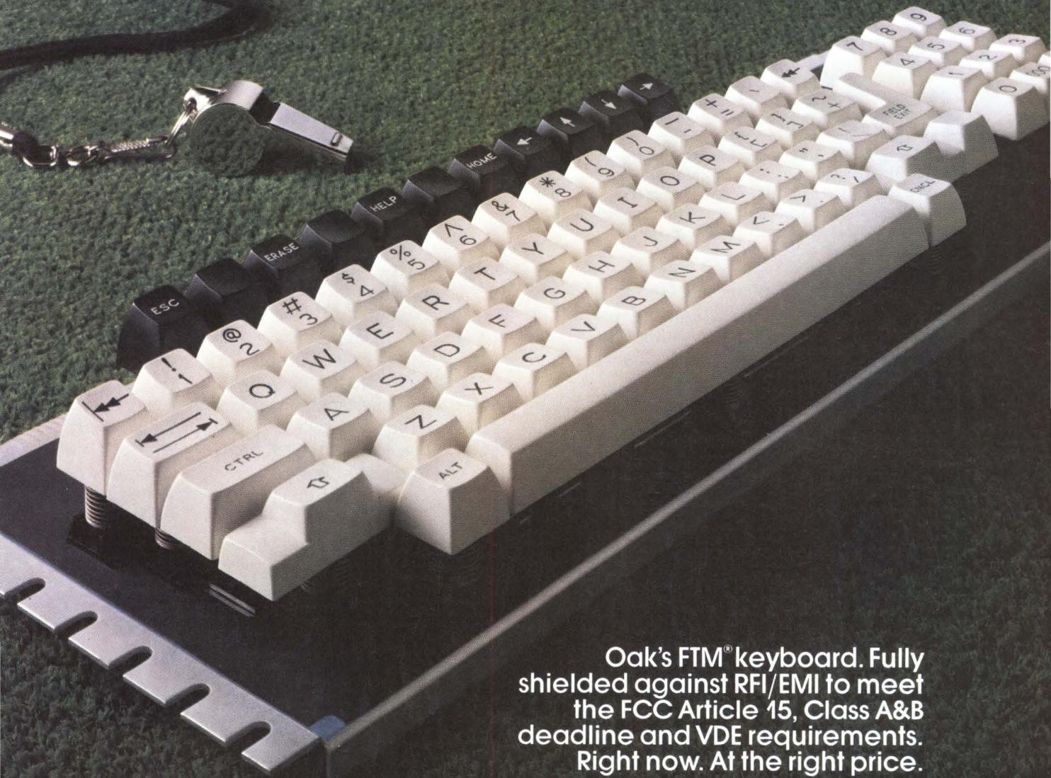
Oak's FTM<sup>®</sup> keyboard. Fully shielded against RFI/EMI to meet the FCC Article 15, Class A&B deadline and VDE requirements. Right now. At the right price.
