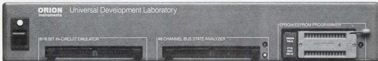
Up to 128K bytes of **ROM EMULATION** (8K standard) allows you to make program patches instantly. Since the target ROM socket connects data and address lines to both the analyzer and the emulator, no expensive adaptors or personality modules are needed.
