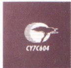
Cache Controller and Memory Management Unit
