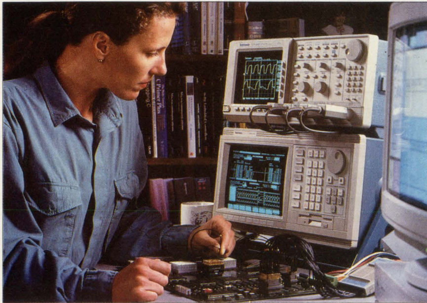
The 3001 GPX logic analyzer (below) addresses the needs of both hardware and software engineers with high-speed analysis of state and timing, disassembly, real-time performance analysis, and ROM emulation on the target system.
