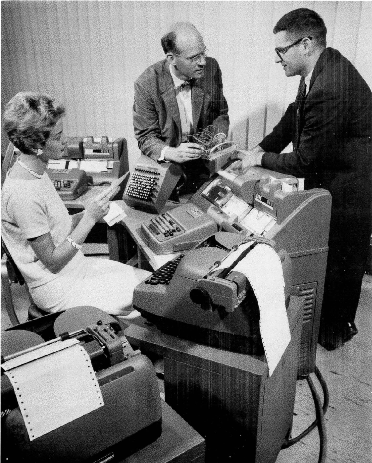
The IBM 870 document writing system shown here speaks in three languages — typewritten script, punched cards, and punched paper tape. The system includes (from top to bottom) an auxiliary card punch; an auxiliary keyboard; the control unit — with a keyboard, a card punching and a reading station, and a tape reader; and two electric typewriters. The system is controlled by a wired panel such as held by the engineer. It is designed by International Business Machines Corp., White Plains, N. Y. (Figure 11)
