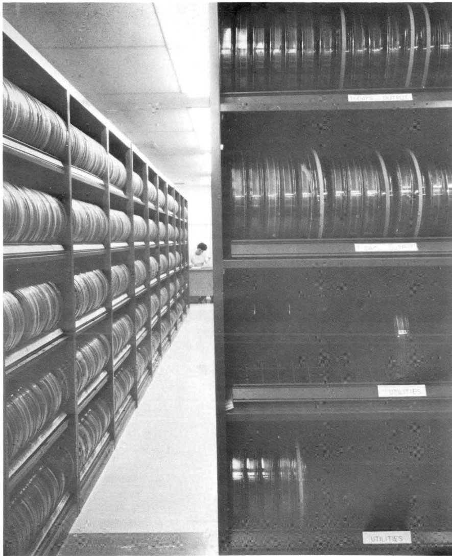
Here is a portion of the magnetic tape library at the Computation and Data Reduction Center of Space Technology Laboratories, Los Angeles, Calif. Each of these magnetic tapes can hold the information contained in 50,000 standard 80-column punch cards. (Figure 12)
