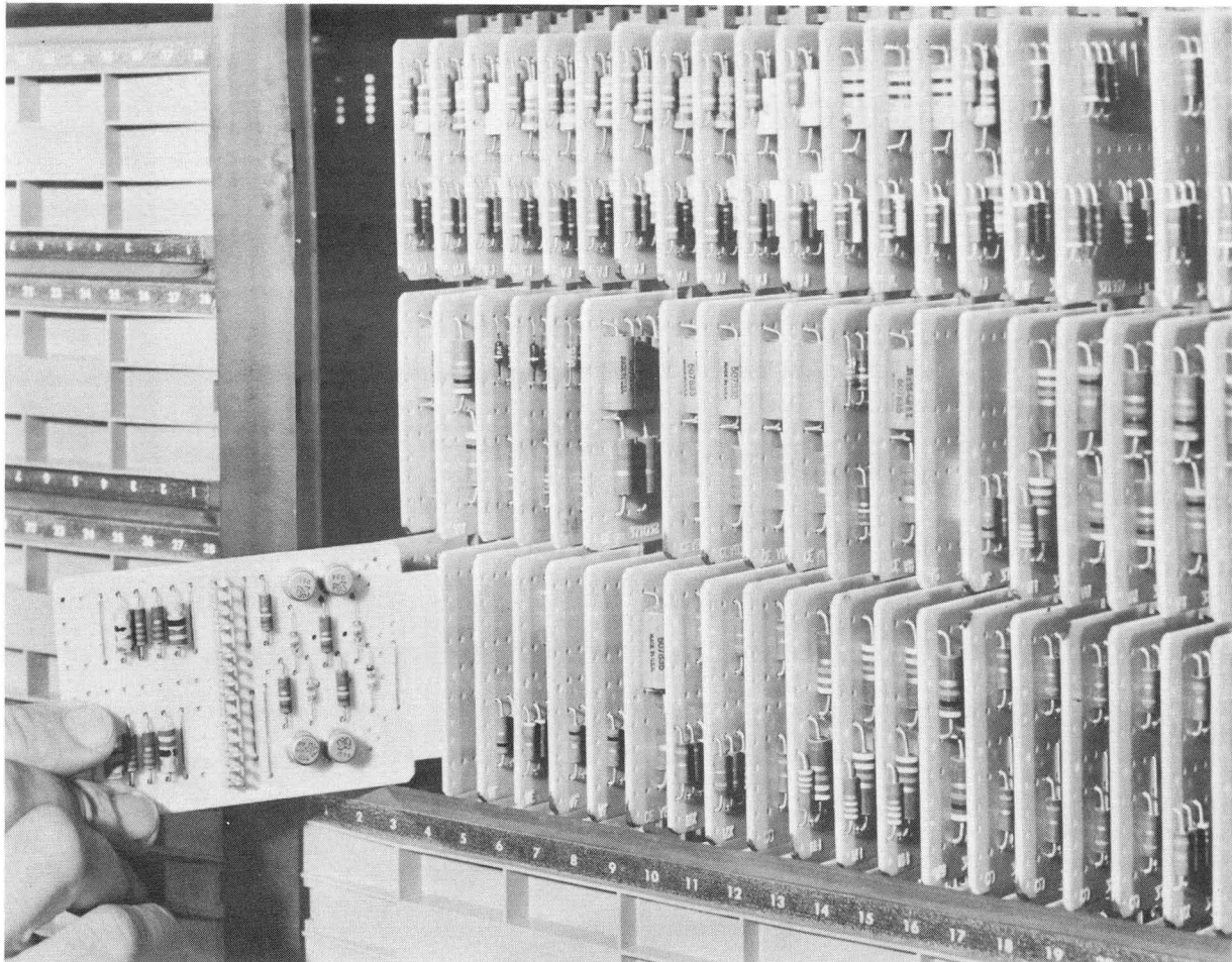
Shown below is one of the electronic component cards featured in the solid-state IBM 1620 data processing system of International Business Machines Corp., White Plains, N. Y. The button-like components at right, top and bottom, are transistors, with resistors and capacitors located near the fingers. Printed wiring matched with automatic soldering make the cards very reliable. (Figure 34)
