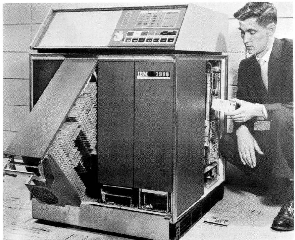
Here an engineer replaces a circuit card in the IBM 1009 data transmission unit that allows computers to exchange data core-to-core. Housed in a single standard modular system (SMS) module, the 1009 utilizes toll or leased telephone lines or high-speed telegraph lines to link solid-state computers located any distance apart across the country. The new unit has a "swinging-gate" construction which gives fast access to its electronic component cards. The unit is made by the International Business Machines Corp., White Plains, N. Y. (Figure 32)
