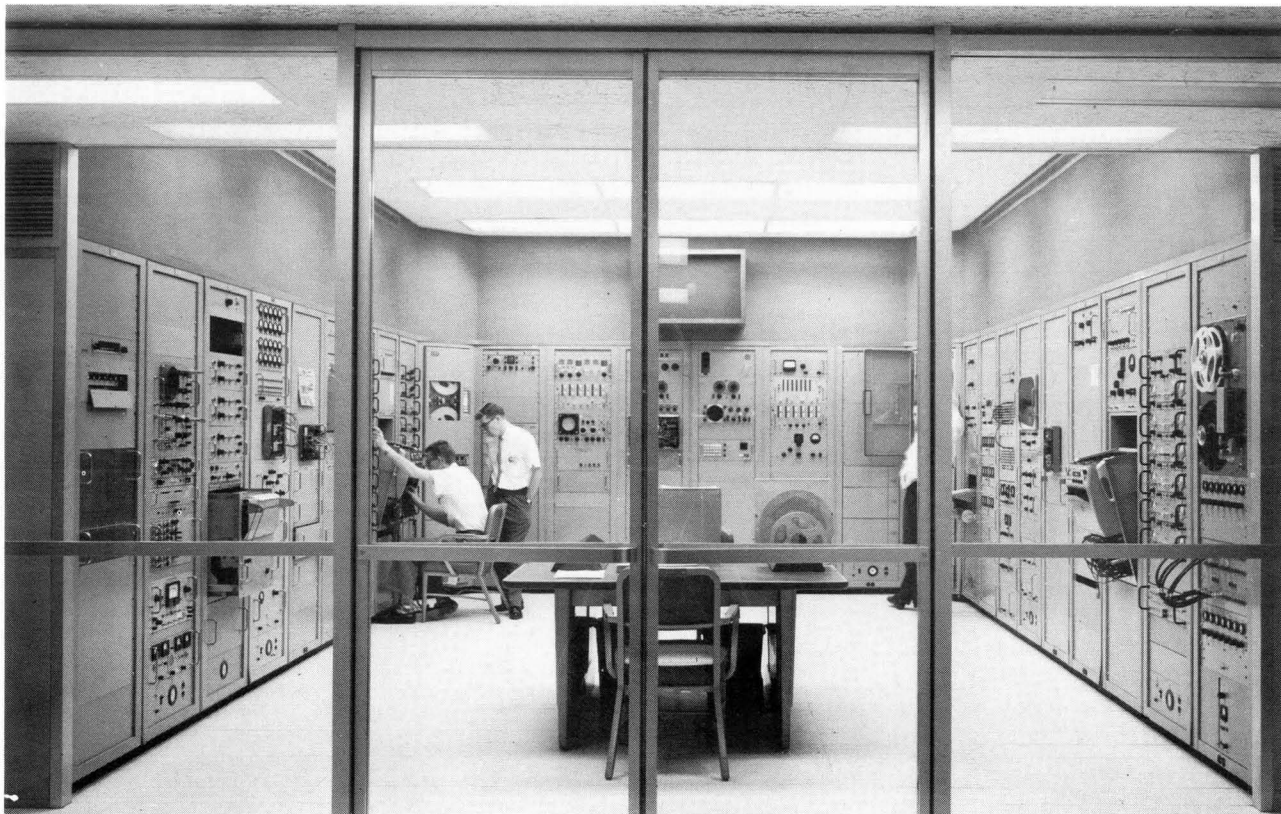
This is one of three equipment areas in Space Technology Laboratories, Inc. new Data Reduction Center located in Southern California. This equipment is used in the conversion of missile and space flight telemetry data into suitable forms for study and analysis. (Figure 1)
