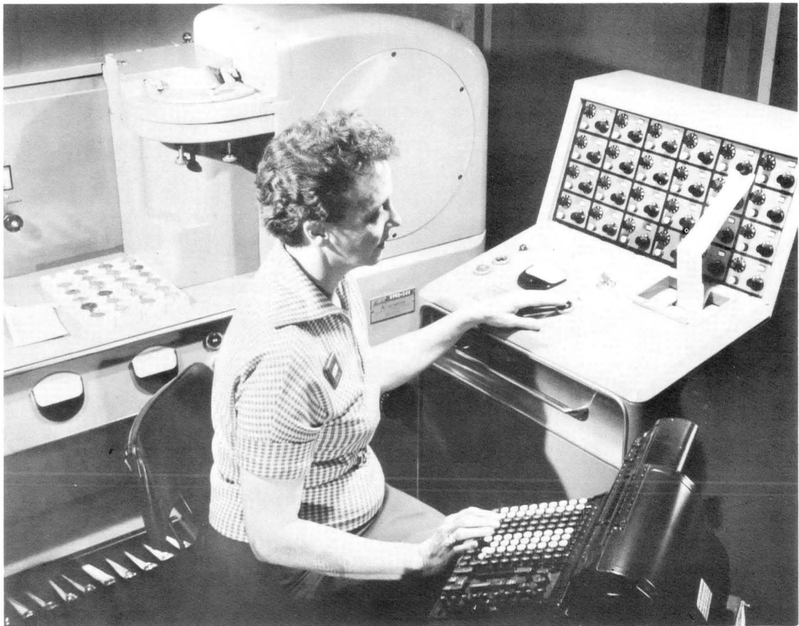
This computer-ized X-ray instrument is shown automatically comparing unknown samples of metal alloys with known standards, and printing out the ratios on tape. The instrument can be programmed to handle in any one cycle up to 24 elements, selected from atomic number 12 to atomic number 98. It is produced by Philips Electronic Instruments a division of Philips Electronics and Pharmaceutical Industries Corp., Mt. Vernon, N. Y. (Figure 4)
