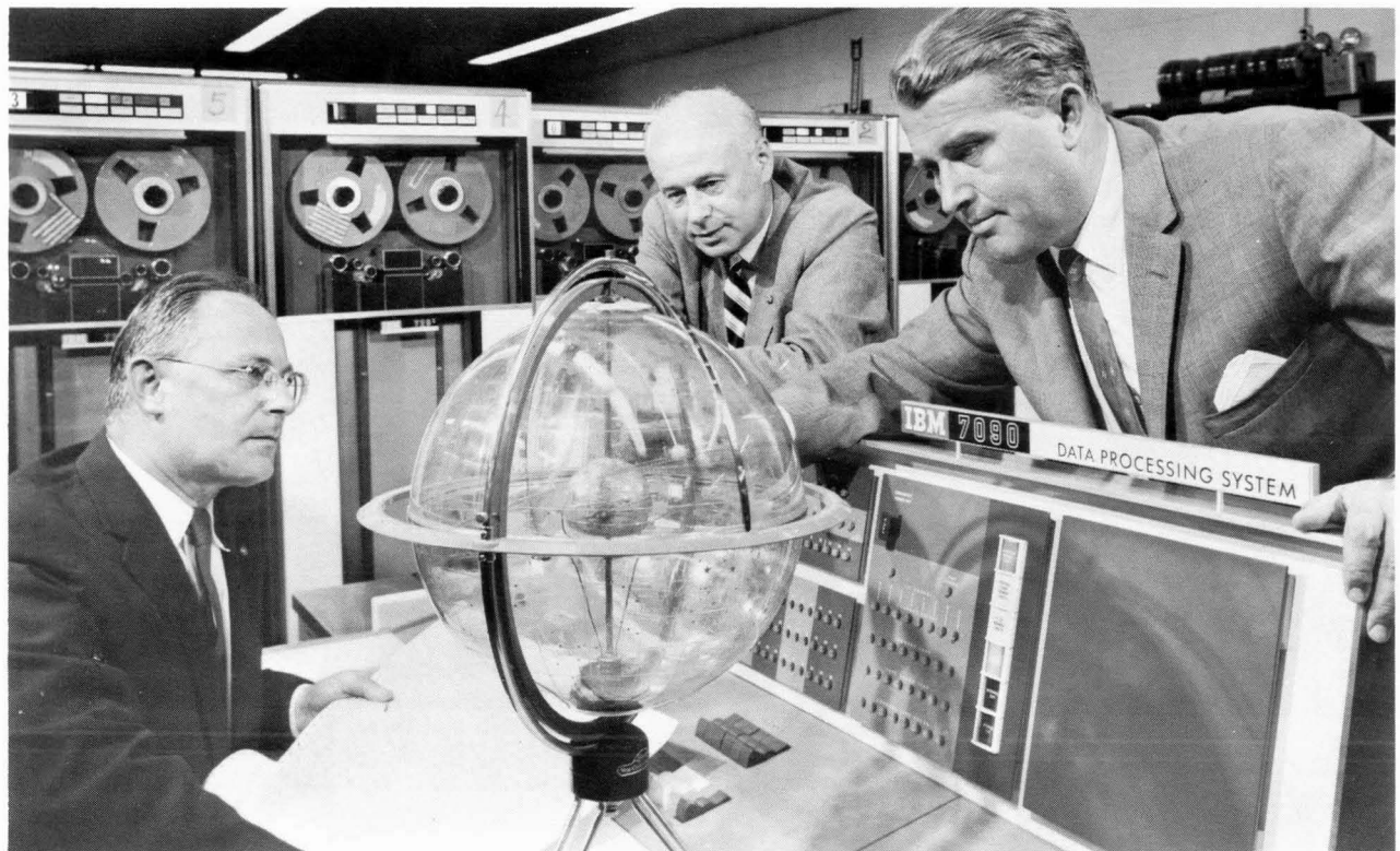
The projected performances of the Saturn missile — which will send multi-ton payloads into earth orbit; around the moon and back; and into deep space — is being studied while the huge vehicle is on the ground. Saturn's 1,500,000-pound-thrust booster will be mathematically "flown" thousands of times by the IBM 7090 computer before reaching the launching pad next year, with each flight taking only a few minutes. Here Dr. Wernher von Braun (right), Director of Marshall Space Flight Center, Huntsville, Ala., reviews solar-system flight calculation with Dr. Helmut Hoelzer (left), Director of the center's Computation Division; and Dr. Eberhard Rees, the center's Deputy Director for Research and Development. (Figure 39)
