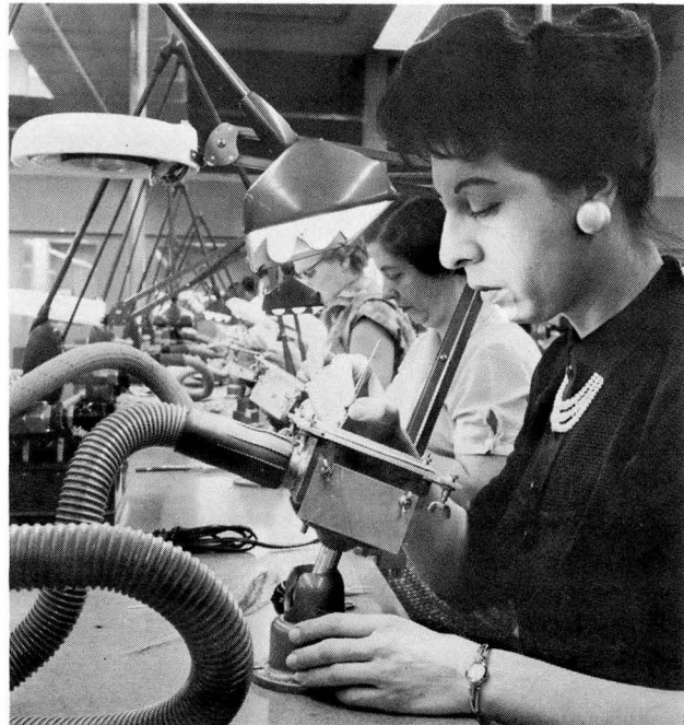
Shown is one of the arithmetic units during assembly of the SAAB D2 transistorized computer of Saab Aircraft Co., Linköping, Sweden. The computer is designed for table-top operation; it contains around 6000 transistors and 3500 diodes; and it can handle thirty-two different logical and arithmetic operations. It operates in pure binary. (Figure 29)
