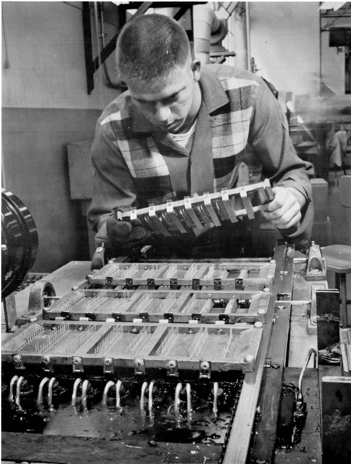
Here computer building blocks at Minneapolis Honeywell's electronic data processing division in Boston, Mass., are being assembled, using automated soldering techniques. Circuit boards ride across the solder jets in the foreground, and streams of molten solder make wire and component connections uniform. Solder joints of very high quality are made by this precisely controlled automatic technique. (Figure 19)
