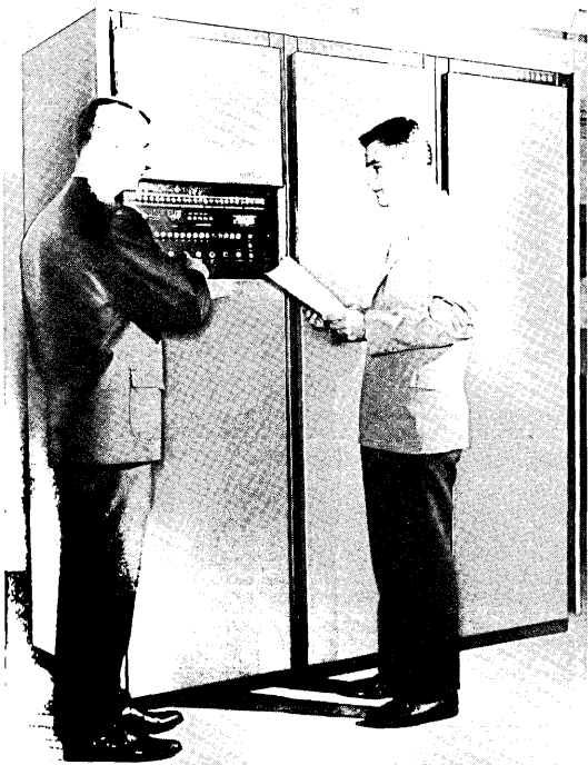
TRW-330 Digital Control Computer -- TRW Computers Co., Canoga Park, Calif. This control computer has a design based on solid-state components, modular construction, plug-in circuit cards, and Mercury-wetted-contact relays. The basic systems accepts up to 1024 variable-voltage inputs from pressure, flow, temperature, or other process state measuring instruments. It samples, converts, and stores this data with an accuracy said to be 0.1%. The work length is 24 bits, including sign. The memory capacity goes to 100,000 words in units of 4000. Speed for an addition or subtraction is 260 microseconds.
