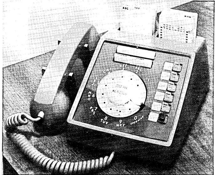
Automatic dial telephone -- Bell Telephone System, New York, N.Y. The card dialer has the automatic dialing unit in the set; it has unlimited capacity. Coded plastic cards, on which the user has previously punched out the specific telephone number, control the dialing equipment.
