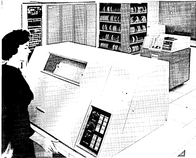
High-speed printer -- Minneapolis-Honeywell's Electronic Data Processing Div., Wellesley, Mass. The high-speed printer (foreground) prints the system's output at the rate of 900 lines a minute. In the background (l. to r.) are a multiple-purpose control unit (for printer, card punch and card reader), a magnetic tape storage rack, and a high-speed card punch.
