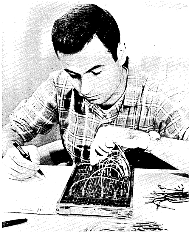
John Wickham, assistant to Dr. Donald McIntyre, chairman of Pomona College Geology Dept., Claremont, Calif., sets up a problem for the Clary DE-60 computer to solve. The computer is available to all geology students in the undergraduate college. This computer is a small general purpose digital computer, and was specifically designed for engineering and scientific applications by the Clary Corp., San Gabriel, Calif.
