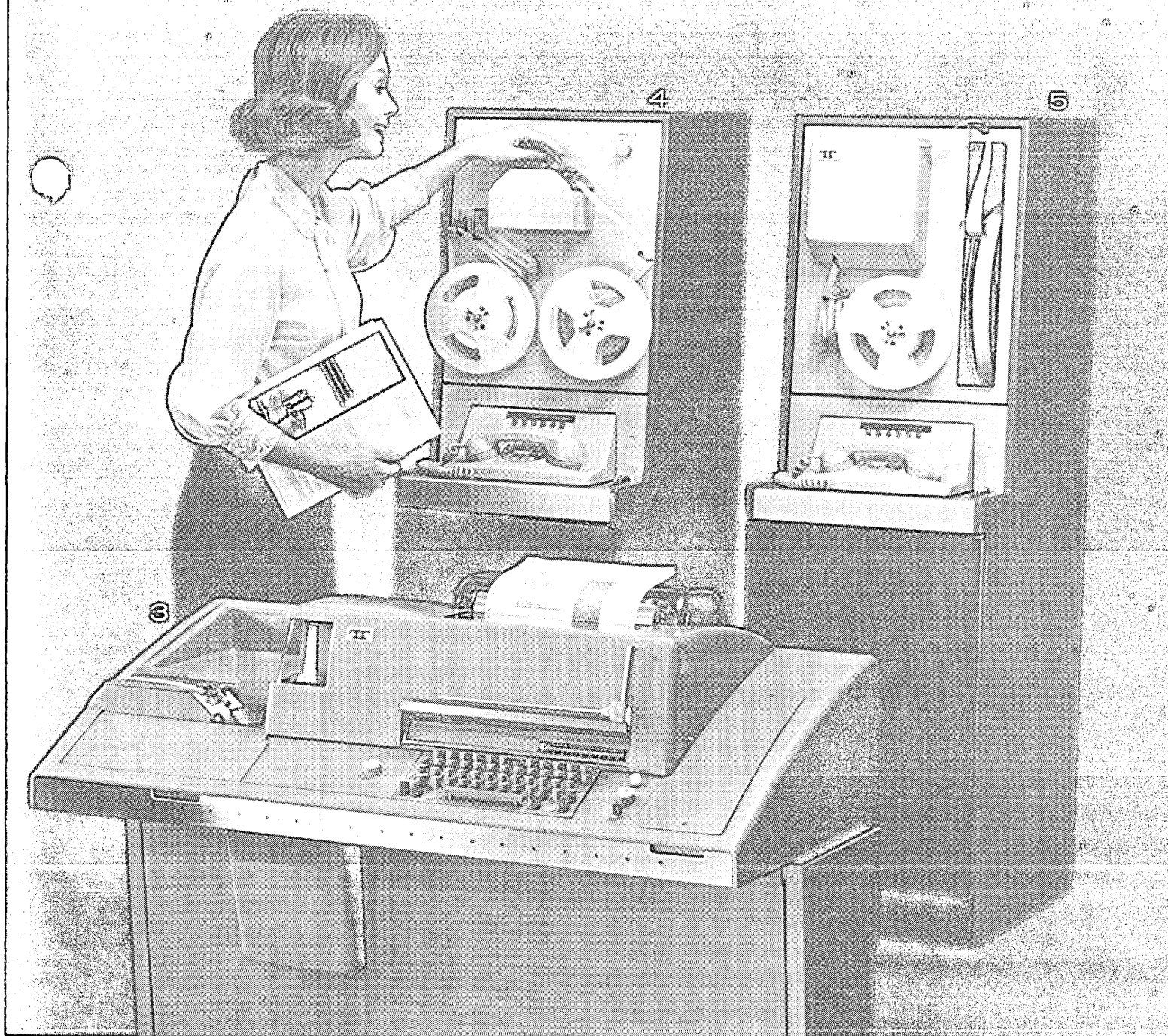
Tape-to-Tape Sending set sends from punched paper tape at 1,050 wpm. (5) Telespeed Tape-to-Tape Receiving set receives on punched paper tape at 1,050 wpm.
