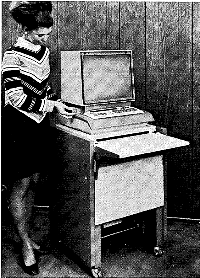
Fig. 3 DatagraphiX 1700 viewer, mounted on enclosed 3500 demand printer.
