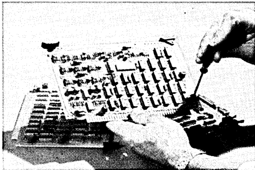
Switch options (external and on PCB's) permit field selection of modes, data rates, stop bits, parity, auto roll-up and line feed, display or non-display of cursor & carriage return symbol.
