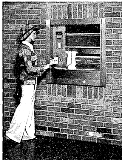
NO TELLER NCR's 770 self-service banking terminal
