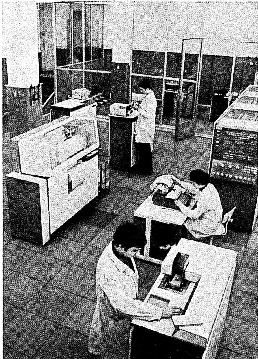
The Riad Series of computers was designed to be compatible with the IBM 360 line, and IBM software is often used with them. This one appears to be about the size of a Model 30.
