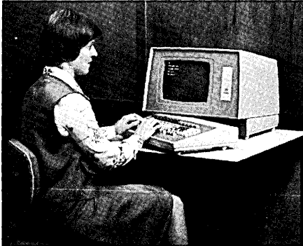
1. Our B500 is an 8080A micro-processor based video display terminal
