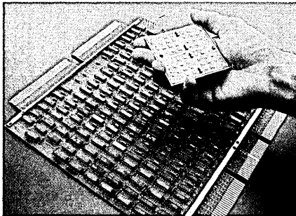
Current Mode Logic (CML) is central to DPS 88's ability to handle today's increasing workloads. CML chips are mounted on three-inch square ceramic substrates each having circuitry counts comparable to that of two conventional circuit boards.
