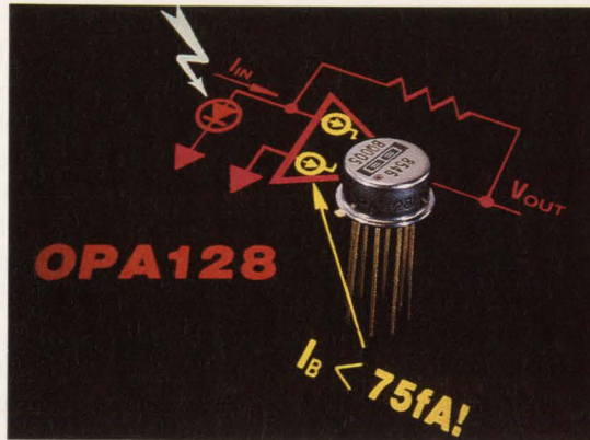
This PIN photodiode amplifier is one application for Burr-Brown's 75-fA I_B and 500- \mu V V_{IO} OPA128. Using an HP 5082-4204 photodiode sensor and a feedback resistor of 10 G \Omega , the circuit's V_{OUT} is 5V/nW.
