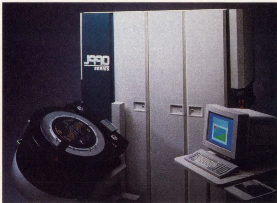
Automatic test systems for ICs are among the largest electronic systems sold today as standard products. In appearance, though not in performance, the memory-IC testers in Teradyne's J990 series are typical of the genre. The systems' 11 custom ICs provide evidence of the testers' state-of-the-art technology.
