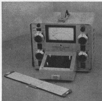
A portable test console measures electrical characteristics of all 1- to 14-lead ICs. The unit contains 6 power supplies, four of which are individually front-panel adjusted over 0 to  $\pm 15$  V. Readout is on the front panel meter or on an external DVM. Accuracy is 1% full-scale with panel meter, and 0.1% with a DVM. Voltages to 30 V and currents of 1 nA can be measured.
