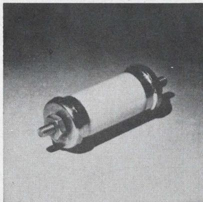
Glass-cased capacitors are suitable in high-voltage applications from  $-55$  to  $+125^\circ\text{C}$  with no voltage derating. The paper-plastic film dielectric, the high dielectric strength of the impregnant, and the thermal glass tubing provide size and weight reductions.
