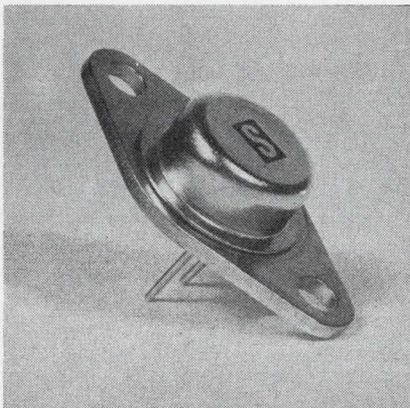
Series MHT 7901 through 7904 transistors are 10-A planar npn devices featuring sustaining voltages from 200 to 300 V. The transistors are offered in a TO-66 package with a power rating of 25 W at 100°C case temperature.  $I_{CBO}$  is 1  $\mu$ A max,  $V_{CE/SAT}$  is 0.5 V max at 5 A and  $h_{FE}$  is 50 MHz.
