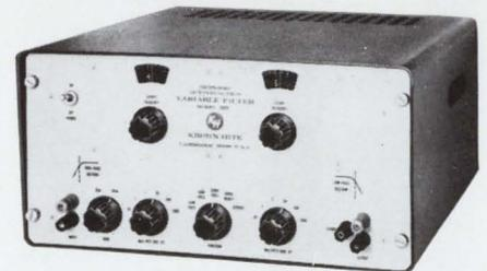
**THIS KROHN-HITE VARIABLE FILTER** provides low-pass, high-pass, band-pass, and band-reject operation with high and low cutoff frequencies independently adjustable from 0.02 cps to 20 kc.
