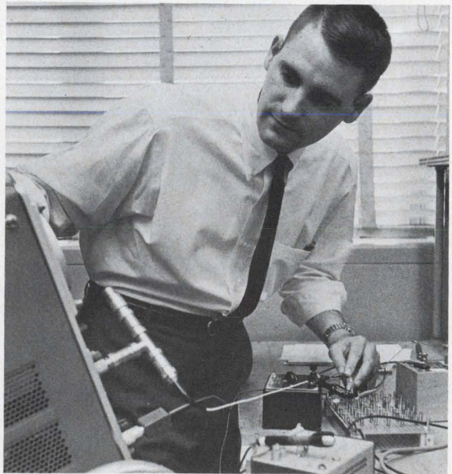
No trace of hysteresis is shown by the CRO. Author Spofford makes waveform measurements on his SBS phase-control circuit. Gate lead on device permits operation without snap-on effect associated with other semiconductor triggers.
