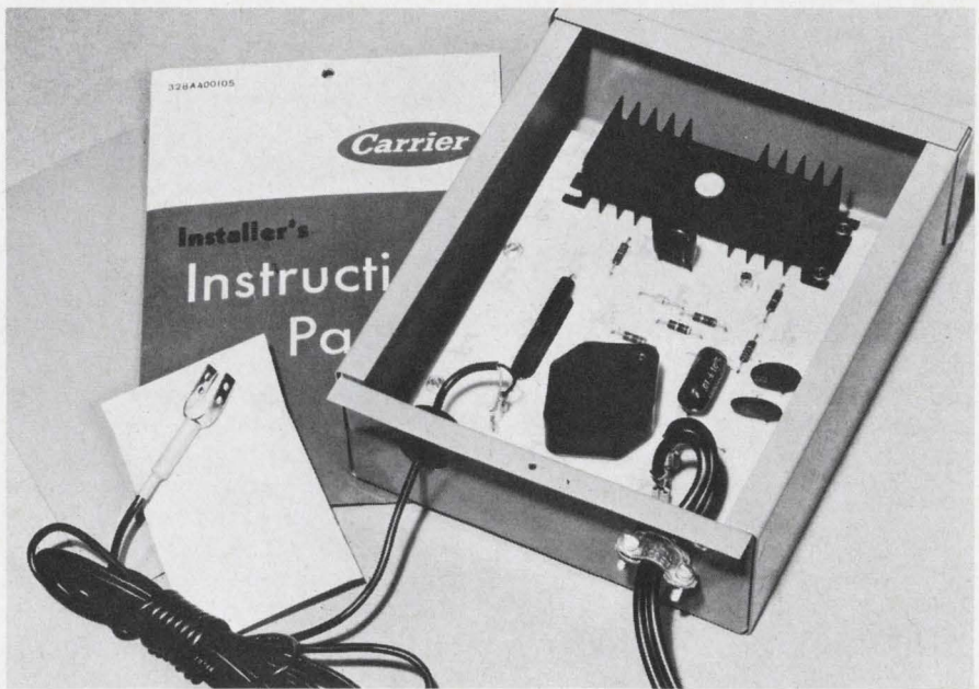
8. Compact control unit regulates the speed of air-cooled condenser fans in accordance with outdoor temperatures. The unit makes possible air-conditioner operation over an outdoor temperature range of -20^{\circ} to +115^{\circ} F.
