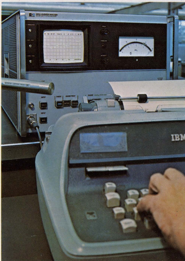
Subject loudness is plotted on the scope face while the meter shows the absolute loudness. Hewlett-Packard's loudness analyzer selects the proper spectrum with comb filters and performs complex analog signal processing to arrive at these data, which formerly had to be calculated manually. But there are no linear integrated circuits in the filter system.
