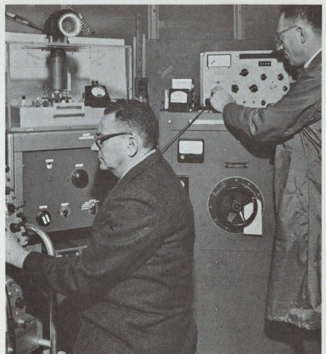
While author Shar stands by analyzer that'll show the distortion product, another engineer checks test signal.
