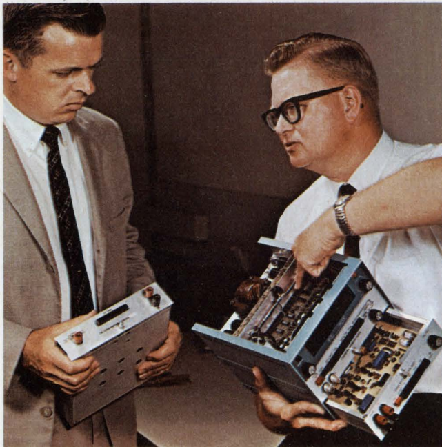
What's in the box? A portable test instrument, that can function as a digital voltmeter, a digital time, frequency or period counter, or as an ac converter. The modular construction permits this flexibility, as Thomas Laugesen points out to Art Hoyt, both from Electronic Associates, Inc.
