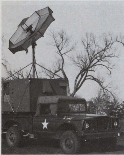
Mobility for the terminal of tactical communication satellites is provided by 1-1/4-ton truck.
