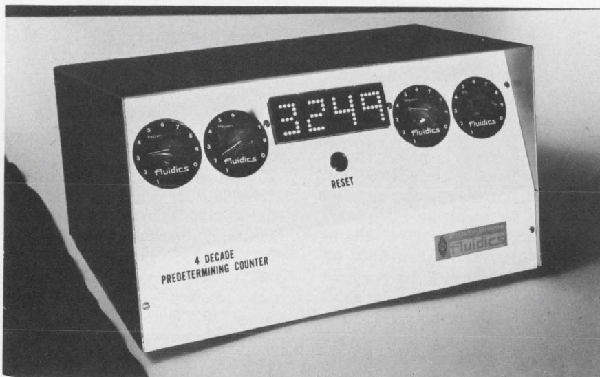
Fluidic 4-decade readout operates from air pressure. Logic pressure signals provide direct counter input without electrical or mechanical interfacing.
