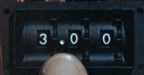
as 15 stations with our snap-on retainer band. And up to 34 of them using mounting rods. They have dust seals and solder tab termination. The dial characters are large and easy to read, and they're protected against dust and moisture by a plastic window.
