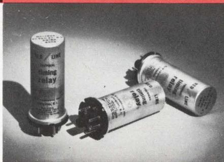
Designed to meet the most demanding applications. They are housed in shatter-proof, dust-proof metal enclosures and feature stainless steel mechanisms and encased heaters for reliable, quiet operation in any plane. **Features:** delays up to 3 minutes, operating voltages 6.3 to 115V, AC or DC.
