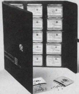
**CHIP KIT NO. 1** consists of 300 monolithic ceramic capacitor chips for hybrid circuits. Browse, examine, and test. There are 10 chips of each standard RETMA values from 1.2 pf to 330 pf in  $\pm 10\%$  tolerances at 50 VDCW.
