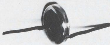
Called an energy-storage device (ESD), a new electrochemical capacitive component bridges the gap between a conventional capacitor and a secondary battery. About the size of a half-dollar, the 0.5-V ESD attains capacitances of about 50 farads with an approximate internal resistance of 1 to 2 ohms.
