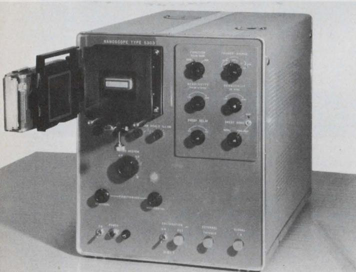
From dc to 5,000 MHz is the range of this Matsushita Nanoscope, which uses a traveling-wave CRT.
