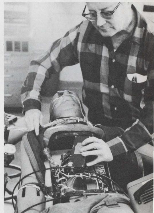
What happens to a pilot ejected from his aircraft at the speed of sound? This transducer-equipped dummy will be blasted off a rocket-propelled sled to find out.
