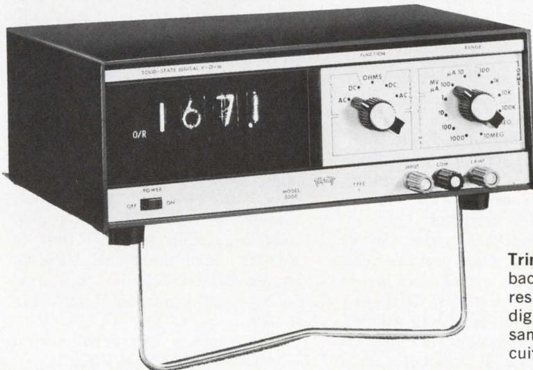
**Trim digital multimeter**, which virtually eliminates kick-back current, can make voltage measurements in high-resistance circuits at its stated accuracy. This 3-1/2-digit instrument also offers 50% overranging and a sampling rate of six times per second. Protective circuitry allows input voltages as high as 1000 V. p. U140.
