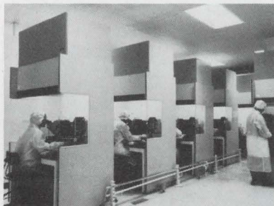
SUPER-CLEAN AIR . . . In vertical laminar-flow hoods designed to provide additional air filtering, wafer photo resist is exposed to ultraviolet light after precise mask alignment.
