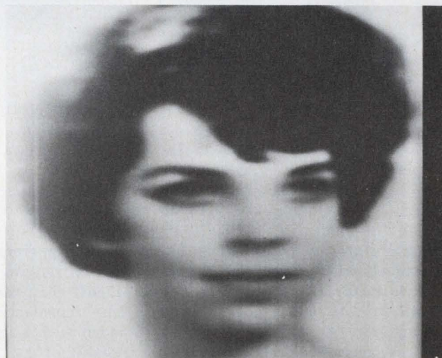
ing drum. Serial video was applied to the input of an oscilloscope. The resulting photograph (right) was taken by a Polaroid camera off the oscilloscope's screen.
