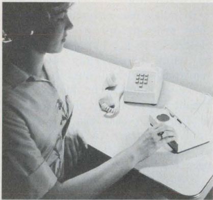
Bell's Code-Com set can enable the deaf to see or feel coded messages.
