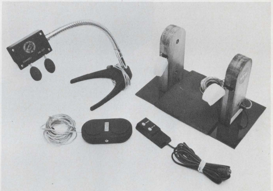
Head, foot and hand switches can also be used with NASA's control system. They offer a choice for the less severely handicapped.
