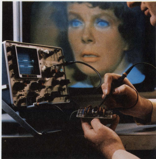
The IC on a chroma board for color television receivers is checked out by a National Semiconductor technician.
