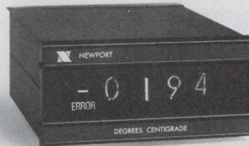
SERIES 260 DIGITAL THERMOCOUPLE INDICATOR: For TC types J,K,T,S,R,E and RTD's 1° resolution • °F or °C • -310° to +3100° F • BIGS-BCD outputs • 2 1/2" H x 5" W x 6 1/2" D.
