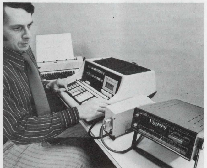
Programmable calculators are now making use of a variety of peripheral equipment. Here a Wang calculator connects to an alphanumeric plotter and digital voltmeter to form an automated measuring system.
