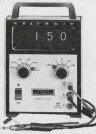
A compact, solid-state multimeter with digital readout — at a fantastic kit-form price. The new Heathkit IM-1202 has four overlapping ranges to measure voltages from 10 mV to 1000 V on DC (either polarity), 10 mV to 700 V rms on AC, 10  $\mu\text{A}$  to 2.5A on AC or DC current. Five resistance ranges measure from 1 ohm to 2.5 megohms. Front panel polarity switch reverses inputs without changing leads. 6 lbs.
