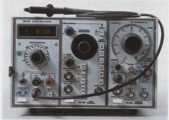
The DM-501 DMM plug-in is just one of many different units that fit into the TM-500 series of instrument mainframes developed by Tektronix.
