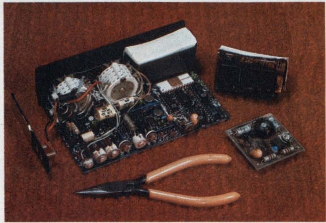
A flexible assembly for the indicator circuit and rigid boards for the rest allows Data Precision's Model 245 DMM to pack many parts in a small space.
