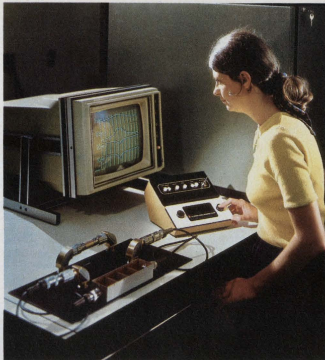
General Radio's 2200-line emphasizes binary computer/system communication and instrument-on-a-board circuitry. The 2260 automatic network analyzer shown can characterize circuit performance in the 200-kHz-to-500-MHz region with 0.1-Hz resolution. A simple user-oriented language controls the system.
