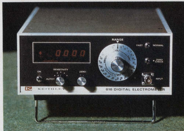
The Keithley 616 electrometer is one of the new breed of specialized digital measuring instruments. It can measure currents down to 20 pA.
