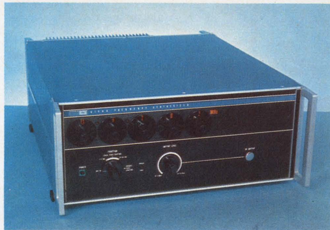
Indirect synthesis to 160 MHz, 100-Hz resolution and 0.5-ms switching of frequencies, typify the Fluke 6160A synthesizer.
