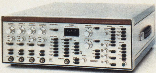
A 4-channel transient recorder from Biomation features 10-bit a/d conversion at rates up to 100 kHz. Data are stored in four 1024 word memories.
