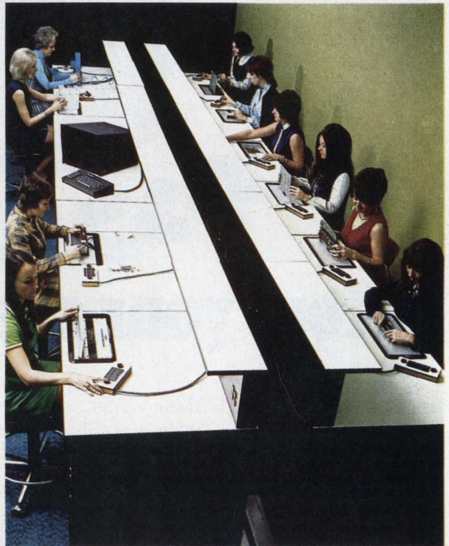
Ten independent, simultaneous test program can be run on this General Radio 2200 modular test system. Active or passive devices or logic circuits can be tested.
