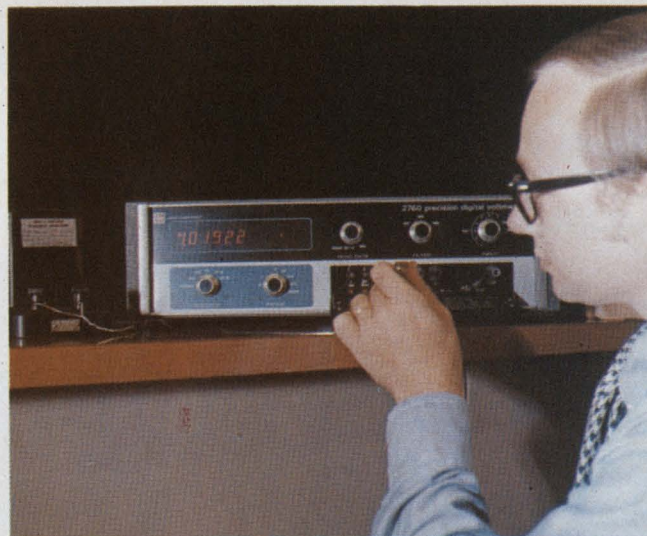
Precision digital voltmeter , by Leeds & Northrup, allows user to standardize the instrument at the work station. All that's needed are a screwdriver and five minutes.
