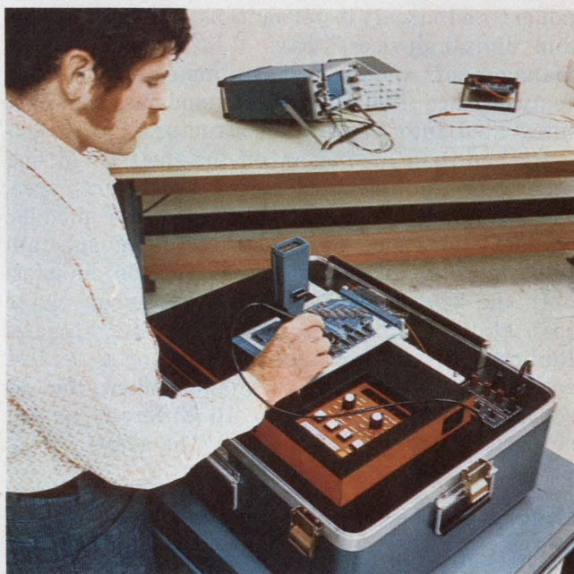
Node transition counts are compared to verify circuit operation in this Trender 1000 Logictester. To isolate a defect in an IC a special test fixture is used.
