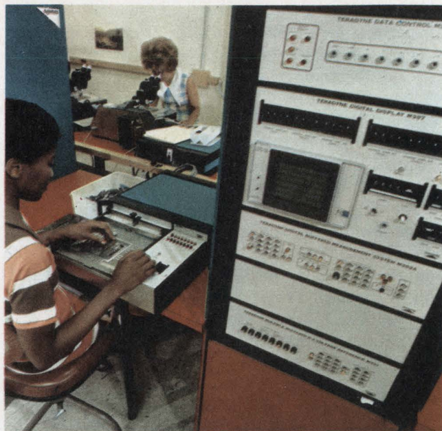
Final tests on character generators and dynamic shift registers are being made with Teradyne's J235 system. Digital ICs, hybrids and PC boards can also be tested.
