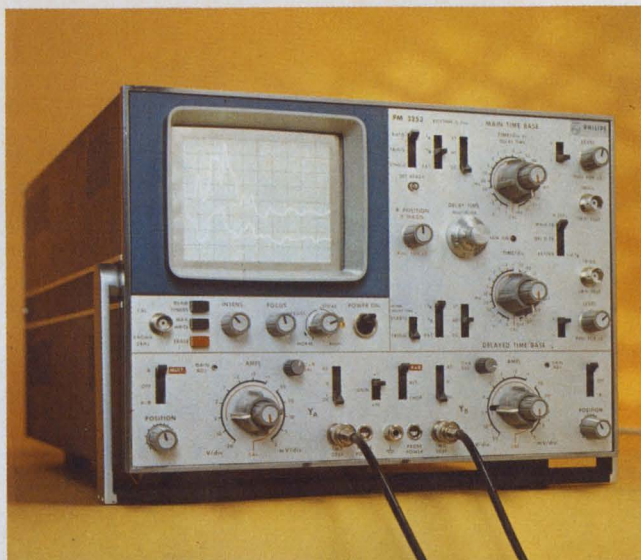
The Philips PM3253 scope multiplies two waveforms and displays the result. It has a 60-MHz bandwidth and sells for $3495. With it, the engineer can look at collector dissipation of a power transistor by applying both collector voltage and current simultaneously.
