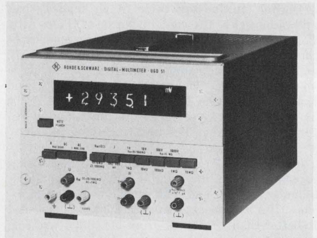
This DMM, Model UGD 51, from Rohde & Schwarz measures ac/dc volts and ohms. It delivers very high accuracy readings with its maximum count of \pm 30,000 .
