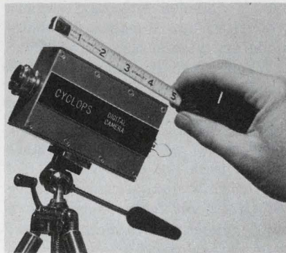
This solid-state camera kit uses a 32-by-32 array of MOS photodiodes to produce a low-resolution picture.
