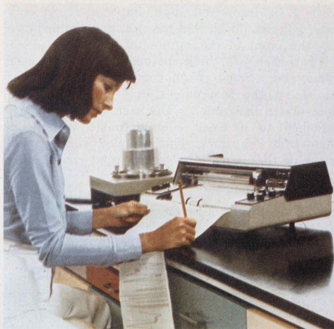
Flat-bed laboratory units, such as this one from Fisher Scientific, let the user write notes conveniently. The pen lifts electrically or manually, depending on model.
