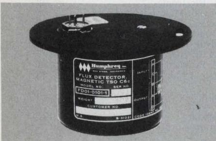
**LOW COST MAGNETIC FLUX DETECTOR** Model FD01 series provides continuous north reference when used with directional gyro or servo compass. TSO'd for autopilots and ideal for guidance and control systems for RPV's, drones, marine vehicles, buoys. Sensing element uses flux gate windings suspended in pendulous position. Freedom to  $\pm 45^\circ$  pitch and roll. Operates on 14 mA, frequency 400-Hz. 2.28" dia. x 1.91" high. Humphrey, Inc., 9212 Balboa Ave., San Diego, CA 92123. (714) 565-6631.
