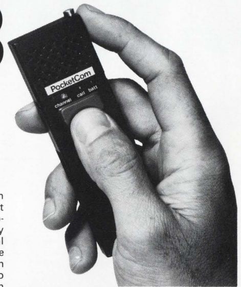
The PocketCom measures approximately 3/8" x 1 1/2" x 5/8" and easily fits into your shirt pocket. The unit can be used as a personal communications link for business or pleasure.
